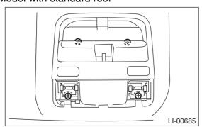
4) Disconnect the harness connectors and remove the spot map light.
