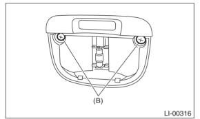
3) Disconnect the harness connector and remove the room light.
