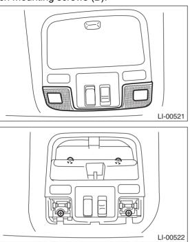
3) Disconnect the harness connector, and then remove the sunroof switch.
