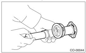
2) Increase pressure until the tester gauge pointer stops. Radiator cap is functioning properly if it holds the service limit pressure for five - six seconds.
