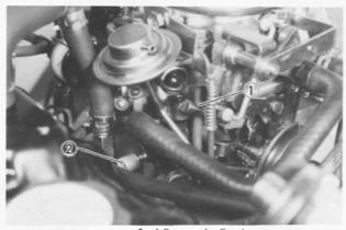
Idle speed adjusting screw
