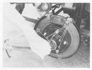
Fig. 17-5-28 Special Tool © (Hexagon Bit 6mm 09900-00414)
