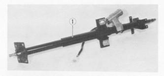
Fig. 18-10 ① Double tube type (Can't be disassembled)
