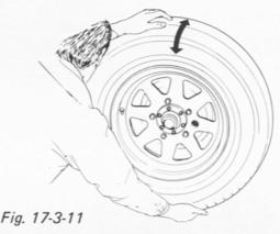
The above-mentioned method of making a shim adjustment demands a high degree of skill on the part of the serviceman. The alternative method is to adjust shim thickness by referring to the torque resistance which knuckle arm offers when pulled in the condition shown in figure. For this method, the reference torque value is established as indicated below, and you are to increase or decrease shim thickness to produce this torque value.
