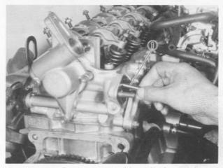
Fig. 3-6-54 Fuel pump rod installation
