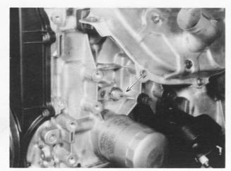
Fig. 3-8-8 Oil pressure switch
