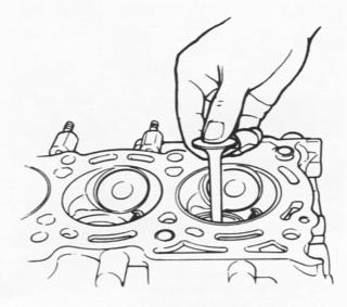
Fig. 3-6-30 Valve installation
