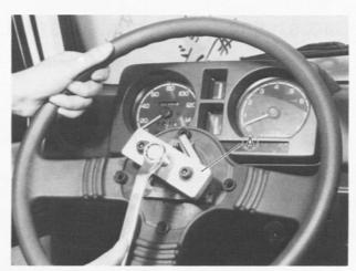
Fig. 18-4 (A) Special tool (Steering wheel remover 09944-38210)
