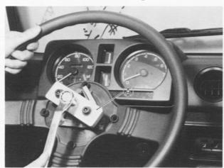
Fig. 7-6 (A) Special tool (Steering wheel remover 09944-38210)
