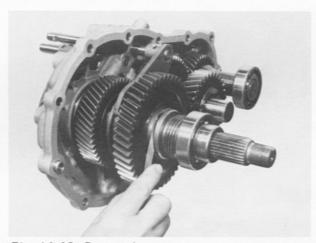
Fig. 14-40 Output low gear
