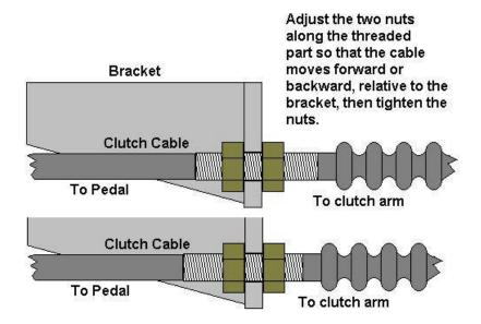
The distance that the clutch pedal travels before you feel any tension in the pedal is adjusted with the nuts on the engine bracket. The allowable pedal travel distance is .6 to 1 inch. Play with the two adjusting nuts on the bracket until the pedal travel is correct.
