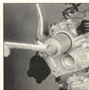
9.7a You can press a new seal into place with a section of pipe and a bolt of the proper size and thread pitch (don't let the camshaft turn as the bolt is tightened)
