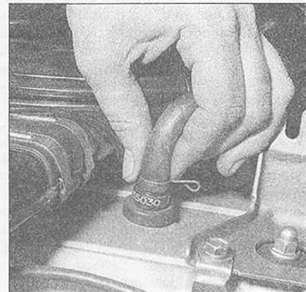
31.2 The PCV valve is located in the rocker arm cover
