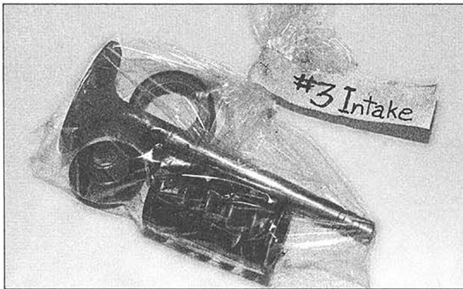
8.2a A small plastic bag, with an appropriate label, can be used to store the valve train components so they can be kept together and reinstalled in the correct guide
