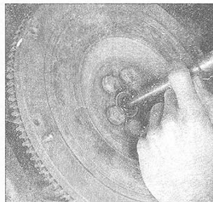
5.10 ... then force the bearing out hydraulically with a steel rod slightly smaller than the bore in the bearing - when the hammer strikes the rod, the grease will transmit force to the backside of the bearing and push it out
