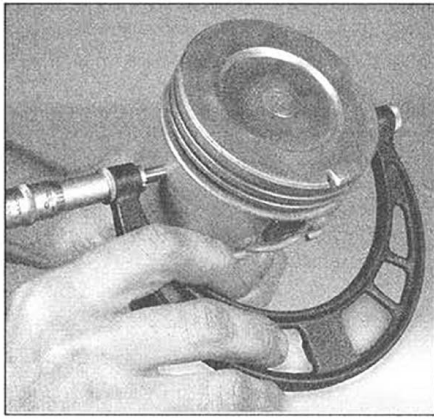
18.11 Measure the piston diameter at a 90-degree angle to the piston pin - the pistons must be measured at a precise point:
