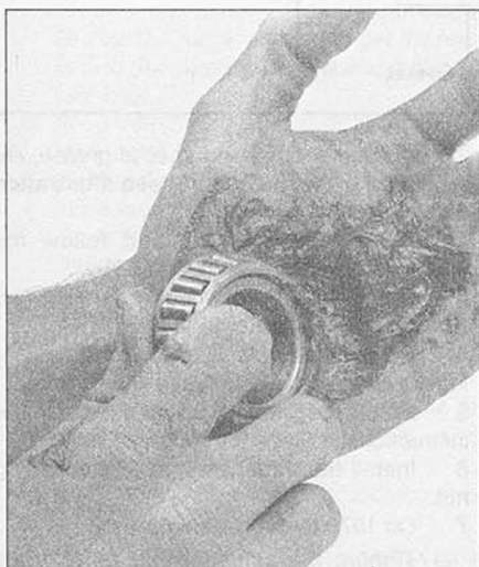
23.15 Work clean grease of the recommended type into each bearing until it's full
