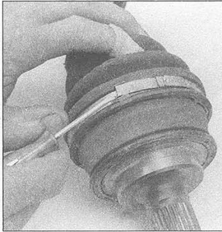
25.3 The large boot clamps can be pried open with a small screwdriver
