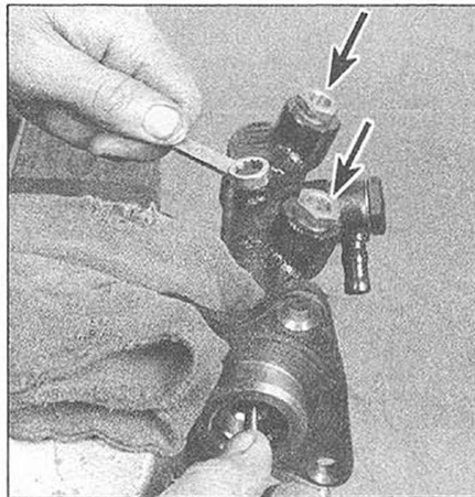
7.9 Push the pistons in all the way and remove the piston stop bolt and the copper gasket (also remove the two outlet plugs [arrows] and gaskets)
