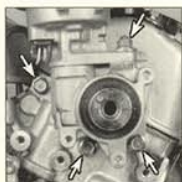
9.5a To remove the distributor drive adapter, remove the distributor hold-down nut (upper arrow), remove the distributor and remove the three adapter retaining bolts (arrows)
