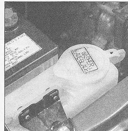
4.14 The windshield washer fluid level should be kept near the top of the reservoir - don't confuse the windshield washer and engine coolant reservoirs
