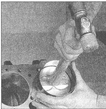
24.9 The piston can be driven (gently) into the cylinder bore with the end of a wooden hammer handle
