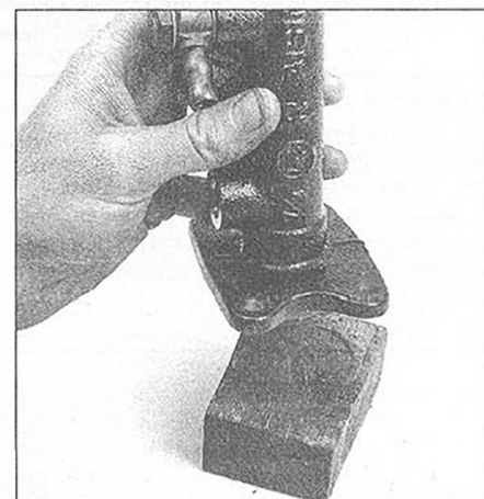
7.11b To free the No. 2 piston and spring, tap the cylinder firmly against a block of wood
