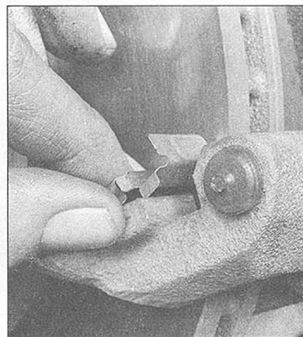
2.18 Install the pad support plates into the torque plate
