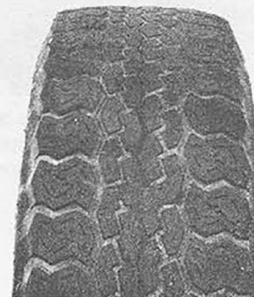
FEATHERING DUE TO MISALIGNMENT
