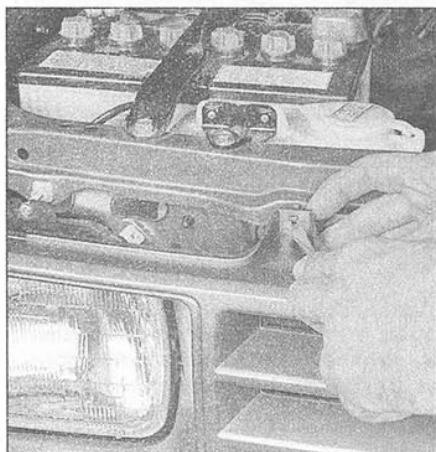
18.6 Disengage the grille by prying on the retaining clips while pulling out on the grille
