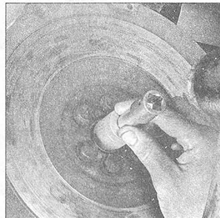
5.11 Using a hammer and socket, carefully drive the new bearing into place
