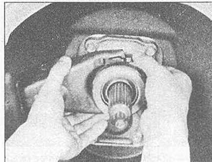
4.5 Removing the retaining clips from the clutch release bearing
