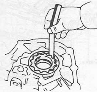
14.10c Measuring drive gear-to-driven gear clearance with a feeler gauge
