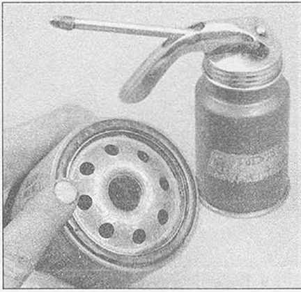
15.18 Lubricate the oil filter gasket with clean engine oil before installing the filter on the engine
