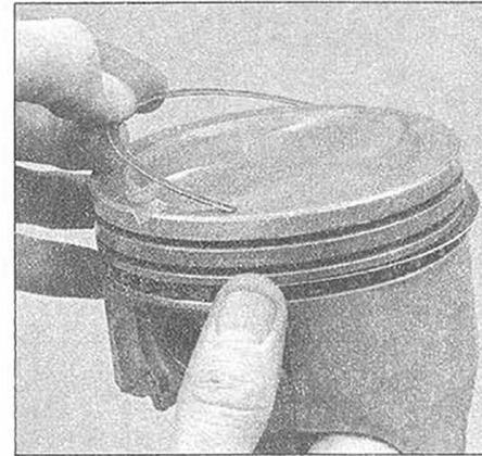
21.9b DO NOT use a piston ring installation tool when installing the oil ring side rails
