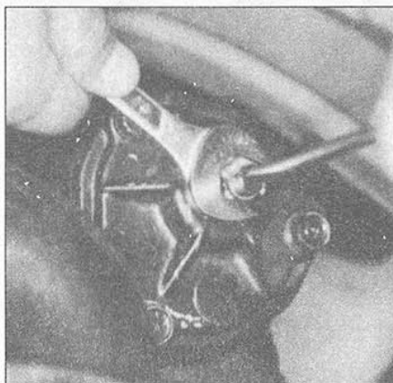
20.6 The adjusting screw must be held stationary while tightening the locknut
