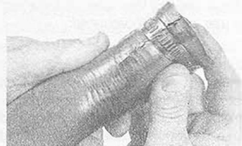
11.4 Hoses, like drivebelts, have a habit of failing at the worst possible time - to prevent the inconvenience of a blown radiator or heater hose, inspect them carefully as shown here
