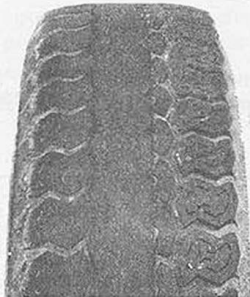
INCORRECT TOE-IN OR EXTREME CAMBER
