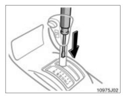
If you cannot shift automat transmission selector lever (four-wheel drive models)
