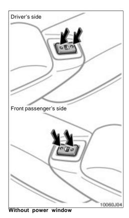
LOCKING AND UNLOCKING WITH POWER DOOR LOCK SWITCH Push the switch.
