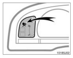
This SRS airbag system has a service reminder indicator to inform the driver of operating problems. If either of the following conditions occurs, this indicates a malfunction of the airbags. Contact your
