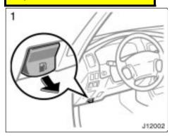
1. To open the fuel filler door, pull the lever.
