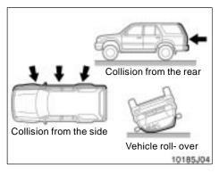
The SRS airbags are not designed to inflate if the vehicle is subjected to a side or rear impact, if it rolls over, or if it is involved in a lowspeed frontal collision.
