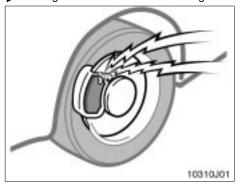
Even if the anti-lock brake system should fail, the brake system will still operate conventionally. However, when the "ABS" warning light is on (and the brake system warning light is off), the anti-lock brake system is not assisting brake performance so that the wheels can lock-up during sudden braking or braking on slippery road surfaces. Have your vehicle checked by your Toyota dealer as soon as possible.
