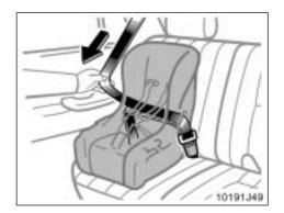
2. Fully extend the shoulder belt to put it in the lock mode. When the belt is then retracted slightly, it cannot be extended.
