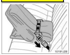
1. Run the center lap belt through or around the infant seat following the instructions provided by manufacturer and insert the tab into the buckle taking care not to twist the lap belt.
