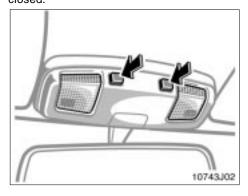
To turn on the personal light, push the switch. To turn the lights off, push the switch once again. Luggage compartment light
