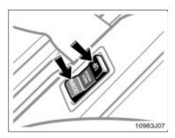
The back window can be operated with the inner switch on the center console or outer switch on the back door.
