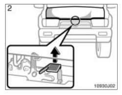
2. In front of the vehicle, pull up on the Jauxilialy catch lever and lift the hood.
