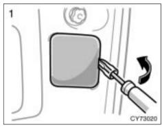
Use a flat-bladed screwdriver which is wrapped with a cloth.
