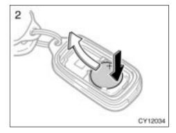
2. Remove the discharged transmitter batterv.
