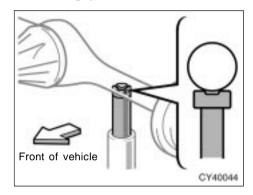
After making sure that no one is in the vehicle, as the jack touches the vehicle and begins to fit, double check that it is properly positioned.
