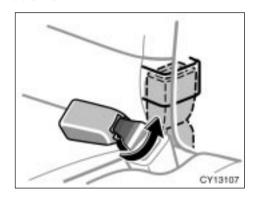
The rear center seat belt buckle can be stowed when not in use.
