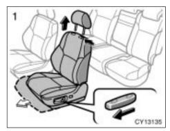
Remove the head restraint. Push the seat position adjusting switch forward to slide the seat further forward than the front-most position.
