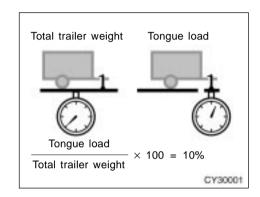
The trailer cargo load should be distributed so that the tongue load is 10% of the total trailer weight, not exceeding the maximum load of the following.
