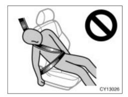
Do not get your head closer to the area where the side airbag and curtain shield airbag inflate, since these airbags inflate with considerable speed and force. Otherwise, you may be killed or seriously injured. Special care should be taken especially when you have a small child in the vehicle.
