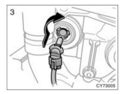
Install a new bulb and connector into the mounting hole and turn them clockwise to the front of the vehicle.
