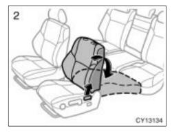
Pull the seatback angle adjusting lever to unlock and push down the seatback.
