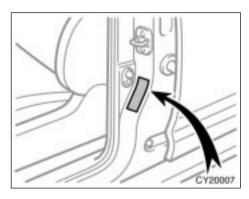
The vehicle identification number (VIN) is also on the Certification Label.
