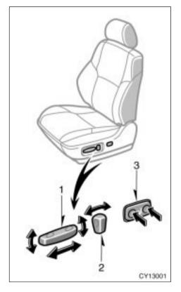
1. DRIVER'S SEAT: SEAT POSITION, SEAT CUSHION ANGLE AND SEAT HEIGHT ADJUSTING SWITCH
