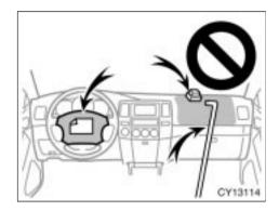
Do not put objects or your pets on or in front of the dashboard or steering wheel pad that houses the front airbag system. They might restrict inflation or cause death or serious injury as they are projected rearward by the force of the deploying airbags. Likewise, the driver and front passenger should not hold objects in their arms or on their knees.
