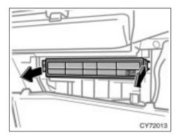
3. Remove the filter case by holding both sides.
