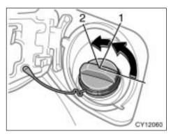
To remove the fuel tank cap, turn the cap counterclockwise by 90 degrees (to the pressure point 1), and then turn it an additional 30 degrees (to point 2). Pause slightly before removing it.
