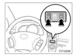
The back window can be operated with the switch on the instrument panel or the key operation in the back door keyhole.
