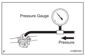
(e) Check the vacuum when the engine idles.
