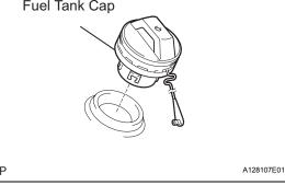
(5) Check if the pressure decreases when the fuel tank cap is removed while applying pressure. HINT:
