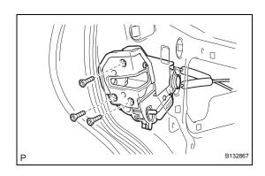
(b) Using a torx socket wrench (T30), remove the 3 torx screws and rear door w/ motor lock assembly LH. HINT:
