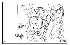
(b) Using a torx socket wrench (T30), remove the 3 torx screws and the front door lock assembly LH. HINT:
