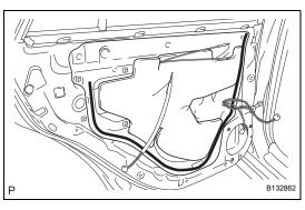
(b) Install the rear door service hole cover LH, as shown in the illustration.
