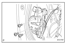
(c) Insert the control rod into the door lock, and then set it to the door panel.
