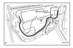
(b) Install the front door service hole cover LH, as shown in the illustration. HINT:
