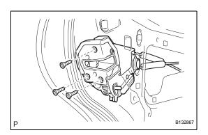
(d) Apply adhesive to the threads of the 3 torx screws. **Adhesive:**
