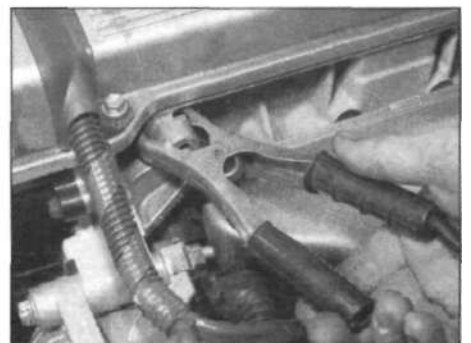
4 Connect the other end of the black jump lead to a bracket on the cylinder head, well away from the battery, on the vehicle to be started
