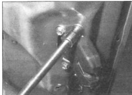
20.3 ... then unbolt the tailgate lock
