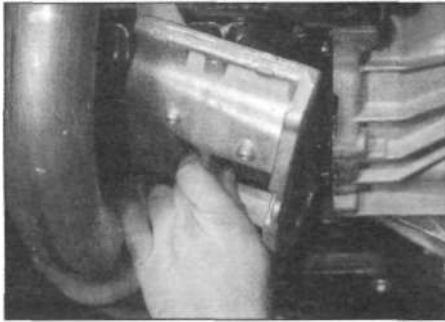
6.14 Removing the engine-to-transmission reinforcing plate
