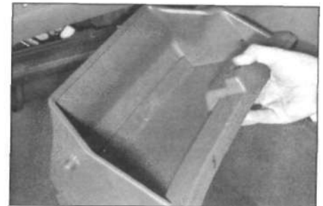
29.24 Removing the glovebox from the fascia panel
