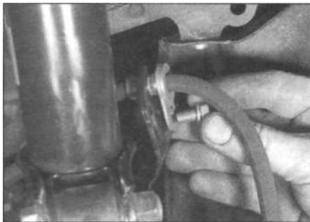
4.2 Removing the flexible brake hose bracket from the suspension strut
