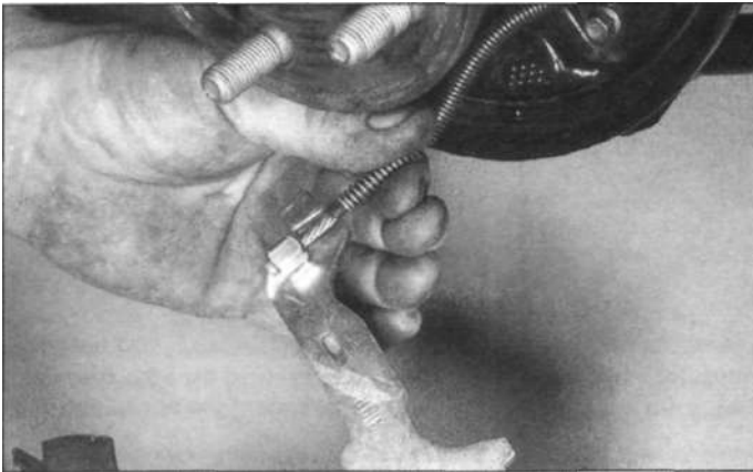
8.33 Disconnect the handbrake cable from the lever on the trailing brake shoe
