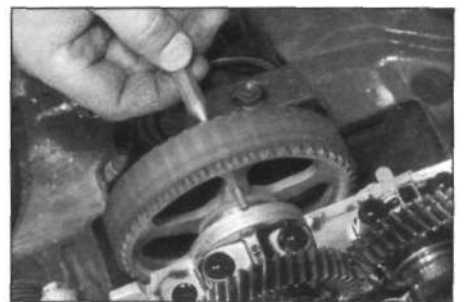
3.6 Check the camshaft is at TDC by inserting a dowel rod through the hole into the bearing cap cut-out
