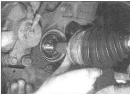
2.11 Removing the driveshaft outer CV joint from the hub carrier
