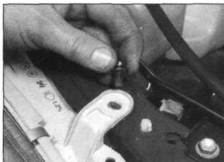
7.6a ... and upper mounting bolt.
