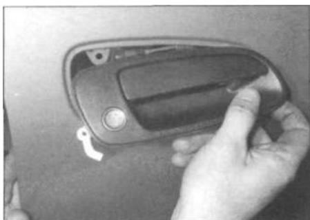
13.19 Removing the front door exterior handle and lock cylinder
