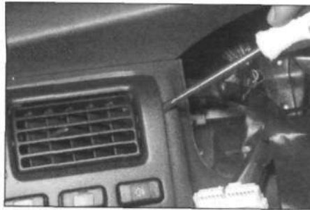
29.10a Use a screwdriver to prise out the centre surround ...
