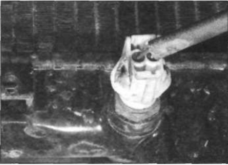
3.5 Cooling fan temperature switch on the radiator bottom tank (3S-FE and 3S-GE engines)
