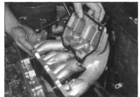
9.24a Removing the inlet manifold and gasket...
