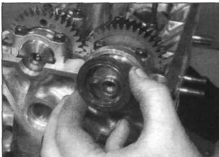
7.4a Ease the new oil seal over the end of the camshaft...
