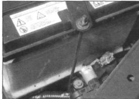
3.4 Battery retaining clamp and rod
