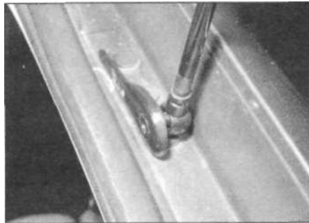
19.12 Tailgate support strut mounting on the rear body panel
