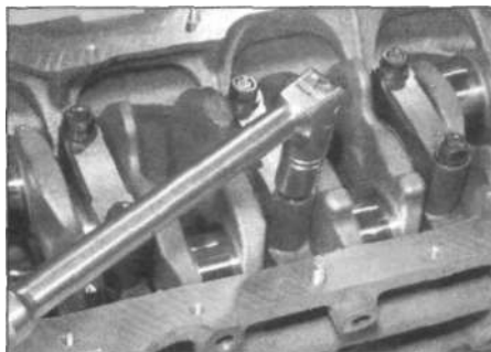
10.4b Loosening the main bearing cap bolts
