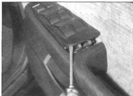
12.15a Prise the power window switch panel from the armrest...
