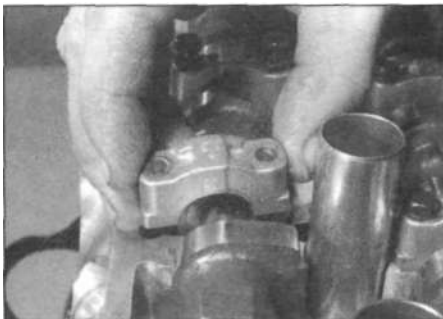
8.42a Refitting the inlet camshaft bearing caps
