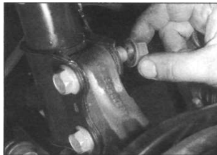
4.3 Remove the nuts and the bolts, and release the suspension strut from the hub carrier
