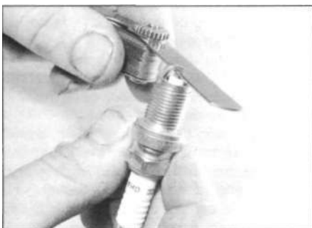
31.9a Measuring the spark plug gap with a feeler blade
