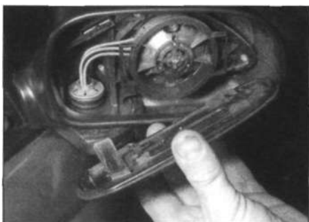
21.7 Removing the mirror glass
