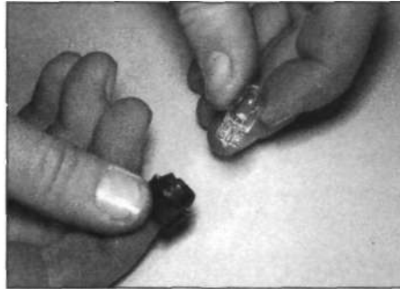
6.10 ... and pull out the wedge-type bulb
