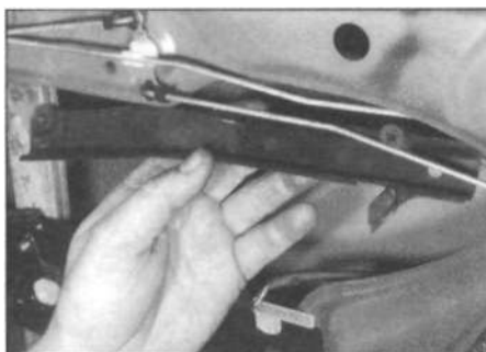
13.12b ... and remove the security bracket
