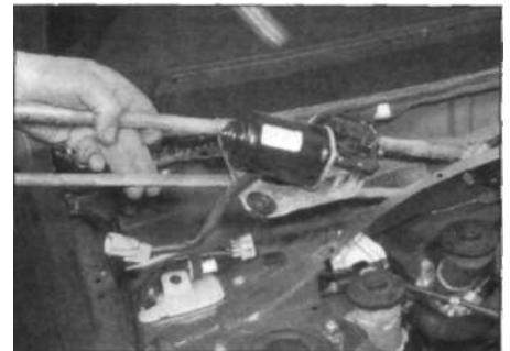
15.6b ... and remove the windscreen wiper motor and linkage
