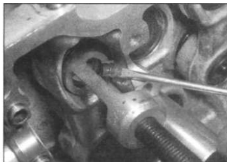
8.4 Using a dab of grease to retain the collets on the valve stems
