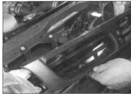
7.2 ... and withdraw the radiator grille
