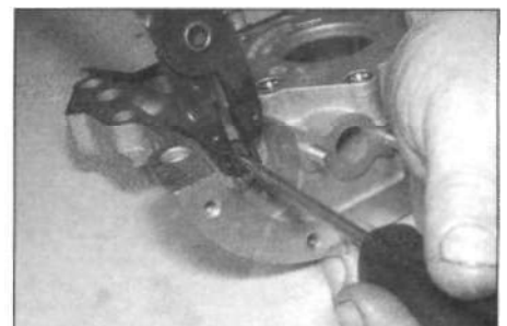
11.14 When refitting the circlip to the oil pump housing, depress the spring cap with a screwdriver
