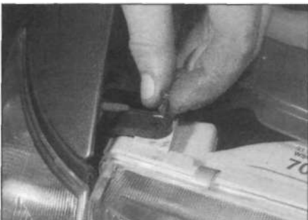
5.18 Removing the front direction indicator retaining screw
