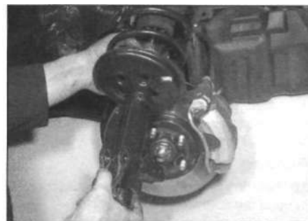
4.4c ... then withdraw the strut from under the wheel arch
