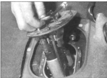
8.10 ... and withdraw the fuel pump/fuel gauge sender unit assembly from the top of the fuel tank
