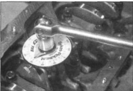
18.22 Using an angle-tightening gauge to tighten the big-end bearing cap bolts to their Stage 2 angle
