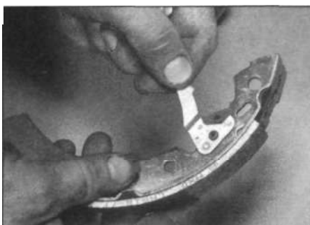
8.37a Place the adjuster lever on the peg of the new leading brake shoe ...
