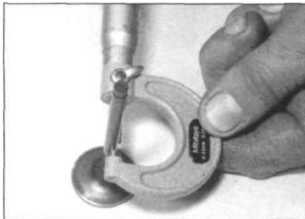
7.11 Measuring the valve stem diameter
