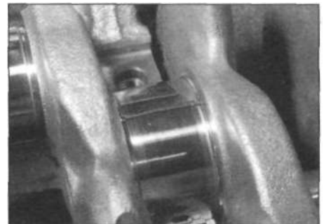
16.5 Cut several lengths of Plastigauge and place one on each crankshaft journal
