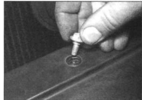
6.8 Front bumper upper mounting bolt removal
