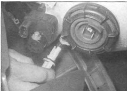
5.13 Removing the front sidelight bulbholder from the headlight
