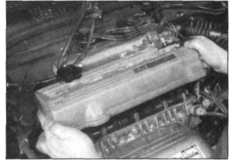
4.13c ... and remove the camshaft cover (3S-FE engines)
