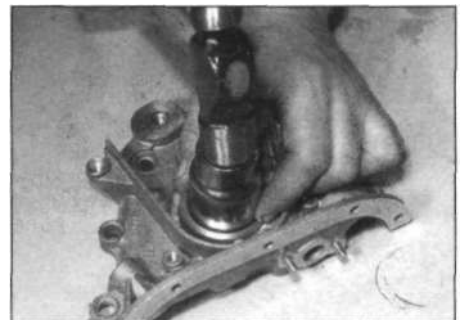
13.1b Using a hammer and socket to drive in the new oil seal
