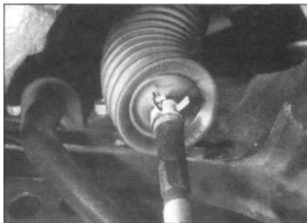
21.3 Steering gear rubber gaiter outboard retaining clip
