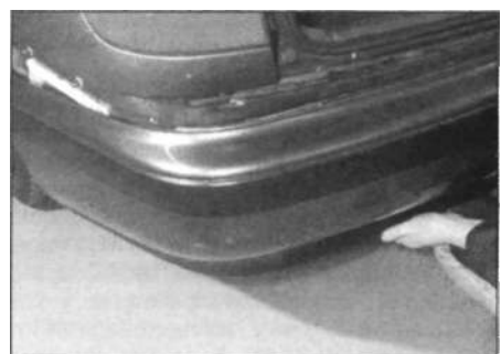
6.18 Withdrawing the rear bumper from the body
