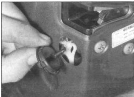
13.11 Prise out the child safety lock control
