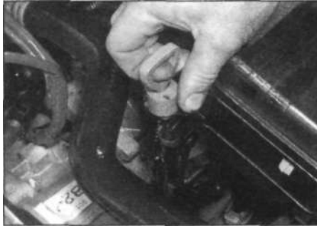
5.4 Withdraw the automatic transmission fluid dipstick from its tube
