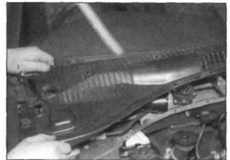
15.4c ... and remove the cowl panels
