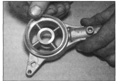
12.5b The O-ring is located in the housing groove
