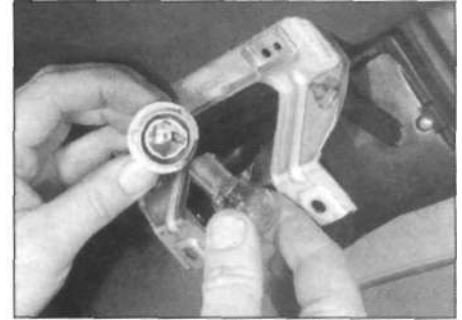
5.51b ... and remove the bulb
