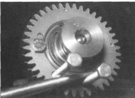
8.12a Use two bolts to hold the inlet camshaft sub-gear tensioned while the retaining bolts is removed
