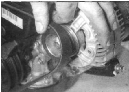
5.2 Disconnecting the auxiliary drivebelt from the alternator
