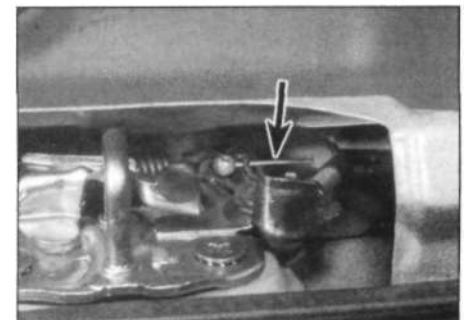
20.11b Control cable on the tailgate lock striker
