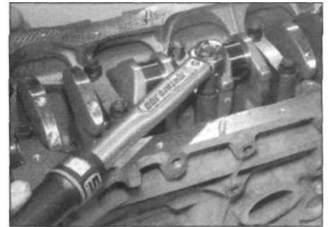
16.19c ... then progressively tighten them to the specified torque
