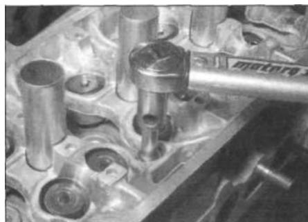
9.50c Tightening the cylinder head bolts to the Stage 1 torque setting
