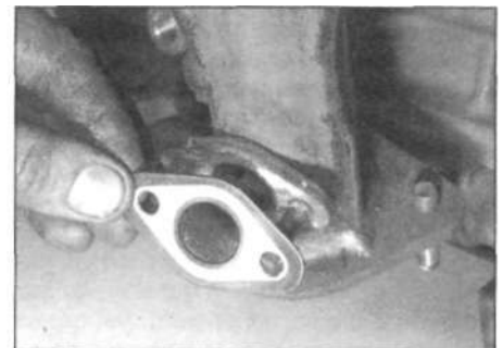
2.7c ... and gasket (lean-burn engines)
