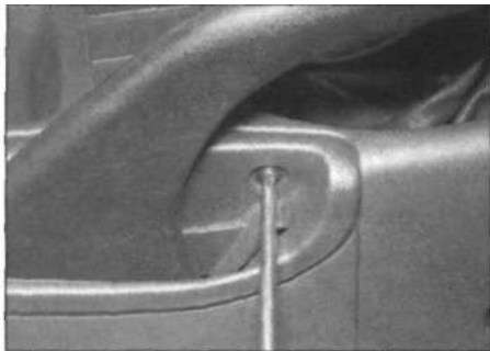
28.3a Remove the screw ..
