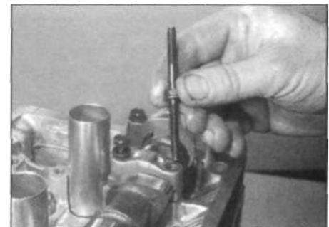
8.10c Remove the bolts ...
