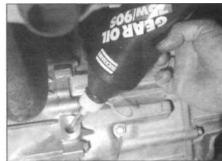
4.3 Topping-up the manual transmission oil level
