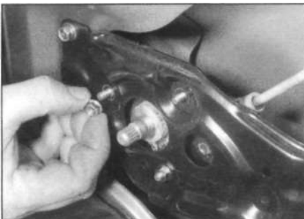
14.16 Removing the rear door window regulator mounting nuts
