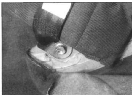
26.7a Rear seat belt lower mounting bolt
