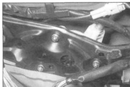
14.5b Front door window regulator mounting bolts (models with power windows)
