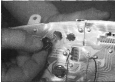
6.9 Remove the bulbholder from the instrument panel...
