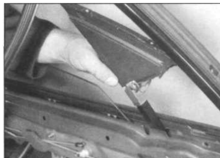
14.21 ... and remove the rear channel/plate from the door
