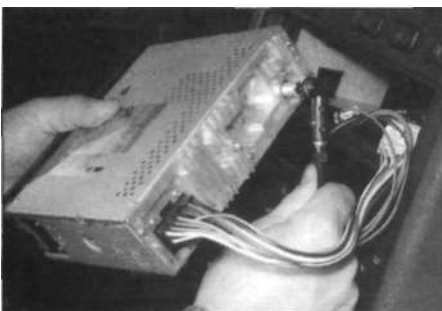
18.5 Disconnecting the aerial from the rear of the radio
