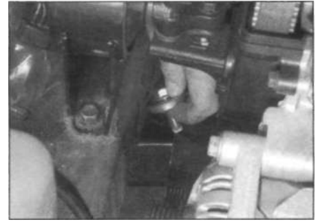
5.11a Removing the crankshaft pulley bolt
