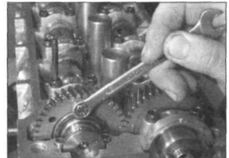
8.43 Unscrewing the bolts securing the sub-gear to the main gear on the inlet camshaft
