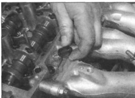
9.23c ... then remove the long spacers...
