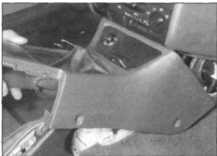
28.4b . withdraw the console ..
