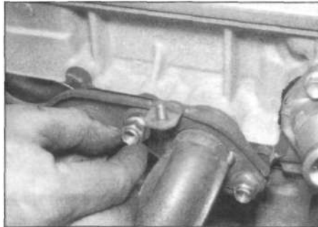
15.5b ... then remove the nuts .
