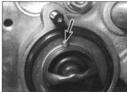
4.11a The thermostat jiggle pin must face upwards
