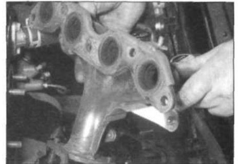
15.5c ... and withdraw the exhaust manifold from the cylinder head studs
