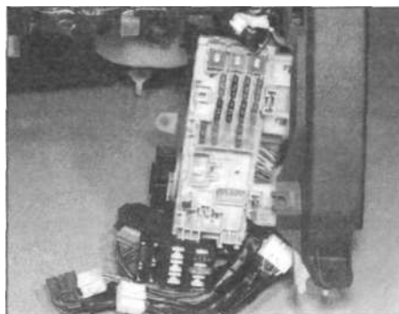
3.10 Facia-mounted fusebox (shown with the facia removed from the vehicle)
