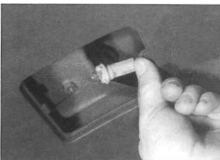
5.45a Remove the rear number plate light bulbholder...
