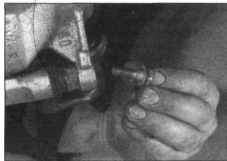
4.3a Remove the brake caliper lower guide pin bolt...
