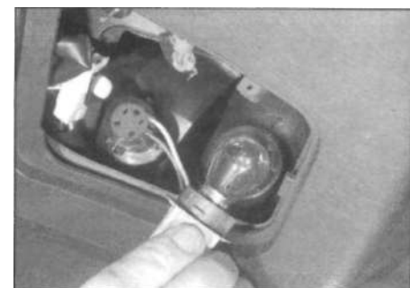
5.39a Remove the rear fog/reversing light bulbholder. ...
