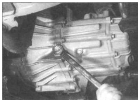
4.2 Unscrewing the filler/level plug from the front face of the transmission
