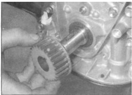
6.4 Removing the crankshaft sprocket
