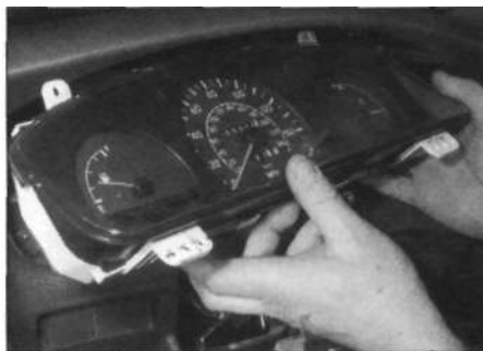
8.4 Removing the instrument panel from the fascia
