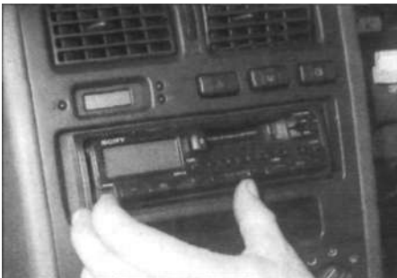
18.2 Removing the security front from the radio
