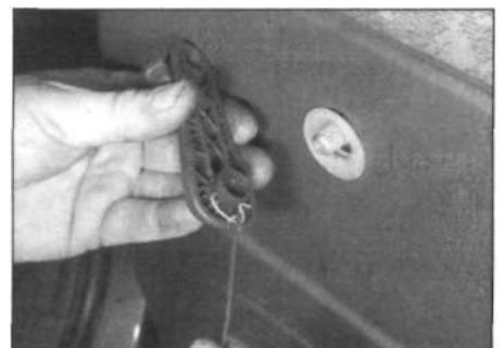
12.5a Using a length of welding rod to release the window regulator handle retaining spring
