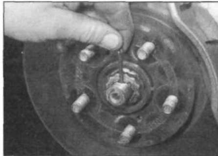
2.22b ... then fit a new split pin and bend over the legs to secure
