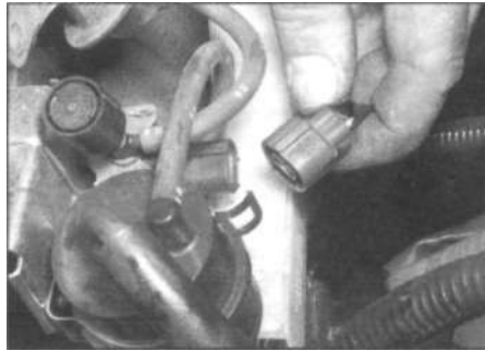
13.106 Disconnecting the wiring from the air control valve vacuum switching valve (4A-FE lean-burn engines)
