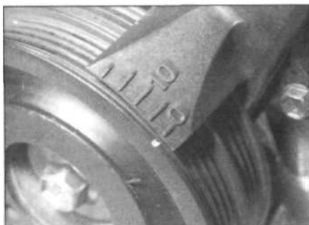
6.2 Ignition timing marks on the crankshaft pulley and timing belt cover (4A-FE and 7A-FE engines)
