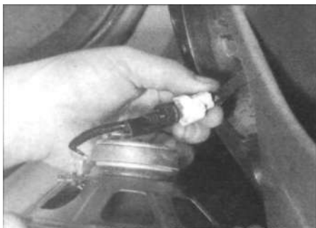
12.17c ... and disconnect the wiring
