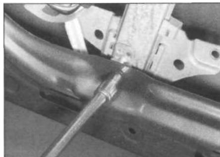
14.5c Front window regulator lower mounting bolt
