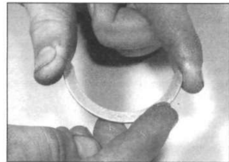
16.15 Use a dab of grease to hold the thrustwashers in position each side of the centre main bearing
