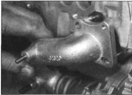
7.14a Removing the water pump rear elbow...
