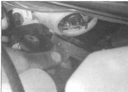
5.6 ... remove the dust cover ...
