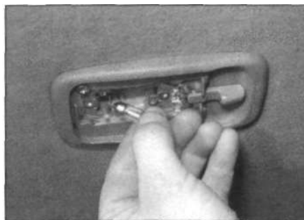
6.6a Removing the festoon-type bulb from the interior light...
