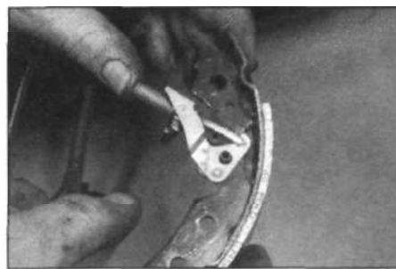
8.37b ... then refit the adjuster strut so that the forked end engages over the adjuster lever
