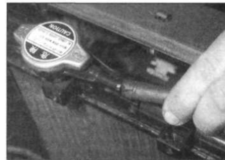
3.4 Disconnecting the expansion tank hose from the radiator
