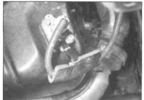
10.7 Oil temperature sensor on the sump
