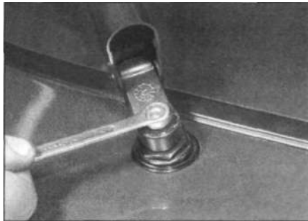
14.3c Unscrewing the tailgate wiper arm-to-spindle mounting nut
