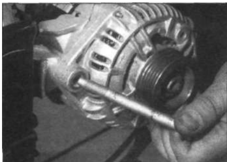
5.5a ... upper mounting bolt.
