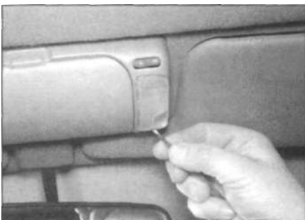
6.2 Prise out the roof front console light lens ...
