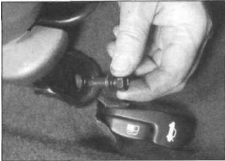
25.1 Front seat front mounting bolts removal
