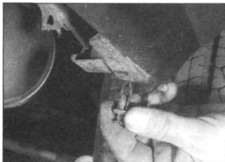
6.15 Removing the special clips from the front lower edge of the rear bumper
