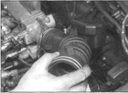
9.12 Removing the air duct from the throttle housing
