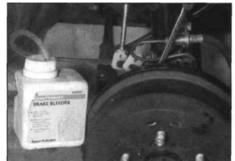
2.28 One-way valve brake bleeding kit connected to a rear wheel cylinder bleed screw
