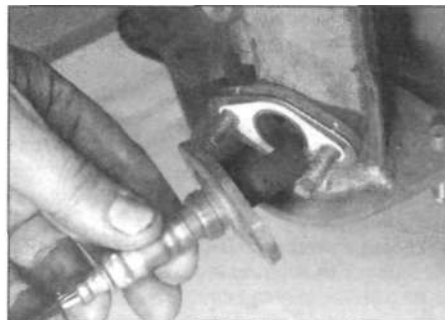
2.7b ... then remove the lean mixture sensor...
