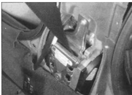
26.3 Front seat belt retractor unit at the base of the B pillar
