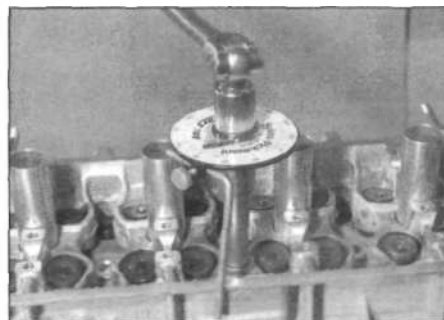
9.51 Angle-tightening the cylinder head bolts to the Stage 2 angle
