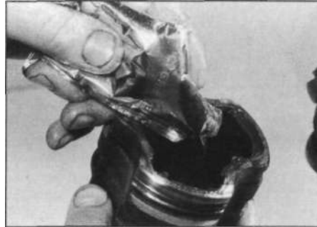
3.18 Pack the joint outer member with the grease supplied in the repair kit
