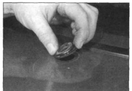
16.7 Removing the spindle grommet from the tailgate
