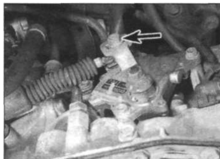
3.3 Gear selector cable-to-transmission selector lever retaining nut (arrowed)
