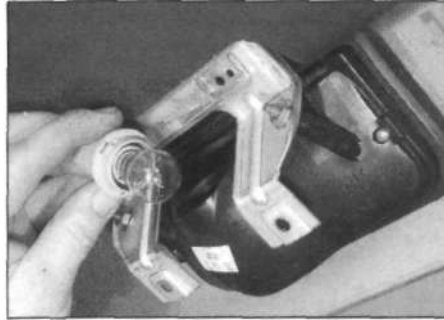
5.51a ... then twist the bulbholder from the body ...
