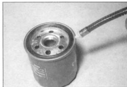
3.11a Apply a light coating of clean engine oil to the sealing ring on the new filter
