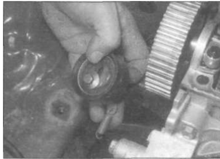
6.6 Removing the tensioner pulley
