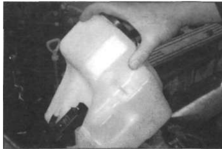
17.2 Removing the washer fluid reservoir
