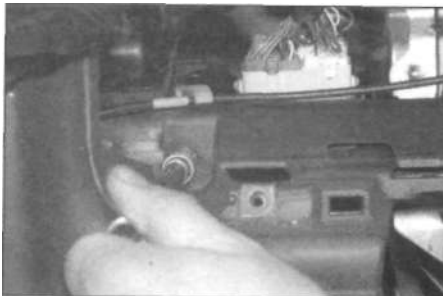
29.16 Removing the fascia mounting bolts on the bottom of the instrument panel aperture
