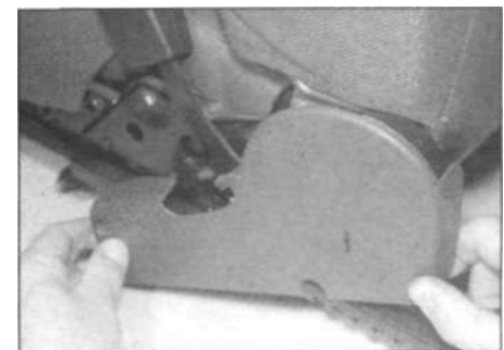
26.1a With the front seat removed, remove the plastic trim ...
