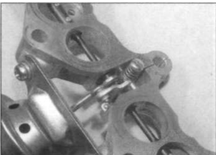
14.9 Vacuum adjustment screw on the air control valve assembly (do not adjust)
