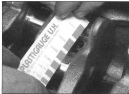
16.9 Using the Plastigauge scale to measure the main bearing running clearance
