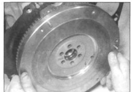
14.4d Removing the flywheel
