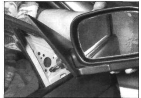
21.5b ... and remove the mirror assembly
