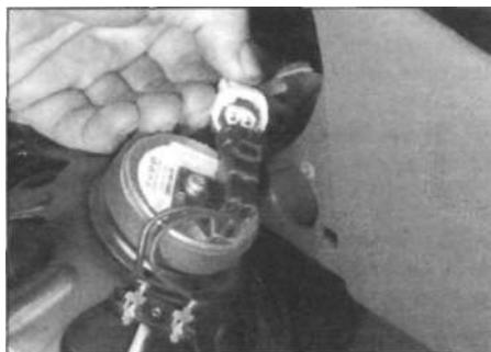
12.6c ... and disconnect speaker the wiring
