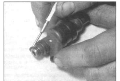
13.21b Removing the O-rings from the injectors
