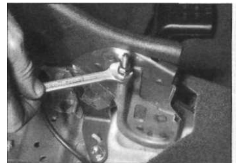
19.5 Adjusting the handbrake cable at the adjuster nut on the handbrake lever
