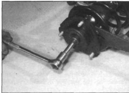
4.8 Unscrew the central piston rod nut while holding the upper spring seat
