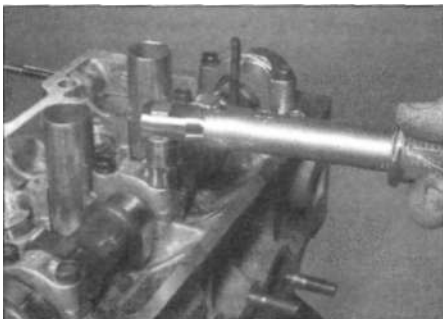
8.38d Tightening the exhaust camshaft bearing cap bolts to the specified torque
