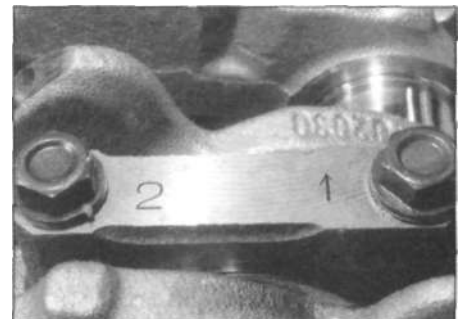
10.4c Main bearing caps are numbered and marked with an arrow towards the timing end of the engine
