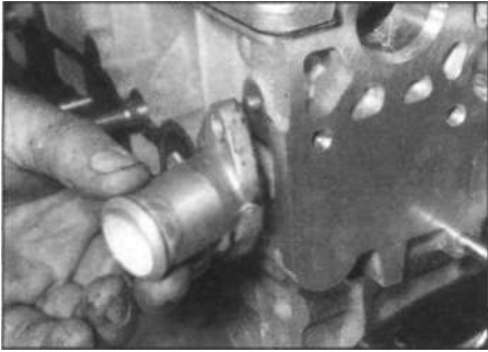
6.1a Removing the coolant outlet...
