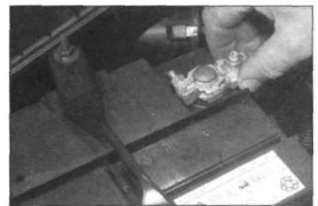
3.2 Disconnecting the battery negative terminal
