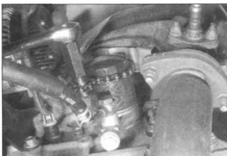
3.9 Using a chain strap to remove the oil filter (4A-FE engines)
