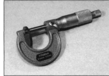
37.9 Measuring a shim with a micrometer
