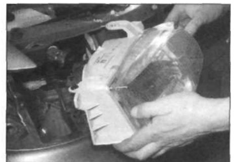
... and withdraw the headlight unit from the front of the vehicle
