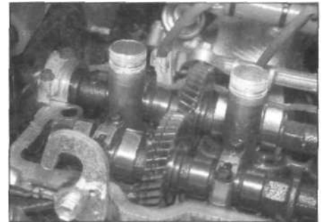
8.13 Inlet and exhaust camshafts showing the drive gears (3S-FE engine)
