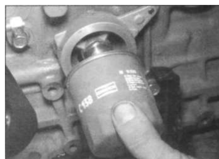
3.11b Screw on the new filter by hand
