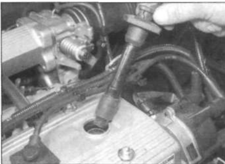
31.2 Disconnecting the HT leads from the spark plugs
