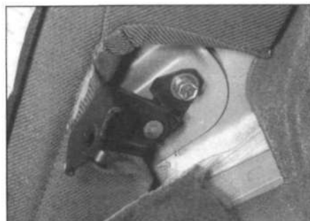
25.6b Fold-down rear seat side hinge and mounting bolt
