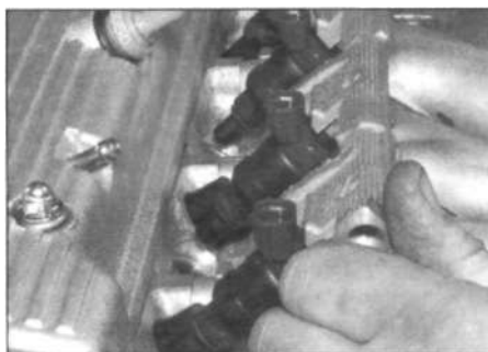
13.20 Removing the fuel rail
