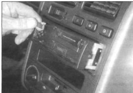
18.3a Insert a feeler blade through the slot in the radio to remove it
