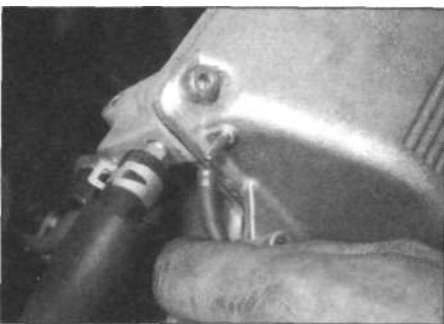
14.6a Disconnecting the pressure regulator vacuum sensing hose from the air inlet chamber cover
