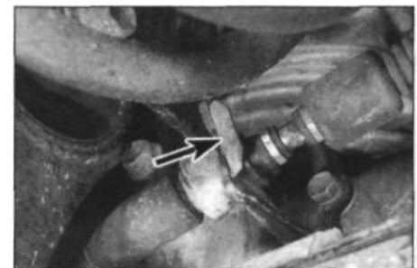
3.11 Extract the retaining clip (arrowed) to disconnect the selector outer cable from the bracket
