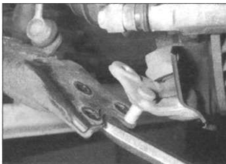
4.26b ... and lever the lower suspension arm downwards
