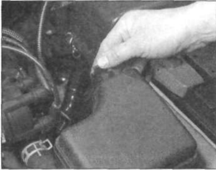
3.3a For access to the engine compartment fusebox, release the clips ...
