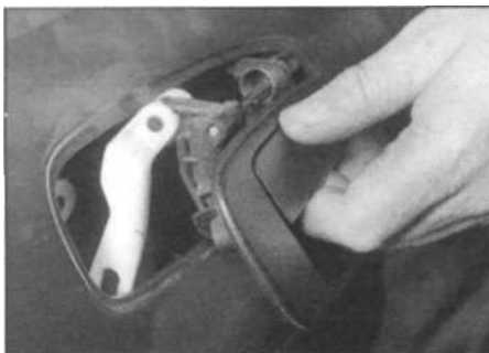
13.22 Removing the rear door exterior handle
