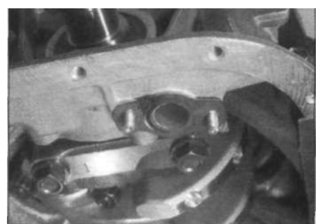
11.4b Oil pick-up tube/strainer assembly gasket on the oil pump housing
