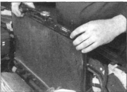
3.9 Lifting the radiator from the engine compartment
