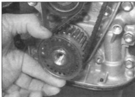
5.13 Slide the outer timing belt guide from the crankshaft key
