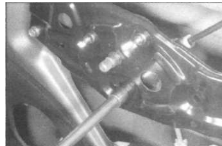
14.5a Front door window regulator mounting bolt removal (models with manual windows)
