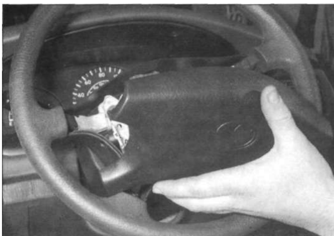
17.9 ... then lift off the module and disconnect the wiring connector
