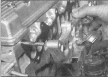
14.8a On lean-burn engines, remove the air control valve assembly ...
