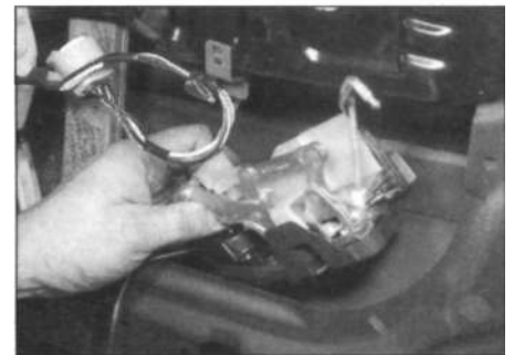
13.8b ... then withdraw the lock assembly from inside the door
