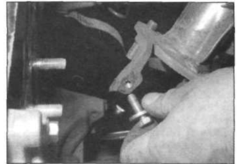
15.4 Removing the bolt from the exhaust manifold stay
