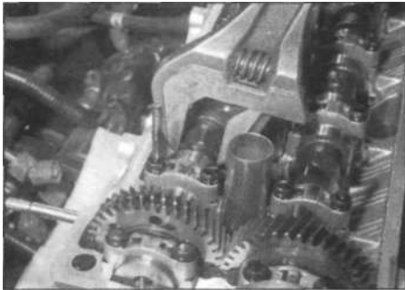
8.4 Using an adjustable spanner on the hexagonal section on the inlet camshaft
