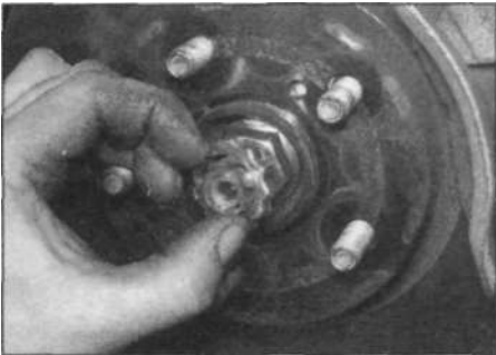
2.22a Refit the hub/driveshaft nut locking cap...
