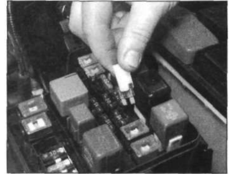
3.6 Using the plastic tweezers provided to remove a fuse
