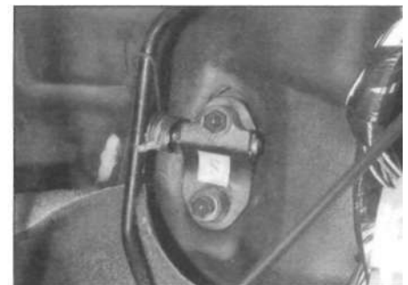
4.2 Accelerator pedal mounting on the bulkhead
