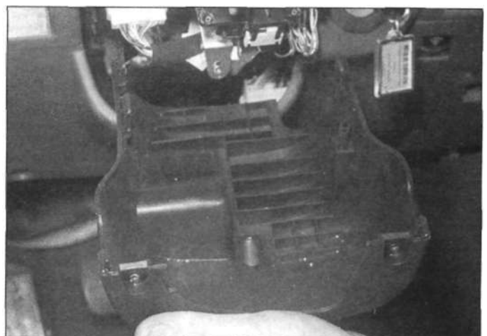
18.3 Undo the screw and lift off the lower steering column shroud
