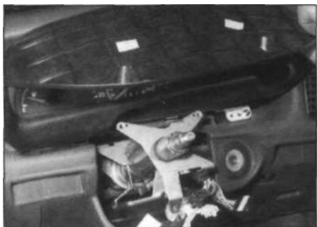
8.3b ... and remove the instrument panel surround
