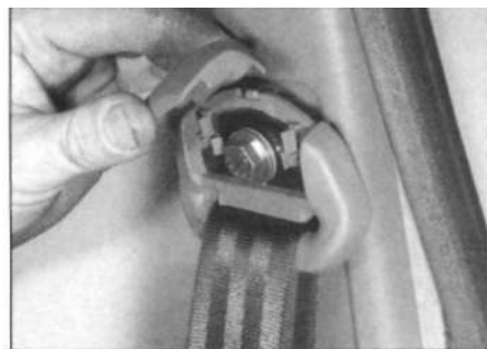
26.4 Prise the plastic cover from the front seat belt upper anchor bolt
