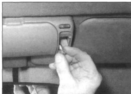
6.3 ... then depress and twist the bulb to remove it
