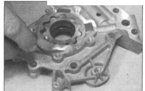
11.10a Using feeler blades to check the outer rotor-to-body clearance ...
