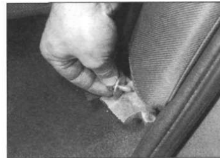
25.7 Removing the mounting bolt from a rear seat side cushion
