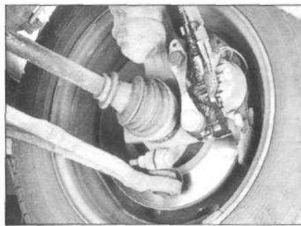
A leak occurring at a wheel is almost certainly brake fluid.
