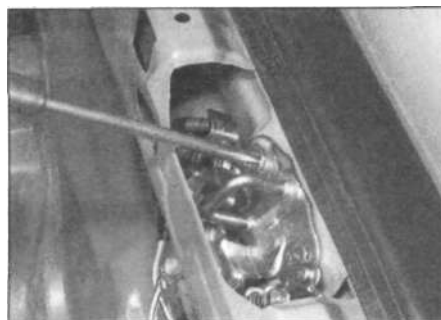
20.11a Tailgate lock striker removal
