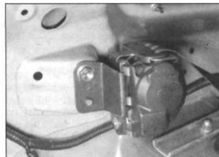
26.7b Rear seat belt retractor and mounting bolt
