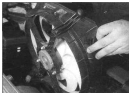
5.7 Removing the electric cooling fan assembly (4A-FE and 7A-FE engines)
