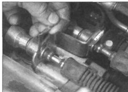
3.6 Extract the retainers securing the gearchange control outer cables to the bracket
