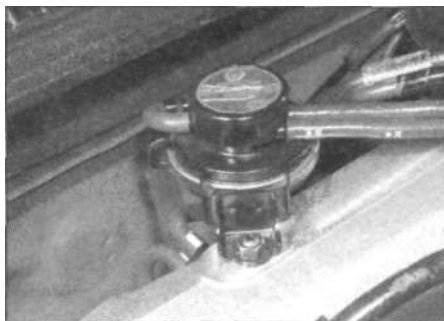
2.20 The EGR vacuum modulator (3S-FE engines)
