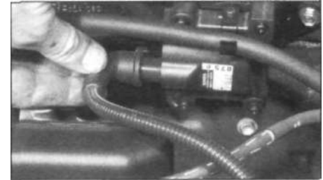
D Check that the HT lead is securely connected to the ignition coil, and spray with water-dispersant if necessary
