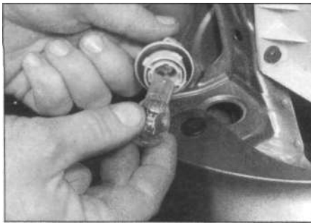
5.19b ... then depress and twist the bulb to remove it
