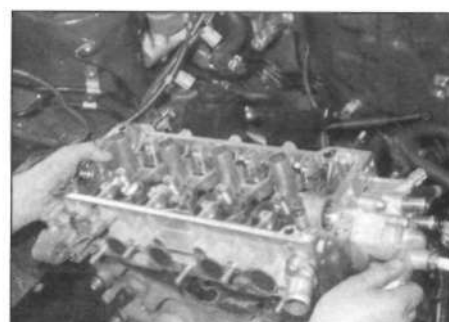
9.39a Lift the cylinder head from the block...
