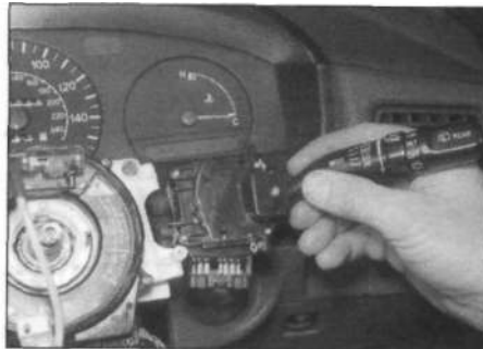
4.3b ... and remove the wiper switch
