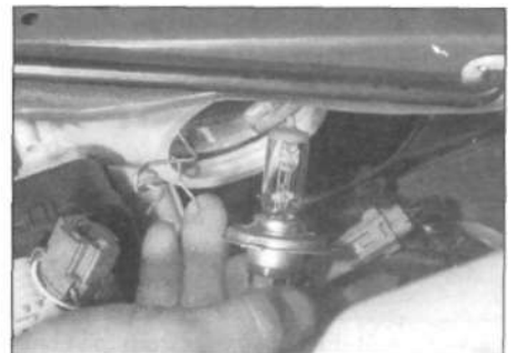
5.8 ... and remove the headlight bulb
