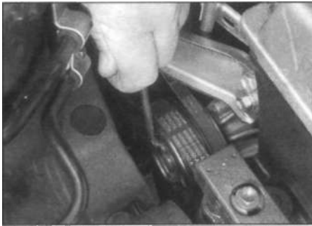
5.4 Loosening the water pump pulley bolts before removing the auxiliary drivebelts
