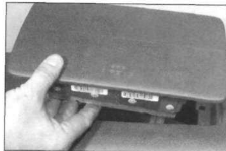
29.22 Passenger bag removal from the fascia panel
