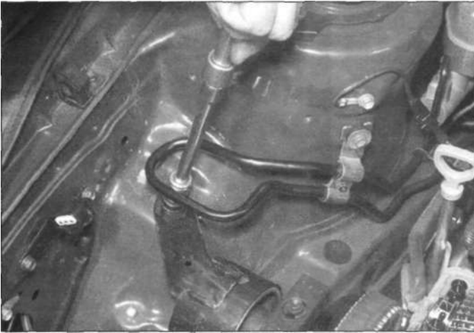
15.7a Unscrew the support bolt.
