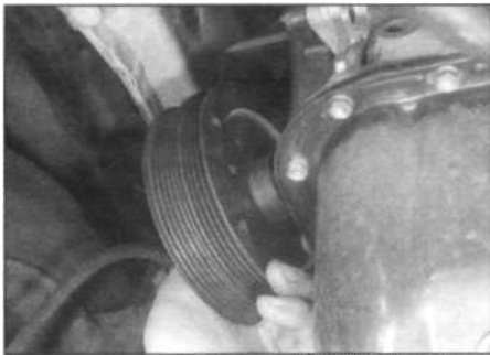
5.11b Sliding the pulley off the end of the crankshaft
