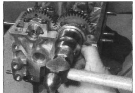
7.4b ... and drive it into position with a socket
