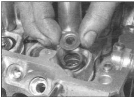
6.2b Remove the spring retainer ...
