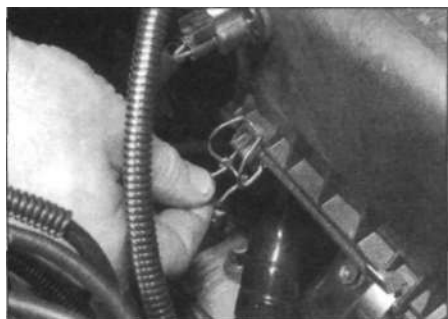
11.1a Release the toggle clips ...
