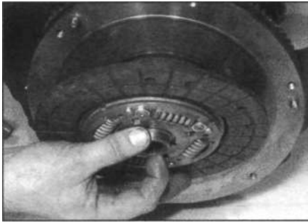
2.4 Removing the clutch disc
