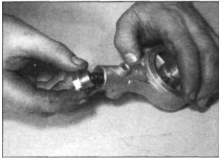
12.4a Remove the plug ...
