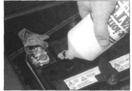
2.9c ... and topping up the electrolyte level
