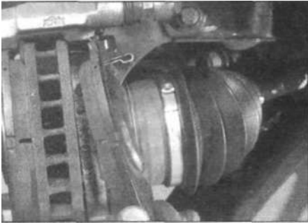
4.4b ... then withdraw the inner brake pad and shims ...
