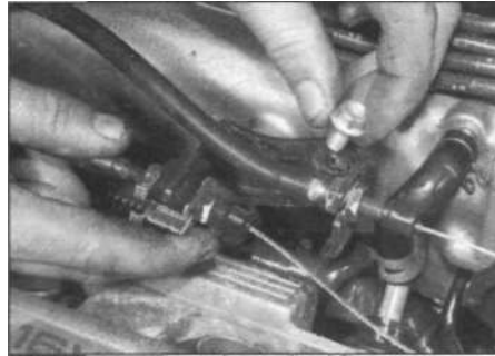
3.2b Unbolting the accelerator cable support (3S-FE engines)
