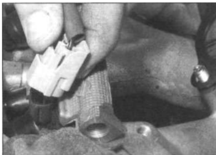
13.18 Disconnecting the wiring plugs from the injectors
