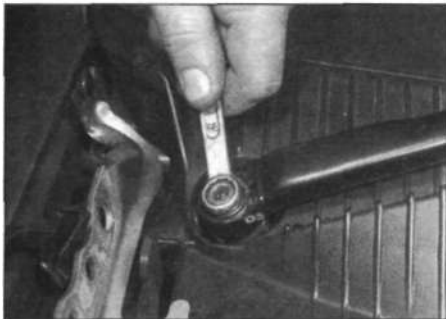
14.3b ... and unscrew the windscreen wiper arm-to-spindle mounting nut
