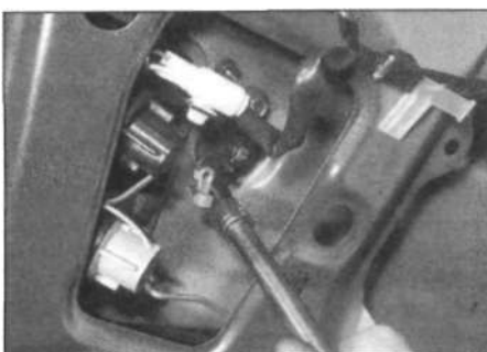
20.7 ... then unbolt the lock cylinder from the tailgate
