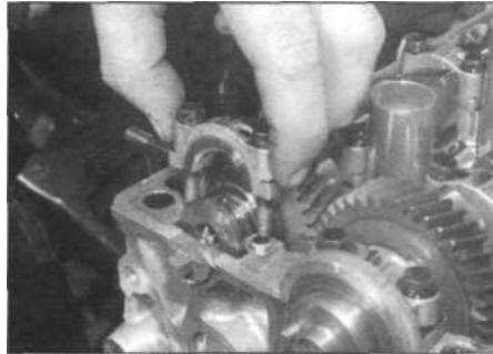
8.5 Removing the right-hand bearing cap from the inlet camshaft
