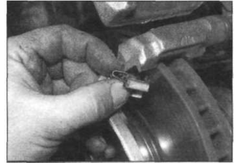
4.5 Remove the four brake pad support plates
