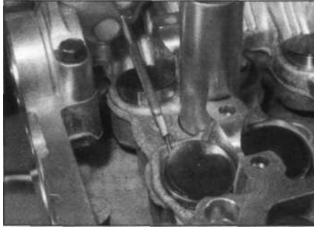
37.8 Using a small screwdriver to remove a shim from the top of the follower
