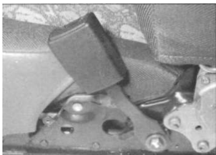
26.1b ... for access to the inner stalk and mounting bolt
