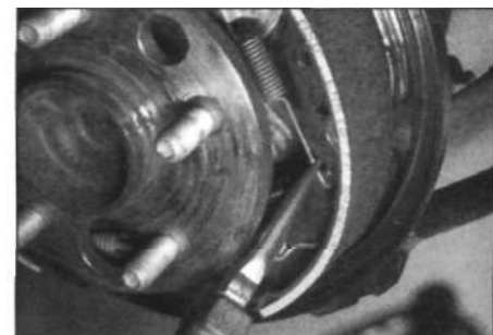
8.44 Attaching the adjuster lever spring to the brake shoe
