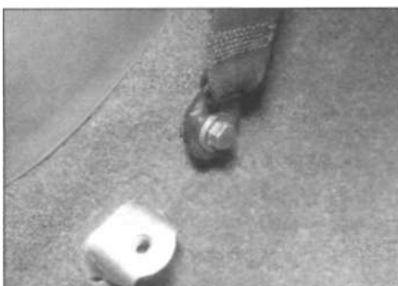
26.5 Front seat belt lower mounting bolt
