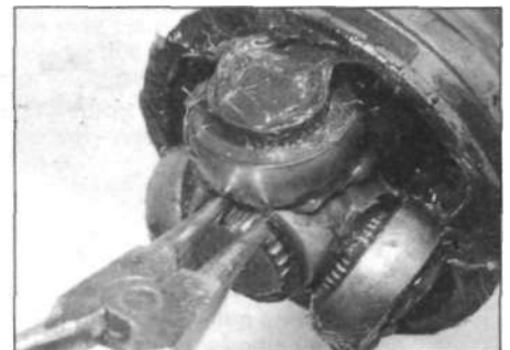
3.7 Removing the tripod retaining circlip
