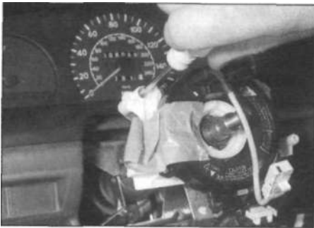
4.3d ... then unscrew the switch base mounting screw
