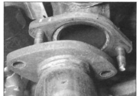
15.2 Separating the exhaust downpipe from the exhaust manifold
