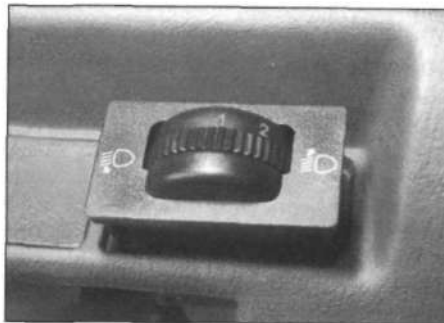
4.6a Prise the headlight leveller switch from the fascia ...
