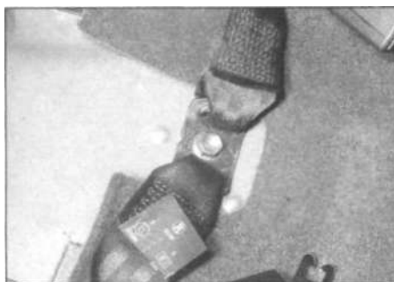
26.8 Rear seat centre lap belts and mounting bolt
