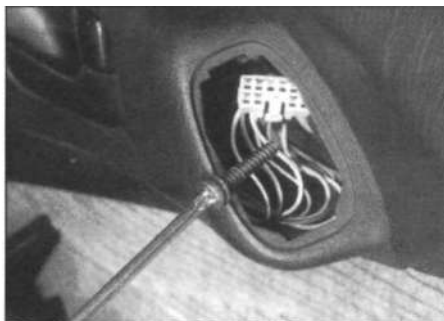
12.18 One of the trim panel mounting screws is located in the exterior mirror control panel aperture
