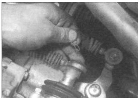
3.5 Removing the gearchange control cable retaining clip and washer at the transmission end
