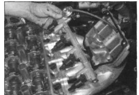
9.23b ... and remove the fuel rail...
