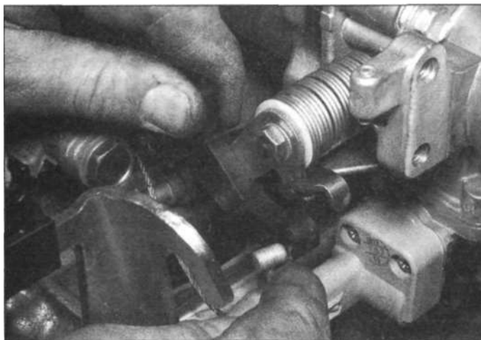
3.1a Disconnecting the accelerator cable from the throttle valve segment (4A-FE and 7A-FE engines)
