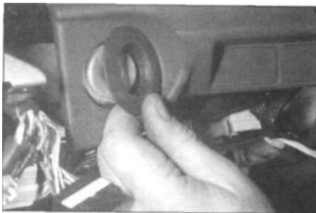
29.14 Removing the rubber grommet from the ignition switch/lock
