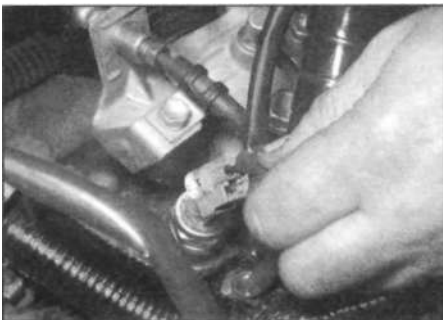
6.5 Disconnect the wiring plug from the reversing light switch
