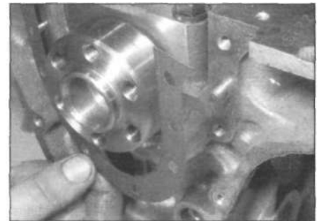
10.1d ... and recover the gasket
