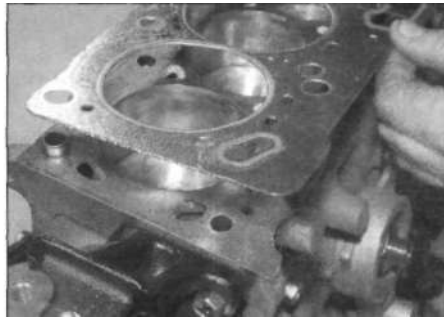
9.46 Locating a new gasket on the cylinder block
