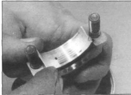
9.8 Recovering the upper half bearing shell from the connecting rod
