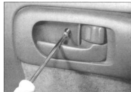
12.25 Rear door inner trim panel retaining screw removal
