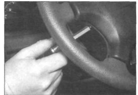
17.8 Using a suitable Torx bit, undo the screws securing the air bag module to the steering wheel...
