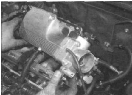
9.19 Removing the air chamber from the inlet manifold
