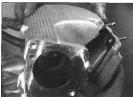
14.6b Removing the air inlet chamber cover...
