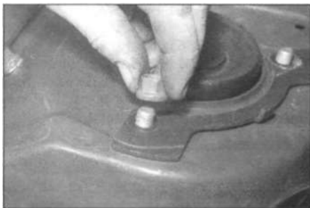
4.4a Unscrew the three nuts securing the top of the suspension strut to the vehicle body...
