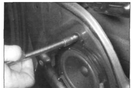
19.3 Removing the rear door-mounted loudspeaker
