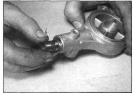
12.4c ... and valve piston from the oil pressure regulating valve
