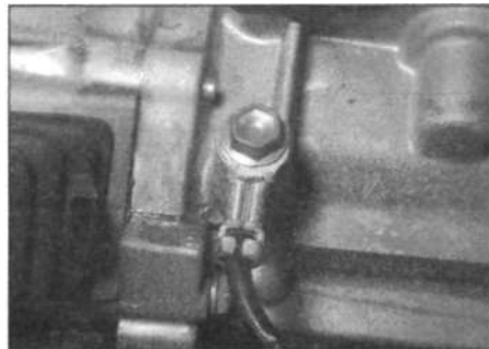
6.6 Unbolt the earth lead from the transmission
