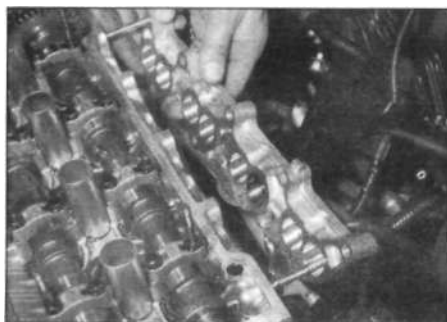
9.24b ... the intake air control valve assembly...
