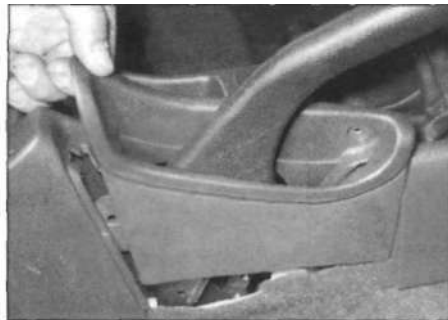
28.3b ... and withdraw the cover from the top of the handbrake lever
