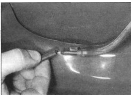
8.2 Disconnecting the windscreen washer fluid supply hose
