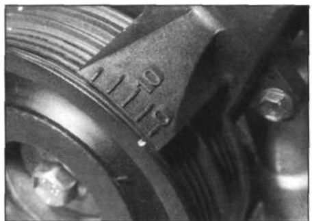
3.3 Timing marks on the crankshaft pulley and lower timing belt cover
