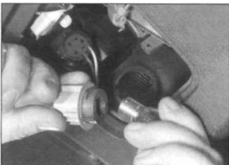
5.39b ... then depress and twist the bulb to remove it
