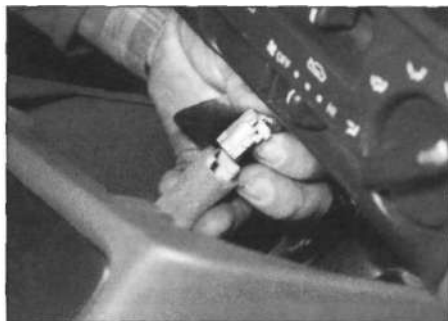
28.4c ... and disconnect the wiring from the cigar lighter
