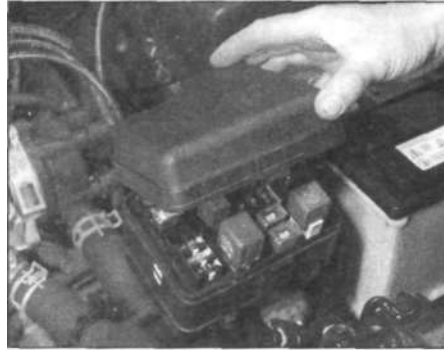
3.3b ... and remove the cover
