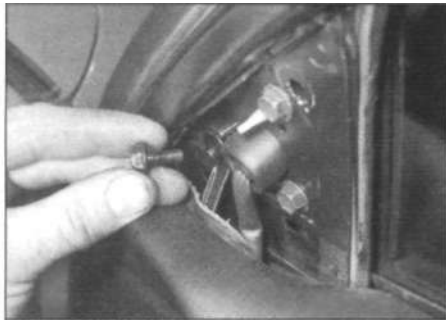
12.16 Trim panel upper mounting bolt removal
