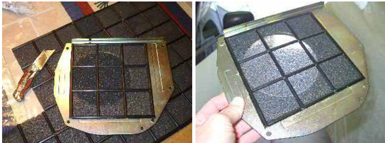
Above: I cut a section easily enough with a utility knife and glued it to the brass fan plate with DAP Contact Cement (also sold at ACE.) As you can see below it looks as though it was ment to be there. I'll check it in a few months for lint build-up and adhesion and post the results here... Fingers crossed!
