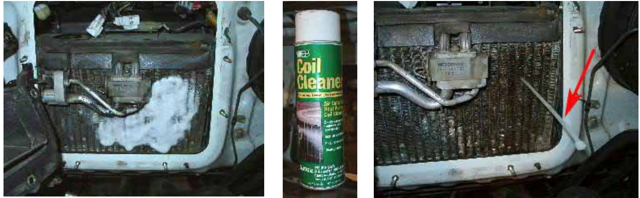
Above: The lower part of the vent box is shown after it is removed by unscrewing six nuts, two on each side and two at the bottom. Top red arrow shows electrical couplings that need to be unplugged. Bottom red arrow shows a coupling that needs to be removed from its bracket to give the vent box more room to swing to the side. I tried but could not unplug this coupling.
