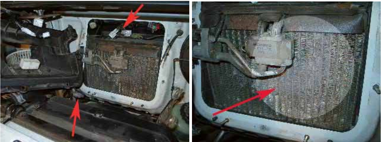
Above: The lower part of the vent box is shown after it is removed by unscrewing six nuts, two on each side and two at the bottom. Top red arrow shows electrical couplings that need to be unplugged. Bottom red arrow shows a coupling that needs to be removed from its bracket to give the vent box more room to swing to the side. I tried but could not unplug this coupling.
