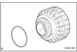
(c) Remove the O-ring from the clutch drum sub-assembly.
