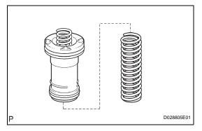
(b) Install the spring and accumulator piston into the hole.
