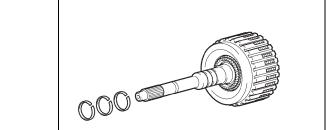
14. INSTALL INPUT SHAFT OIL SEAL RING
