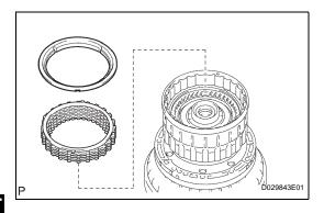
(b) Remove the reverse clutch reaction sleeve, clutch cushion plate, reverse clutch flange, 5 reverse clutch discs, and 4 clutch plates from the reverse clutch hub sub-assembly.
