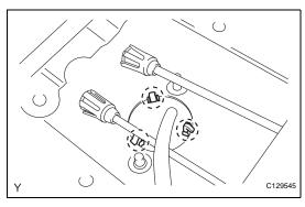
(c) Engage the 3 claws to connect the control cable.
