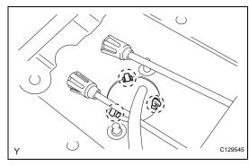
(c) Disengage the 3 claws and disconnect the control cable.
