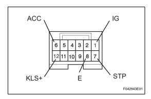
(b) Using an ohmmeter, measure the resistance at terminal E (8) and body ground. HINT:
