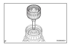
(b) Remove the input shaft assembly from the clutch drum assembly.
