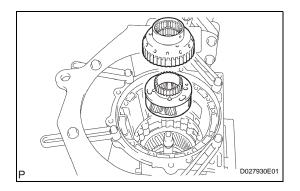
(c) Install the front planetary gear assembly and 1-way clutch inner race into the case.
