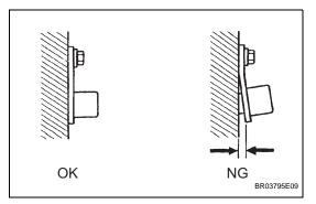
(a) Check the speed sensor (NT) installation.
