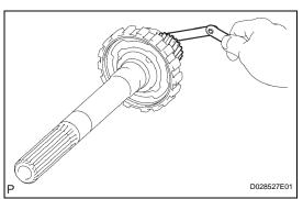
(b) Using a micrometer, check the outer diameter of the intermediate shaft positions shown in the diagram.
