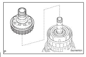
(b) Remove the reverse clutch hub sub-assembly, reverse clutch reaction sleeve, clutch cushion plate reverse clutch flange, 5 reverse clutch discs and 4 clutch plates from the clutch drum assembly.
