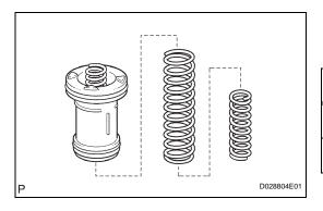
(b) Install the 2 springs and accumulator piston into the hole.
