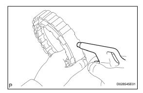
(c) Hold the 2nd brake piston and apply compressed air (392 kPa, 4.0 kgf/cm<sup>2</sup>, 57 psi) to the brake cylinder to remove the 2nd brake piston.
