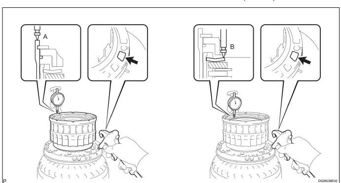
(b) If the pack clearance is outside the standard, select and install a clutch flange that makes the pack clearance within the standard.
