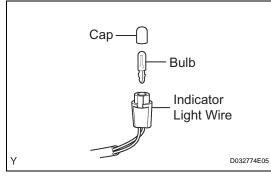
(b) Connect the indicator light wire connector onto the shift lever assembly.
