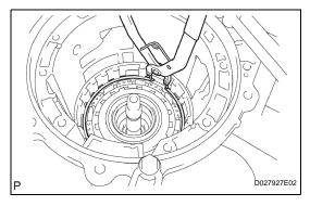
(b) Using SST, install the snap ring.
