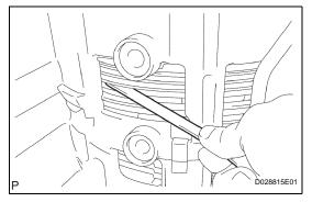
(b) Using a feeler gauge, measure the B3 brake pack clearance between the snap ring and flange.Piston stroke:
