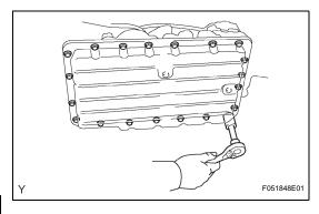
4. INSTALL AUTOMATIC TRANSMISSION OIL PAN SUB-ASSEMBLY
