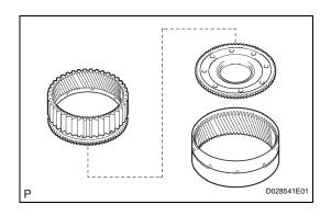
(b) Remove the center planetary ring gear and front planetary ring gear flange from the front planetary ring gear.
