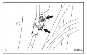
(b) Connect the control cable to the body with the 2 nuts.
