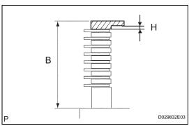
(c) Using vernier calipers, measure the thickness (length B) of the 2 brake flanges, the 7 No. 4 brake plates and the 8 No. 4 brake discs altogether at both ends across a diameter, and calculate the average. HINT:
