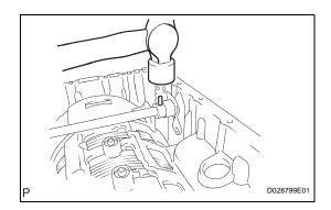
(c) Using a hammer, tap in a new spring pin.
