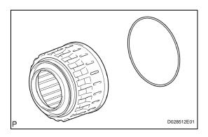
(b) Coat a new O-ring with ATF, and install it onto the reverse clutch piston sub-assembly.
