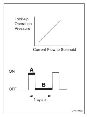
The current flow to the solenoid is controlled by the duty ratio\* of the ECM output signal. The higher the duty ratio becomes, the higher the lock-up hydraulic pressure becomes during the lock-up operation.
