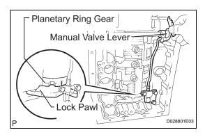
(b) Shift the manual valve lever to the P position, and confirm that the planetary ring gear is correctly locked up by the lock pawl.
