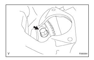
(b) Install the 6 torque converter clutch mounting bolts.
