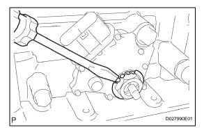
(f) Using a screwdriver, bend the tabs of the lock washer.
