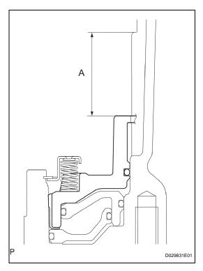
(b) Using vernier calipers, measure the level difference (length A) between the upper surface of the 1st and reverse brake piston and the hitting surface of the No. 4 brake flange at both ends across a diameter, and calculate the average.
