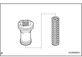
(b) Install the spring and accumulator piston into the hole.
