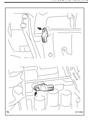
(b) Install the 2 transmission revolution sensors with the 2 bolts.
