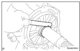
(c) Using a feeler gauge, measure the clearance between the snap ring and the race.
