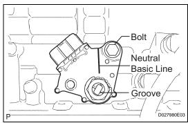
(e) Align the neutral basic line with the switch groove as shown in the illustration, and tighten the adjusting bolt
