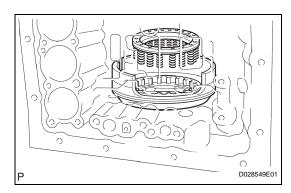
(d) Place the 1st and reverse brake return spring onto the 1st and reverse brake piston.
