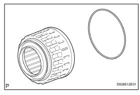
(b) Remove the O-ring from the reverse clutch piston sub-assembly.
