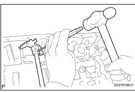
(b) Using a pin punch and hammer, tap out the spring pin.
