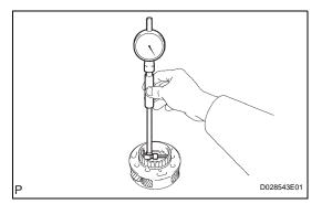
(b) Using a dial indicator, measure the inside diameter
