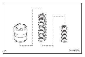
(b) Install the 2 springs and accumulator valve into the
