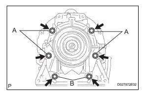
(g) Install the extension housing with 6 bolts. Torque: 34 N\*m (345 kgf\*cm, 25 ft.\*lbf) HINT:
