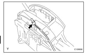
(b) Disconnect the indicator light wire from the position indicator housing lower.
