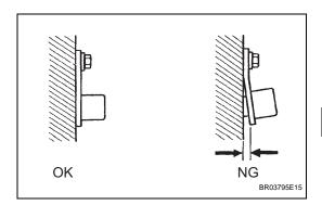
(a) Check the speed sensor (SP2) installation.
