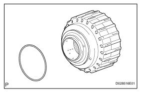
(d) Remove the O-ring from the clutch drum.
