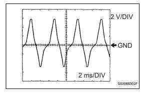
Check the waveform between terminals NT+ and NT- of the ECM connector.
