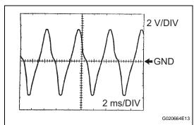
Check the waveform between terminals SP2+ and SP2- of the ECM connector.
