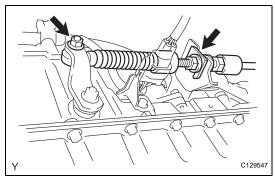
(e) Remove the nut and clip then disconnect the control cable.
