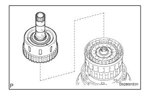
(b) Install the forward clutch hub sub-assembly onto the clutch drum assembly.
