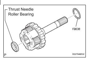
(b) Remove the No. 9 thrust bearing race and the thrust needle roller bearing from the rear planetary gear assembly.
