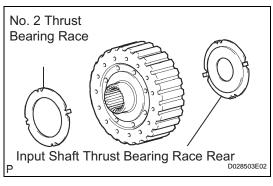
(b) Remove the No. 2 thrust bearing race and input shaft thrust bearing race rear from the multiple disc clutch hub.
