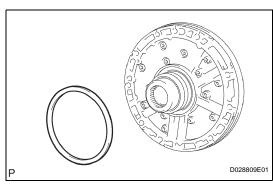
(c) Remove the No. 1 thrust bearing race from the front oil pump.
