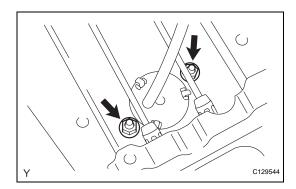
(b) Remove the 2 nuts and disconnect the control cable from the vehicle body.
