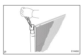
(b) Using pliers, remove the cooler dryer.
