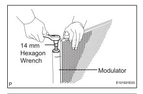
(c) Using a 14 mm straight hexagon wrench, install the cap onto the modulator.
