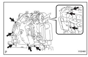
(b) Remove the 8 screws and separate the heater case.
