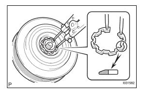
(d) Using SST, install the magnet clutch rotor and a new snap ring with the chamfered side facing up. NOTICE:
