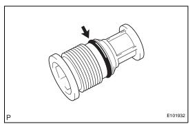
(b) Apply sufficient compressor oil to the O-ring and the fitting surface of the cap.
