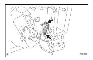
(f) Install the plate with the 2 screws.
