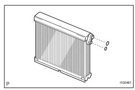
(c) Remove the cooler evaporator.
