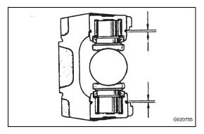
(e) Install 4 new snap rings of equal thickness which will allow no axial play.
