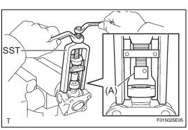
(d) Using SST, push out the spider bearing from the propeller shaft.
