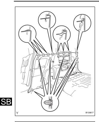
(2) Disengage the 6 clips and the 8 claws and remove the deck trim side panel.
