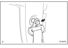
22. REMOVE REAR SEAT OUTER BELT ASSEMBLY (a) Remove the bolt and the through anchor.
