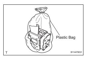
(h) Dispose of the front seat outer belt (with the seat belt pretensioner).
