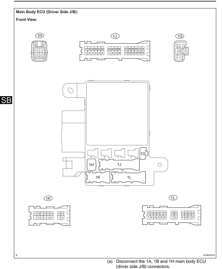
(b) Measure the voltage and resistance of the wire harness side connectors.
