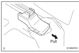
(c) Lift up on the area where the claw was removed. Then push in the direction of the claw on the opposite side to remove the outside claw.
