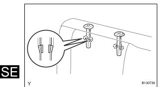
(b) Disengage the 2 claws and remove the rear seat headrest support.HINT:Use the same procedure for both sides.
