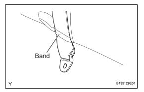
(b) Disengage the 2 claws and remove the rear seat headrest support. HINT:
