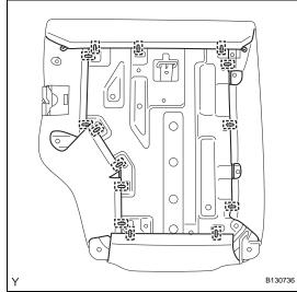
9. **REMOVE REAR SEAT HEADREST SUPPORT** (a) Remove the 14 hog rings.
