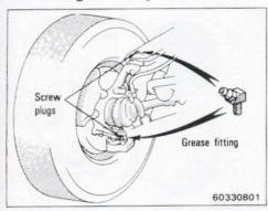
1. Remove the screw plug and temporarily screw on a standard grease fitting.
