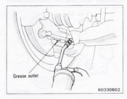
2. With a grease gun, pump molybdenumdisulfide lithium base chassis grease (NLGI No. 1 or 2) into the fitting until it begins to flow from the grease outlet in the rubber dust boot. Remove the grease fitting and reinstall the screw plug.
