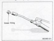
Wipe off each grease fitting. With a grease gun, pump chassis grease into each fitting until it begins to flow from the grease outlet or from around the oil seal. Remove the grease gun.
