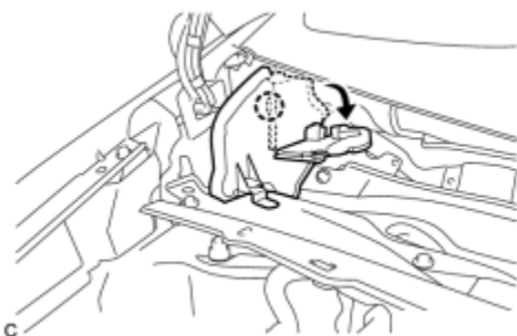
(b) Disengage the claw and bend the No. 1 heater air duct splash shield seal.
