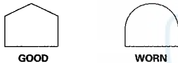
Example of synchro ring teeth
