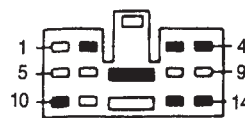
X62, 62A FRT/RH DOOR HARNESS (FRT BODY HARNESS REF.) X62 : FEMALE CONNECTOR X62A : MALE CONNECTOR
