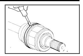
2. Remove the circlip with a flat-blade screwdriver.
