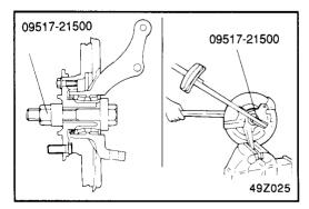
18. Measure the hub bearing starting torque.
