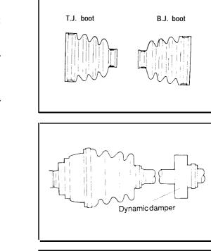
4. Apply grease into the T.J. boot and install the boot.
