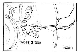
8. Disconnect the drive shaft from the hub using the special tool.
