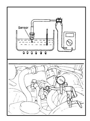
Apply a vacuum to check for a maintained vacuum when voltage applied directly to the EGR solenoid valve.
