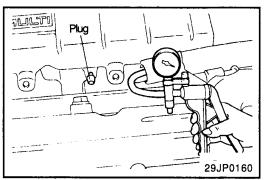
Check the following points when the engine is cold [engine coolant temperature 60°C (140°F) or below] and when it is warm [engine coolant temperature 70°C (158°F) or higher].
