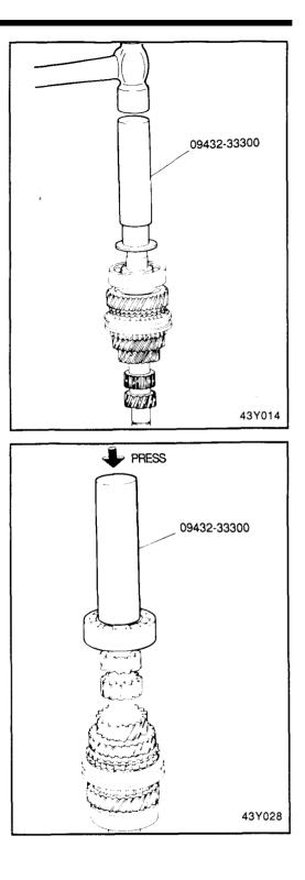
11. Install the front bearing using the special tool (09432-33300).12. Install the snap ring.
