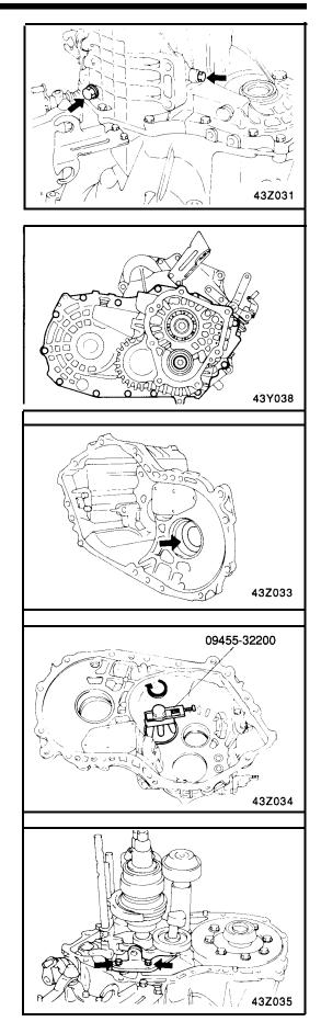
17. Remove the reverse gear shaft and reverse gear.
