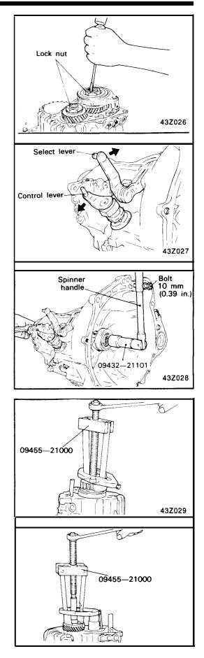
10. Remove the reverse idler gear shaft bolt and restriction ball assembly.
