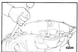
26. Remove the input shaft oil seal.
