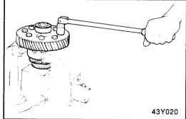
3. Remove the taper roller bearings using the special tool (09\$32-11000, 09532-11100, 09532-11301).
