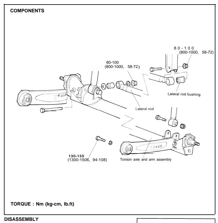
1. Drive out and press in the arm bushing using the special tool.
