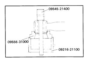
2. Press in the lateral rod bushing with the special tool. Press in the bushing so that the amount of projection is equal on either side.
