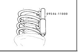
2. While holding the piston rod, remove the piston rod tightening nut.
