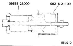
2. Drive out and press in the lateral rod bushing using the special tool.
