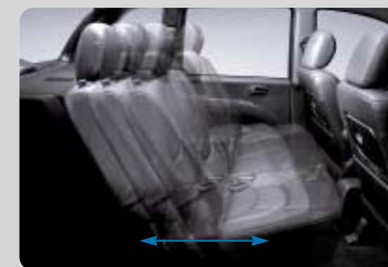
Sliding Rear Seats New seat rails permit 195mm of sliding adjustment to keep knees happy. And the seatbacks have a folding-reclining range of 23 to 58 degrees. In addition to the 60:40 split folding feature, they can be double-folded to make room for over-sized cargo. Up/down adjustable headrests are included.
