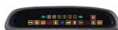
Telltale Lamps Warning icons and automatic gear shift indicator are in the driver's direct line of sight-over the steering column-for maximum visibility.
