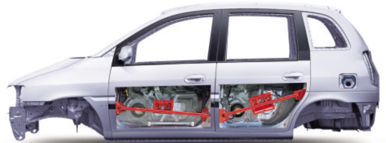
Steel Safety Cage Matrix's bodyshell has been reinforced at critical points with high-tensile strength steel to create a highly rigid safety cage. To reduce the risk of side intrusion, doors are reinforced with members made of high-tensile strength steel.
