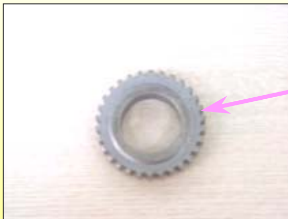
Sensing tone wheel for rear speed (teeth = 30EA)
