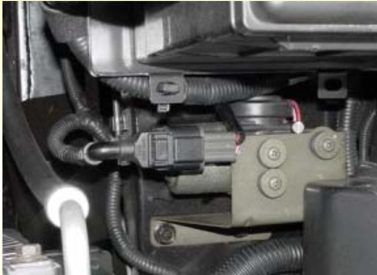
FRRD AIR PUMP CIRCUIT
