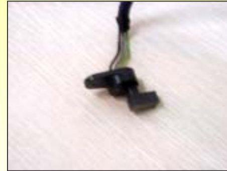
Hall effect type speed sensor
