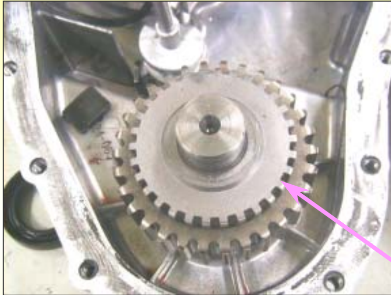
Sensing tone wheel for front speed (teeth = 30EA)
