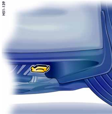
B - Rear jacking point
