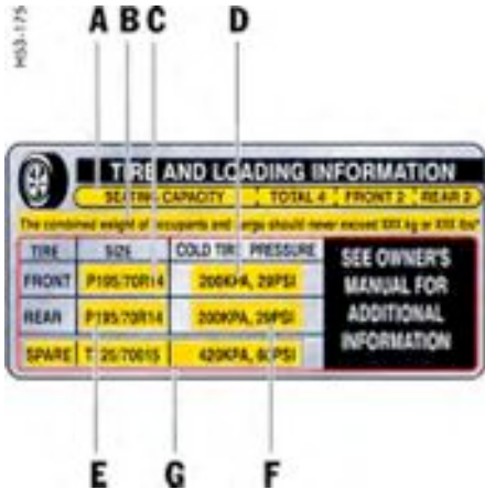
Example of a tire pressure plate
