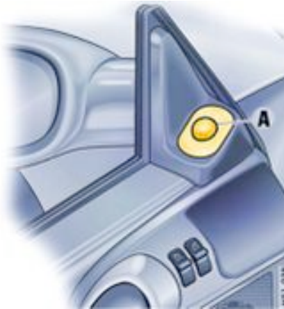
A - Control switch for door mirror adjustment
