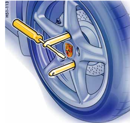
Screw in two assembly aids for vehicles with Porsche Ceramic Composite Brake
