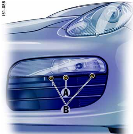
A - Fog light height adjustment B - Fastening screw
