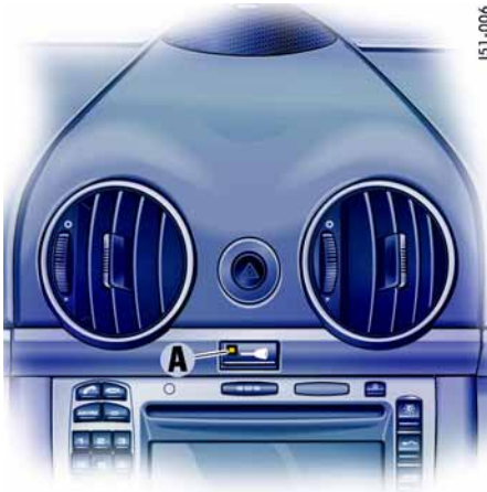
A - Light-emitting diode for alarm system
