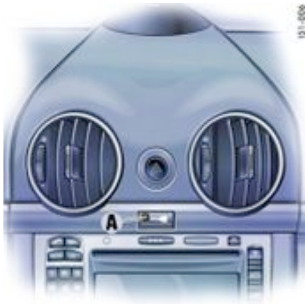
A - Light-emitting diode for alarm system
