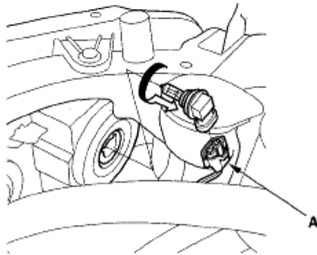
Fig. 27: Identifying 2P Connector From Headlight (SC Model) Courtesy of AMERICAN HONDA MOTOR CO., INC.
