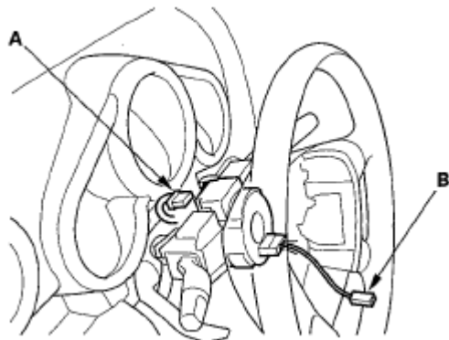
Fig. 6: Identifying Dashboard Wire Harness B 5P Connector And Horn Switch Positive 1P Connector Courtesy of AMERICAN HONDA MOTOR CO., INC.
