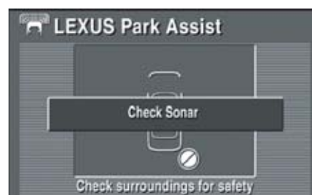
Rear right-hand side sensor Disconnection
