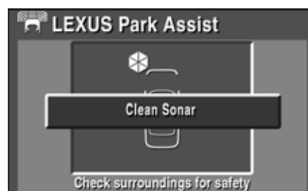
Front left-hand side sensor frozen
