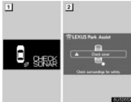
(b) When the sensor is malfunctioning
