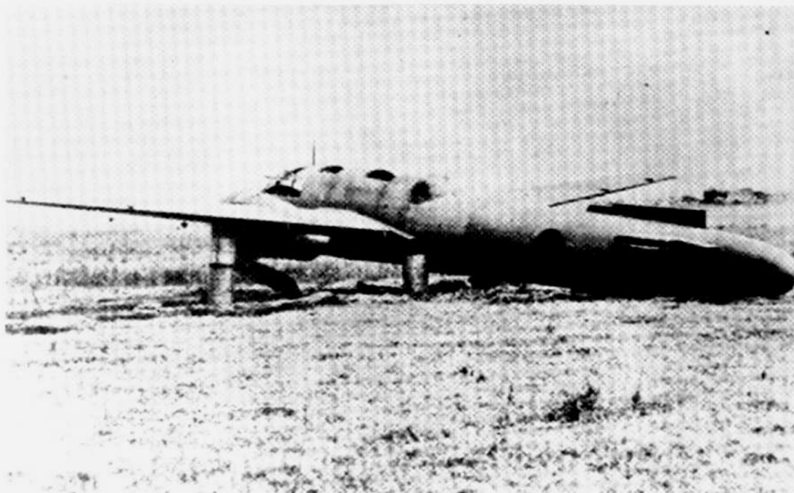
When wrecked examples of the Ki.67-I suicide bombers were found in the Philippines, American Intelligence erroneously thought the faired over aircraft were special reconnaissance versions of "Peggy." The use of a full size aircraft as a flying bomb was inconceivable at the time. USN.
