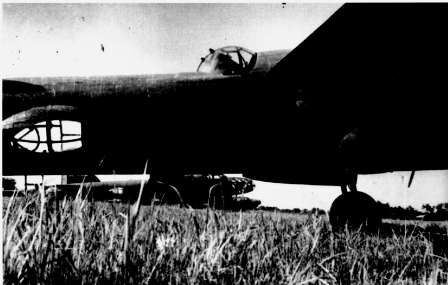
Ki.67-Ib Hiryu of the 74th Air Regiment on Formosa. Armament has been revised to carry two 12.7mm Ho.103 Type 1 MG in the dorsal turret. Mannosuke Toda.
