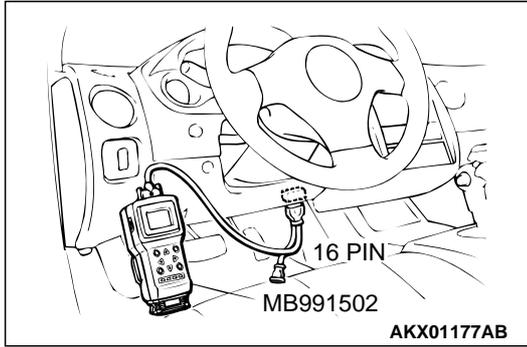
**STEP 4. Using scan tool MB991502, check data list.**
