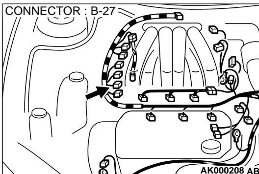
**STEP 4. Check connector B-27 at right bank heated oxygen sensor (front) and connector C-62 at ECM <M/T> or connector C-59 at PCM <A/T> for damage.**
