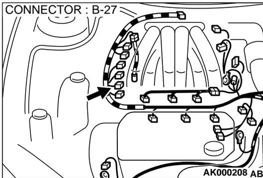
**STEP 8. Check the continuity at right bank heated oxygen sensor (front) harness side connector B-27.**
