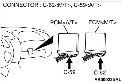
**STEP 9. Check for harness damage between left bank injector connector and ECM connector <M/T> or PCM connector <A/T>.**
