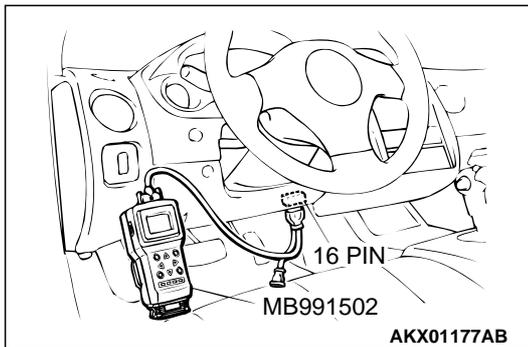
**STEP 6. Using scan tool MB991502, check data list.**
