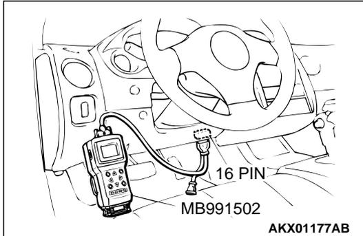
**STEP 4. Using scan tool MB991502, check data list item 13: Intake Air Temperature Sensor.**
