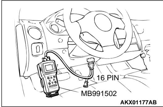
**STEP 10. Using scan tool MB991502, check data list.**
