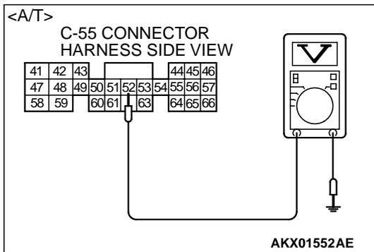
**STEP 7. Check the power supply voltage at ECM connector C-58 <M/T> or PCM connector C-55 <A/T> by backprobing**
