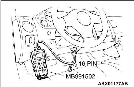
**STEP 1. Using scan tool MB991502, check data list item 11: Heated Oxygen Sensor Bank 2, Sensor 1 (left front).**
