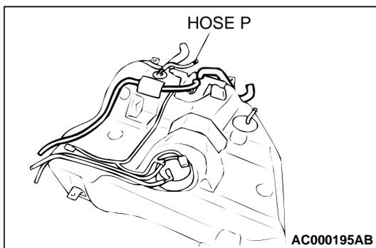
**STEP 12. Check for leaks in the evaporator line from hose P.**
