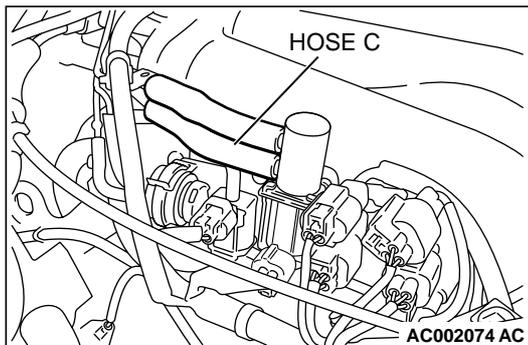
**STEP 25. Check for clogging in the evaporator line hose C to hose E.**
