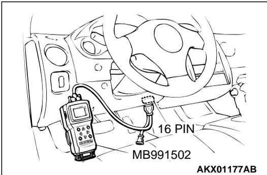
**STEP 6. Check the sensor supply voltage at ECM connector C-62 by backprobing**
