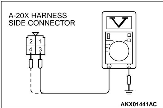
**STEP 7. Check the power supply voltage at fuel pump relay connector A-20X.**
