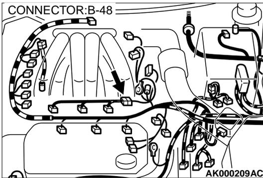
**STEP 6. Check the right bank injector resistance at intermediate connector B-48.**
