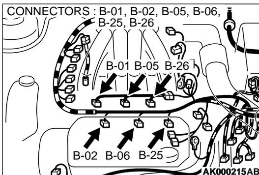
**STEP 14. Check for harness damage between injector connector and PCM connector.**
