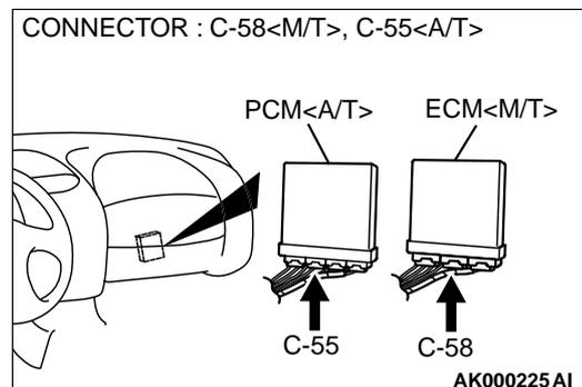
**STEP 10. Check for short circuit to ground between power steering pressure switch connector B-19 terminal 1 and ECM connector C-58 terminal 54 <M/T> or PCM connector C-55 terminal 52 <A/T>.**
