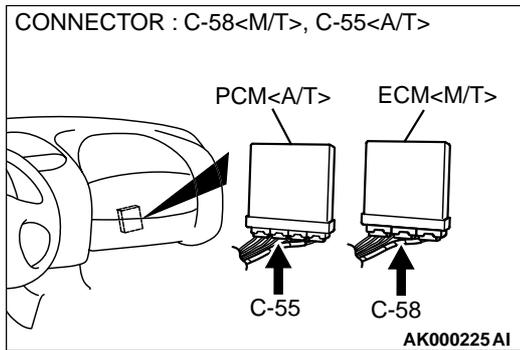
**STEP 6. Check connector B-14 at the barometric pressure sensor and connector C-58 at ECM <M/T> or connector C-55 at PCM <A/T> for damage.**
