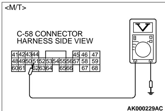
**STEP 3. Check the sensor output voltage at ECM connector C-58 <M/T> or PCM connector C-55 <A/T> by backprobing.**
