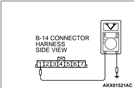
**STEP 7. Check the sensor supply voltage at barometric pressure sensor connector B-14 by backprobing.**
