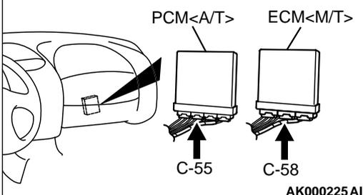
**STEP 10. Check for harness damage between generator connector B-45 terminal 4 and ECM connector C-58 terminal 52 <M/T> or PCM connector C-55 terminal 54 <A/T>.**
