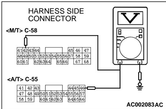
**STEP 11. Check the 5-volt supply circuit voltage at ECM connector C-58 <M/T> or PCM connector C-55 <A/T>.**
