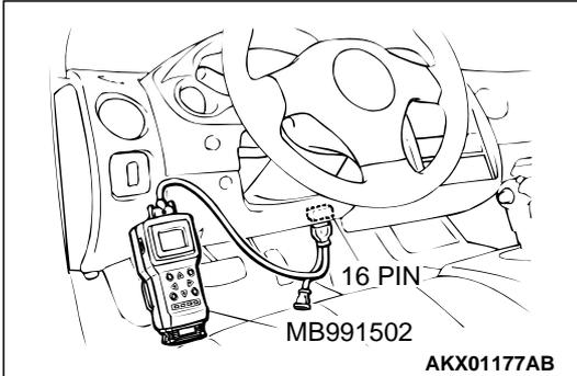
**STEP 3. Using scan tool MB991502, check data list item 39: Heated Oxygen Sensor Bank 1, Sensor 1 (right front).**
