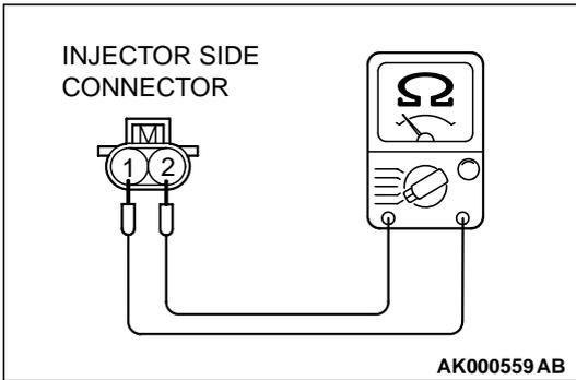
**STEP 5. Check the left bank injector.**
