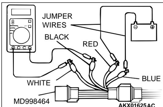
**STEP 14. Check the left bank heated oxygen sensor (front).**
