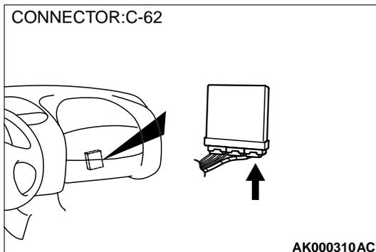
**STEP 13. Check connector C-62 at ECM for damage.**
