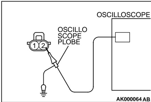
1. Disconnect the injector intermediate connector, and connect the test harness special tool (MD998464) in between.
