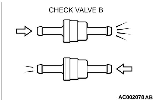
**STEP 14. Check the check valve B.**
