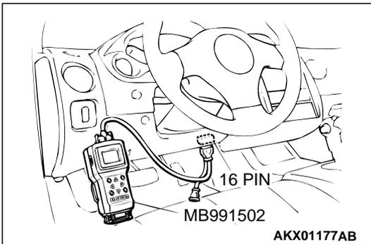
**STEP 3. Using scan tool MB991502, check data list item 82:
