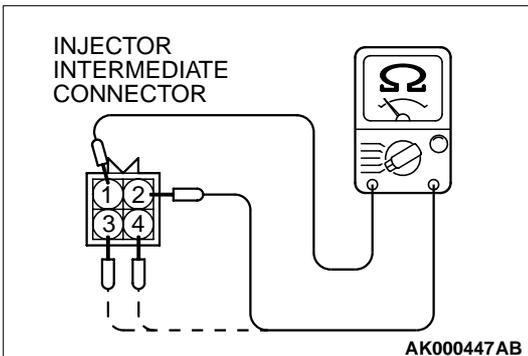
**STEP 7. Check the right bank injector resistance at injector intermediate connector B-48.**
