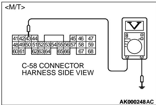
**STEP 7. Check the sensor supply voltage at ECM connector C-58 <M/T> or PCM connector C-55 <A/T> by backprobing**
