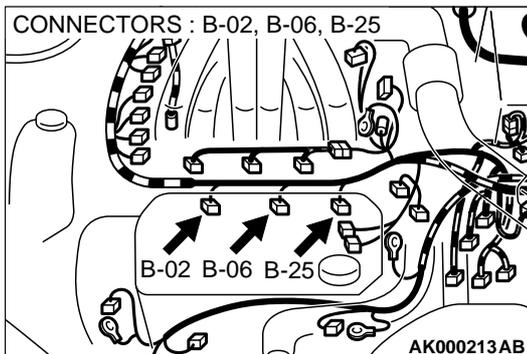
**STEP 7. Check the left bank injector.**
