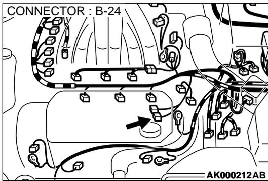
**STEP 7. Check connector B-24 at left bank heated oxygen sensor (front) for damage.**
