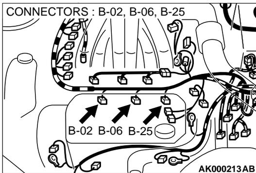
**STEP 7. Replace the left bank injector.**
