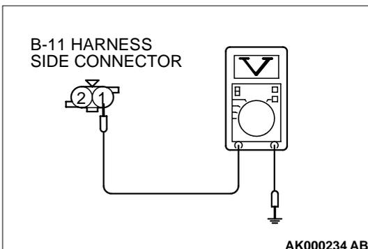
**STEP 6. Check the sensor supply voltage at engine coolant temperature sensor harness side connector B-11.**
