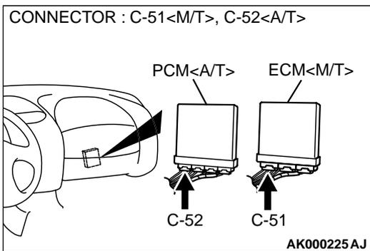
**STEP 8. Check for open circuit and short circuit to ground between EGR solenoid connector B-31 terminal 2 and ECM connector C-51 terminal 6 <M/T> or PCM connector C-52 terminal 6 <A/T>.**
