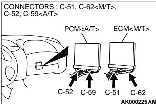
**STEP 7. Check connector C-51, C-62 at ECM <M/T> or connector C-59, C-52 at PCM <A/T> for damage.**
