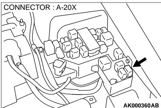
**STEP 5. Check connector A-20X at fuel pump relay for damage.**
