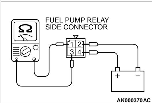
**STEP 6. Check the fuel pump relay**
