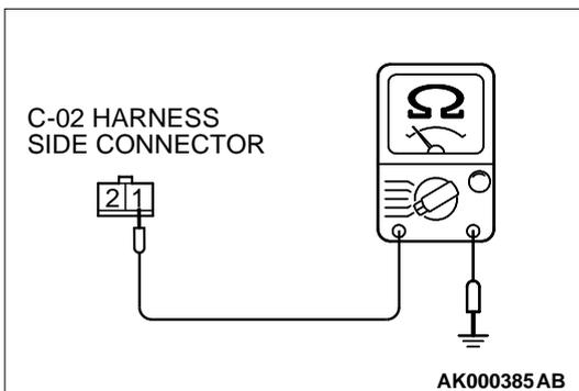
**STEP 9. Check the continuity at interlock switch harness side connector C-02.**
