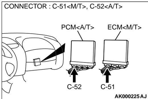
**STEP 13. Check for harness damage between injector connector and PCM connector.**
