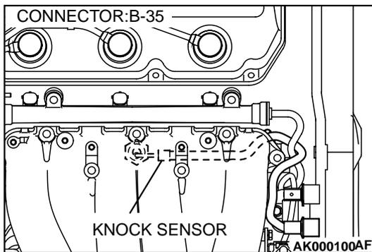
**STEP 4. Check for open circuit, short circuit to ground and harness damage between knock sensor connector B-35 terminal 1 and ECM connector C-62 terminal 91 <M/T> or PCM connector C-59 terminal 90 <A/T>.**
