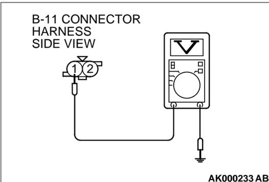
**STEP 3. Check connector B-11 at the engine coolant temperature sensor for damage.**
