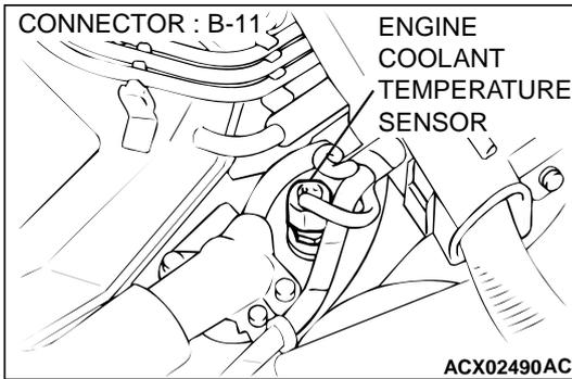
**STEP 8. Check for open circuit between engine coolant temperature sensor connector B-11 terminal 2 and ECM connector C-58 terminal 49 <M/T> or PCM connector C-55 terminal 57 <A/T>.**
