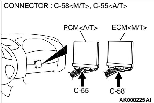
**STEP 10.** Check connector B-14 at the barometric pressure sensor and connector C-58 at ECM <M/T> or connector C-55 at PCM <A/T> for damage.
