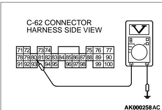
**STEP 7. Check connector C-62 at ECM for damage.**
