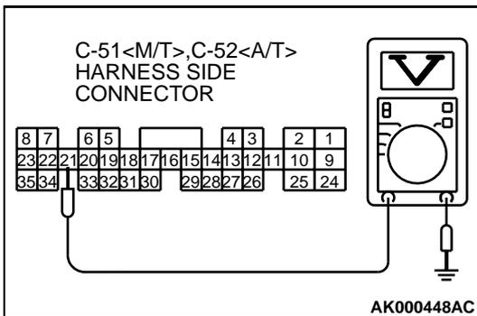
**STEP 10. Check the power supply voltage at ECM connector C-51 <M/T> or PCM connector C-52 <A/T>.**
