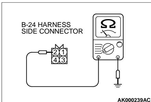
**STEP 8. Check the continuity at left bank heated oxygen sensor (front) harness side connector B-24.**
