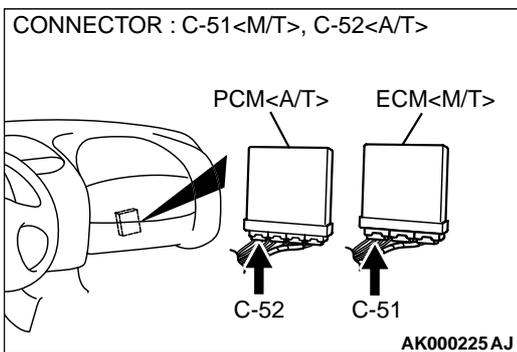
**STEP 14. Check connector C-51 at ECM <M/T> or connector C-52 at PCM <A/T> for damage.**
