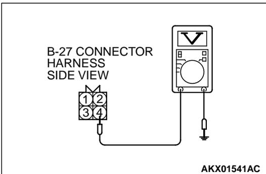
**STEP 2. Check the sensor output voltage at right bank heated oxygen sensor (front) connector B-27 by backprobing.**
