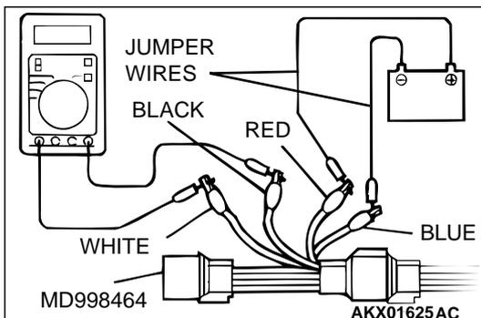
**STEP 14. Check the right bank heated oxygen sensor (front).**
