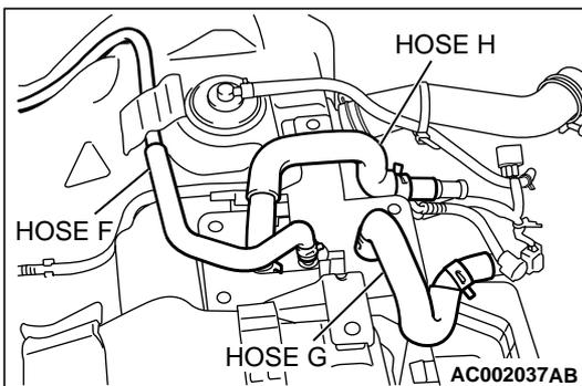
**STEP 7. Check for leaks in the evaporative emission canister.**
