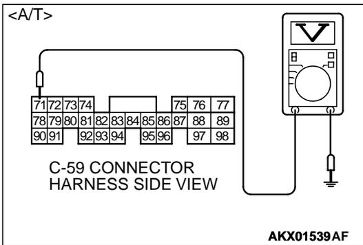
**STEP 4. Check connector B-24 at left bank heated oxygen sensor (front) and connector C-62 at ECM <M/T> or connector C-59 at PCM <A/T> for damage.**
