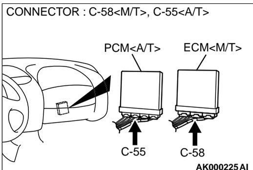
**STEP 11.** Check for short circuit to ground between barometric pressure sensor connector B-14 terminal 1 and ECM connector C-58 terminal 42 <M/T> or PCM connector C-55 terminal 46 <A/T>.
