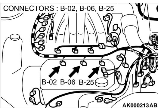
**STEP 8. Check the left bank injector.**
