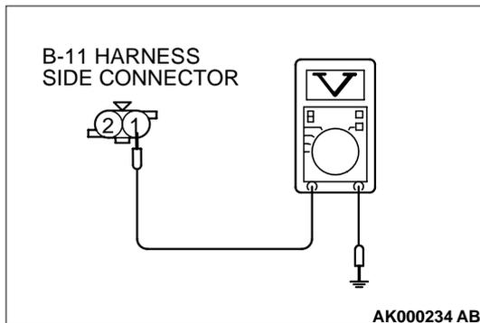
**STEP 3. Check the sensor supply voltage at engine coolant temperature sensor harness side connector B-11.**
