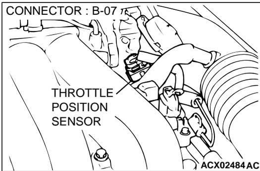
**STEP 8. Check for open circuit and harness damage between throttle position sensor connector B-07 terminal 1 and ECM connector C-58 terminal 49 <M/T> or PCM connector C-55 terminal 57 <A/T>.**
