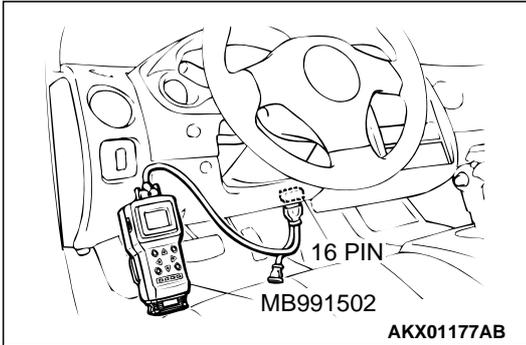
**STEP 1. Using scan tool MB991502, check data list item 69: Heated Oxygen Sensor Bank 1, Sensor 2 (right rear).**
