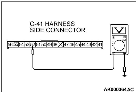
**STEP 4. Check the power supply voltage at combination meter harness side connector C-41.**
