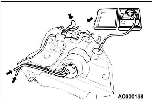
**STEP 13. Check for leaks in the fuel tank.**
