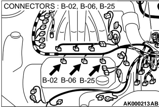
**STEP 6. Check the left bank injector.**
