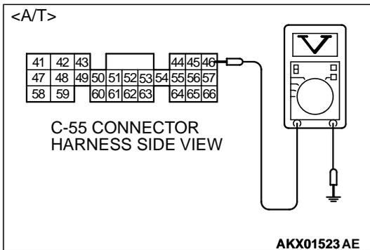
**STEP 9. Check connector B-14 at the barometric pressure sensor and connector C-58 at ECM <M/T> or connector C-55 at PCM <A/T> for damage.**
