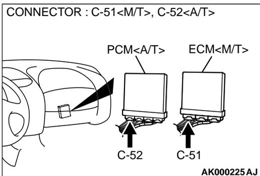
**STEP 10. Check for open circuit and short circuit to ground and harness damage between injector intermediate connector and ECM connector <M/T> or PCM connector <A/T>.**
