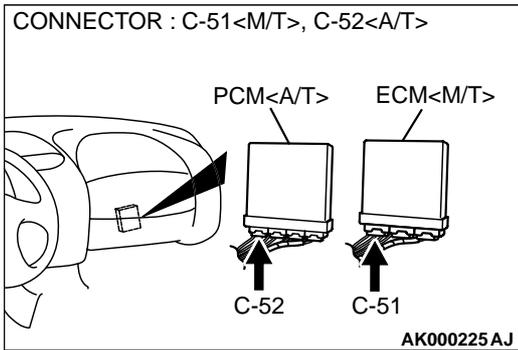
**STEP 8. Check connector C-51 at ECM <M/T> or connector C-52 at PCM <A/T> for damage.**
