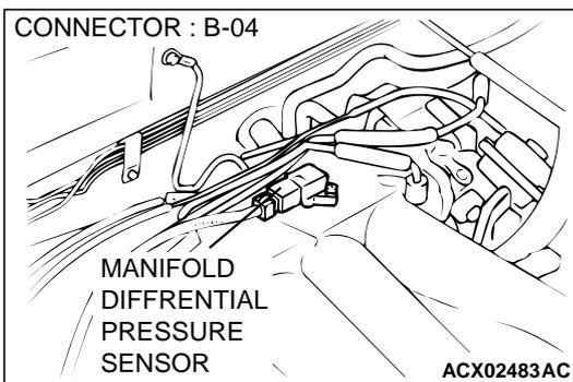
**STEP 11.** Check for open circuit and short circuit to ground and harness damage between manifold differential pressure sensor connector B-04 terminal 1 and ECM connector C-62 terminal 92 <M/T> or PCM connector D-59 terminal 91 <A/T>.
