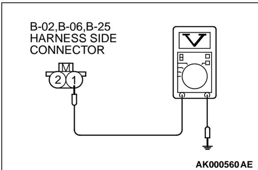
**STEP 3. Check the injector.**
