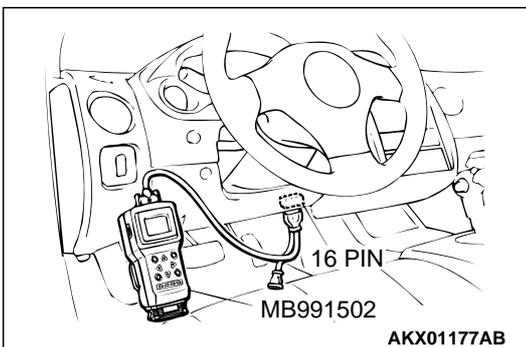
**STEP 5. Checking by operating the accelerator pedal**
