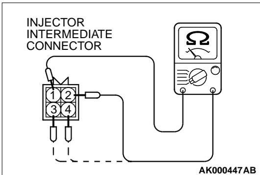
**STEP 8. Check the right bank injector resistance at injector intermediate connector B-48.**
