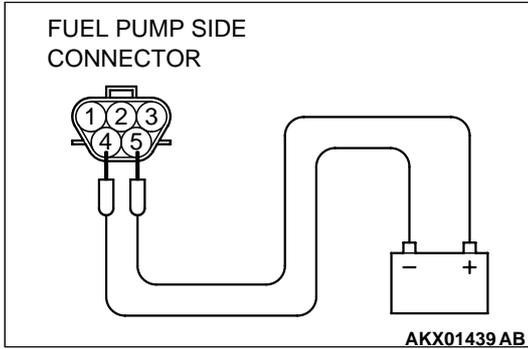
**STEP 3 Check the fuel pump operation.**
