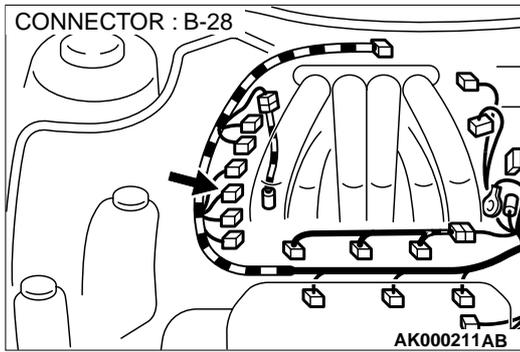
**STEP 1. Check connector B-28 at the right bank heated oxygen sensor (rear) for damage.**
