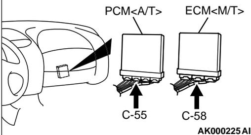
**STEP 12.** Check connector C-58 at ECM <M/T> or connector C-55 at PCM <A/T> for damage.
