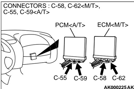
**STEP 10. Check connector C-58, C-62 at ECM <M/T> or connector C-55, C-59 at PCM <A/T> for damage.**
