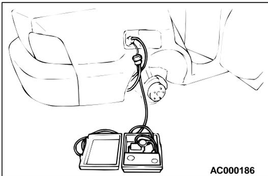
**STEP 2. Check the output circuit voltage at intermediate connector D-16.**
