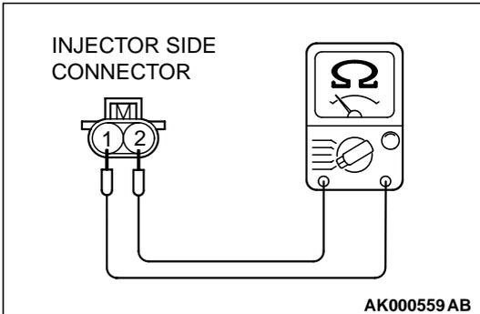
**STEP 5. Check the injector.**
