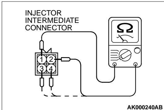
**STEP 8. Check the right bank injector resistance at intermediate connector B-48.**
