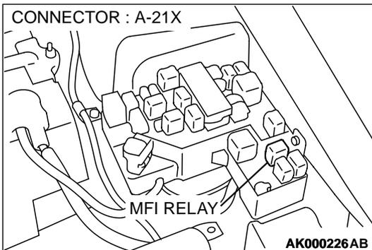
**STEP 6. Check for harness damage between MFI relay connector and injector connector.**
