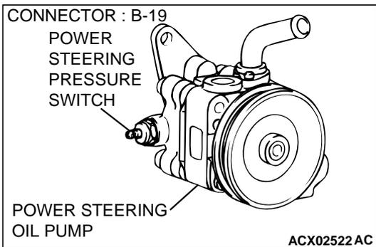
**STEP 3. Check connector B-19 at power steering pressure switch for damage.**
