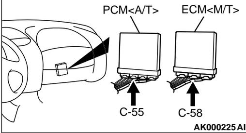
**STEP 10.** Check connector C-58 at ECM <M/T> or connector C-55 at PCM <A/T> for damage.
