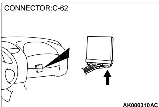
**STEP 15. Check for harness damage between vehicle speed sensor connector B-39 terminal 3 and ECM connector C-62 terminal 80.**
