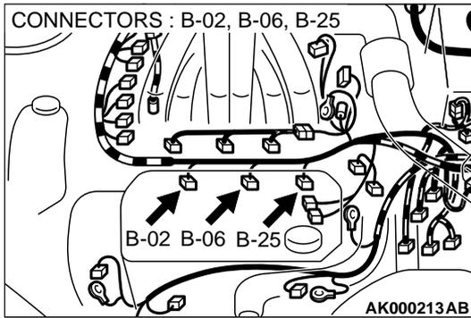
**STEP 8. Check the left bank injector.**
