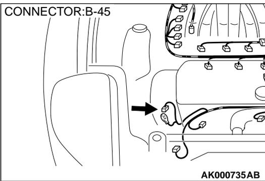
**STEP 3. Check connector B-45 at generator connector for damage.**
