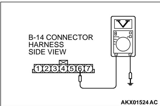
**STEP 3. Check connector B-14 at the intake air temperature sensor for damage.**
