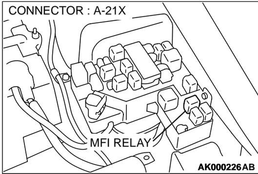
**STEP 7. Check connector A-21X at MFI relay for damage.**
