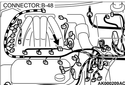
**STEP 11. Check connector B-48 at injector intermediate connector for damage.**
