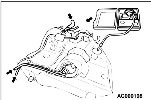
**STEP 17. Check for leaks in the fuel tank.**
