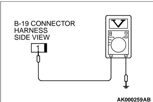
**STEP 2. Check the power supply voltage at power steering pressure switch connector B-19 by backprobing**
