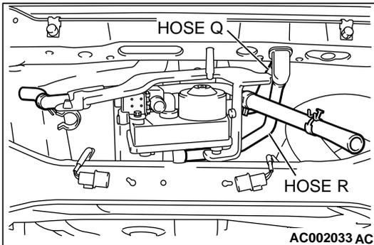
**STEP 23. Check for clogging in the evaporator lines I.**
