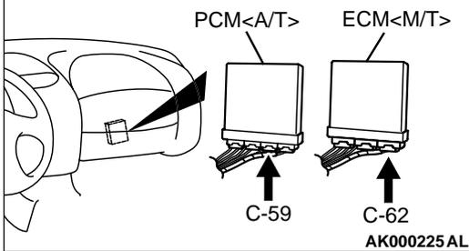
**STEP 11. Check for harness damage between right bank injector connector and ECM connector <M/T> or PCM connector <A/T>.**
