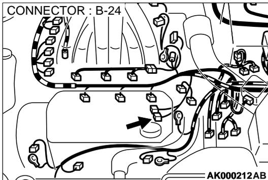
**STEP 10. Check for harness damage between left bank heated oxygen sensor (front) connector B-24 terminal 3 and ECM connector C-51 terminal 3 <M/T> or PCM connector C-52 terminal 3 <A/T>.**
