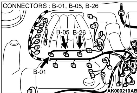
**STEP 9. Check connector B-01 or B-05 or B-26 at right bank injector for damage.**
