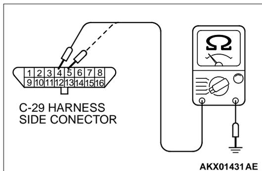
INSPECTION PROCEDURE 2: Scan Tool Communication with ECM or PCM Is Not Possible.
