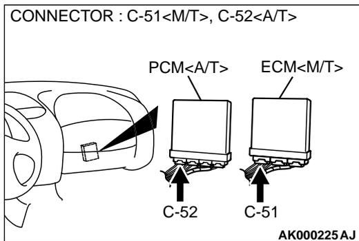
**STEP 10. Check for harness damage between left bank injector connector and ECM connector <M/T> or PCM connector <A/T>.**
