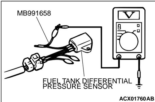
**STEP 9. Check the output voltage at fuel tank differential pressure sensor connector D-18.**
