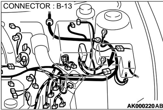
**STEP 4. Check connector B-13 at generator intermediate connector for damage.**
