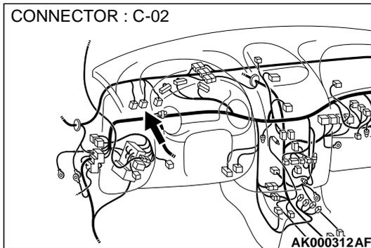
**STEP 6. Check connector C-02 at interlock switch for damage.**
