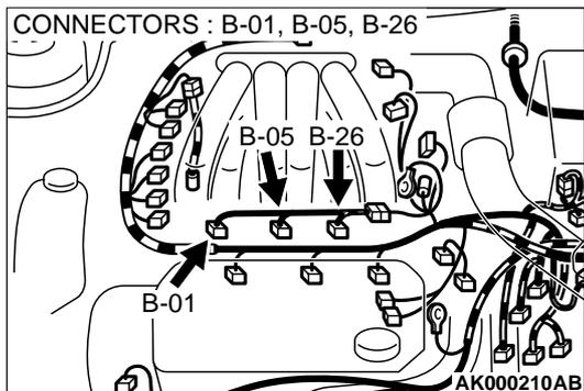
**STEP 9. Check connector B-01, B-05, B-26 at right bank injector for damage.**
