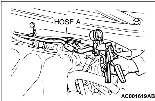
**STEP 2. Check for leaks in the evaporator line hose A.**
