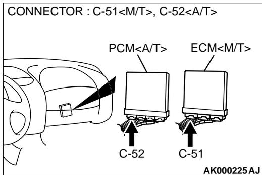
**STEP 4.** Check for short circuit to ground between volume air flow sensor connector B-14 terminal 7 and ECM connector C-51 terminal 19 <M/T> or PCM connector C-52 terminal 19 <A/T>.
