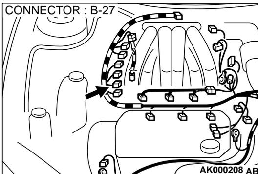
**STEP 10. Check for harness damage between right bank heated oxygen sensor (front) connector B-27 terminal 3 and ECM connector C-51 terminal 4 <M/T> or PCM connector C-52 terminal 4 <A/T>.**
