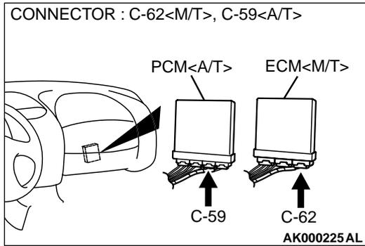
**STEP 11. Check for open circuit and short circuit to ground between throttle position sensor connector B-07 terminal 3 and ECM connector C-62 terminal 78 <M/T> or PCM connector C-69 terminal 78 <A/T>.**
