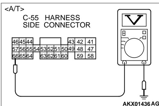
**STEP 3. Check the backup power supply voltage at ECM connector C-58 <M/T> or PCM connector C-55 <A/T> by backprobing.**
