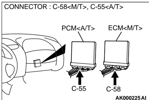
**STEP 10. Check for open circuit and harness damage between right bank heated oxygen sensor (front) connector B-27 terminal 2 and ECM connector C-58 terminal 49 <M/T> or PCM connector C-55 terminal 57 <A/T>.**
