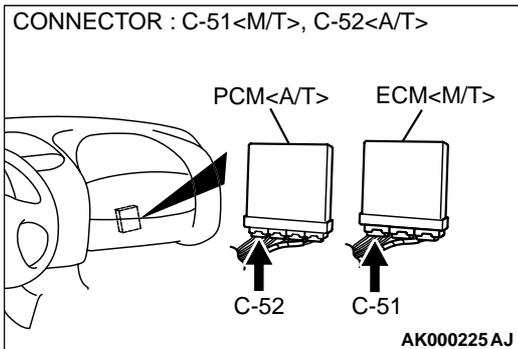
**STEP 4. Check connector C-51 at ECM <M/T> or connector C-52 at PCM <A/T> for damage.**
