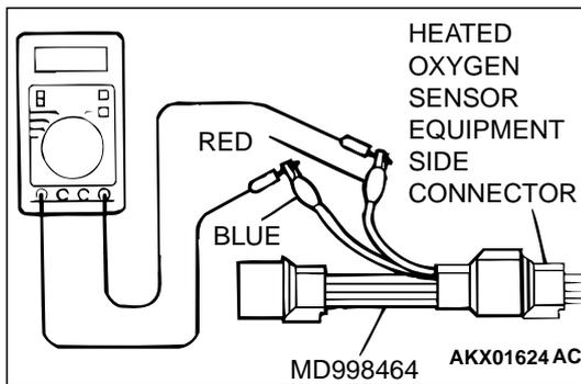
**STEP 3. Check the power supply voltage at left bank heated oxygen sensor (front) harness side connector B-24.**
