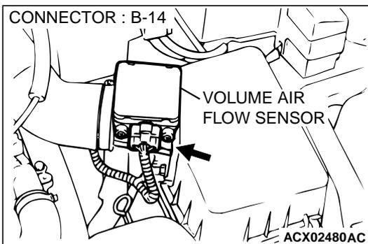
**STEP 5. Check connector B-14 at volume air flow sensor for damage.**
