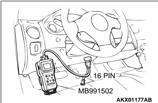
**STEP 9. Using scan tool MB991502, check data list.**
