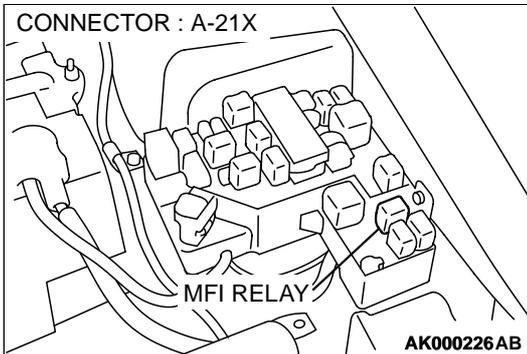
**STEP 10. Check for harness damage between MFI relay connector A-21X terminal 1 and EGR solenoid connector B-31 terminal 1.**
