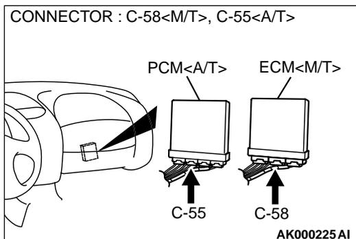
**STEP 17. Check for short circuit to ground and harness damage between barometric pressure sensor connector B-14 terminal 2 and ECM connector C-58 terminal 51 <M/T> or PCM connector C-55 terminal 55 <A/T>.**
