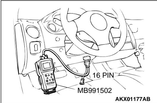
**STEP 1. Using scan tool MB991502, check data list item 27: Power Steering Pressure Switch.**
