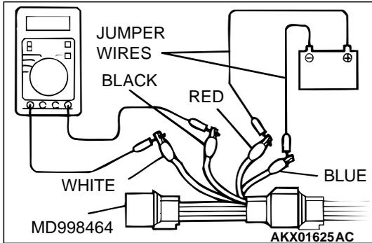
**<Right bank and left bank heated oxygen sensor (front)>**
