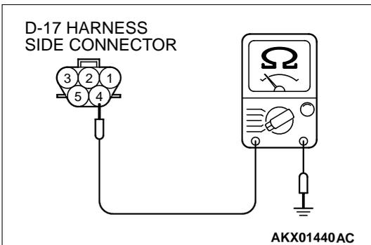
**STEP 4. Check the continuity at fuel pump harness side connector D-17.**
