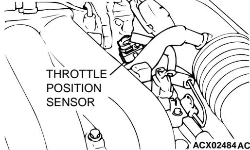
**STEP 5. Check for open circuit and short circuit to ground between throttle position sensor connector B-07 terminal 4 and ECM connector C-58 terminal 42 <M/T> or PCM connector C-55 terminal 46 <A/T>.**
