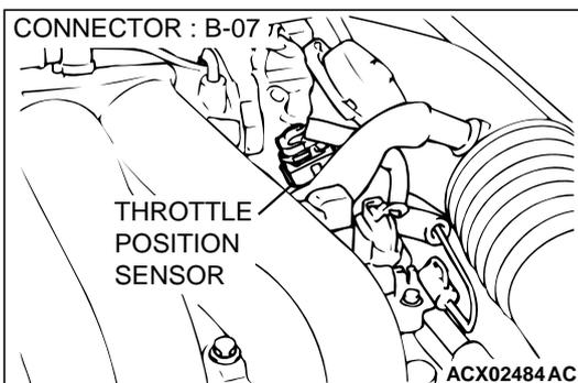
**STEP 3. Check the sensor supply voltage at throttle position sensor harness side connector B-07.**
