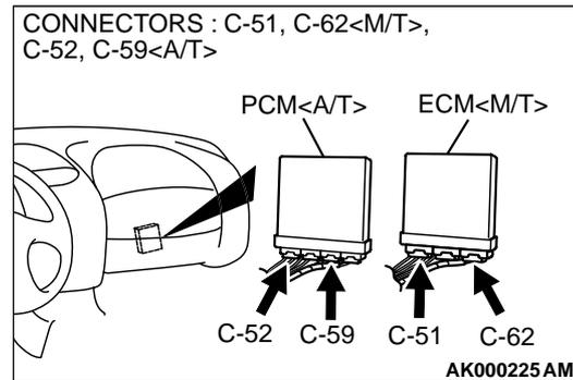
**STEP 9. Check connector C-51, C-62 at ECM <M/T> or connector C-52, C-59 at PCM <A/T> for damage.**
