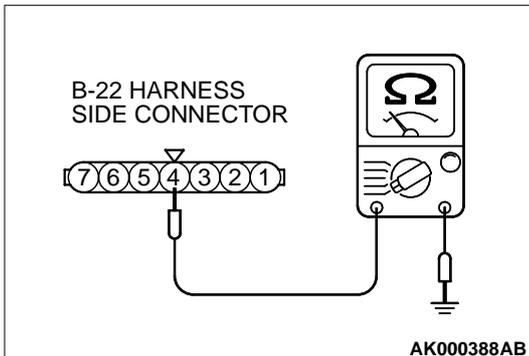
**STEP 5. Check the continuity at distributor harness side connector B-22.**
