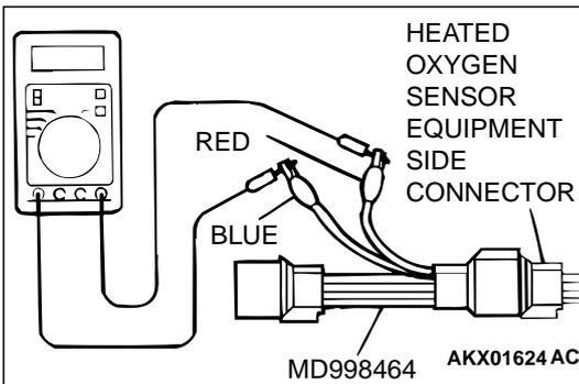
**STEP 2. Check the right bank heated oxygen sensor (front).**
