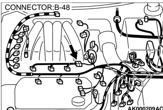
**STEP 4. Check connector at injector and injector intermediate connector for damage.**
