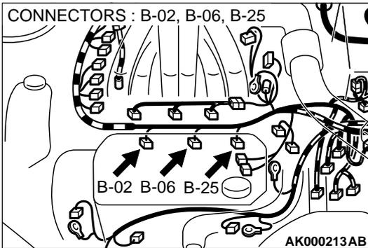
**STEP 12. Check connector B-02, B-06, B-25 at left bank injector for damage.**
