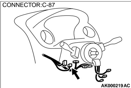
**STEP 14. Check for harness damage between ignition switch connector C-87 terminal 2 and vehicle speed sensor connector B-39 terminal 1.**
