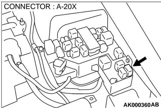
**STEP 8. Check for open circuit and short circuit to ground and harness damage between fuel pump relay connector A-20X terminal 1 and fuel pump connector D-17 terminal 5.**
