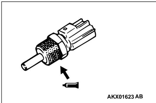
**STEP 9. Check the engine coolant temperature sensor.**
