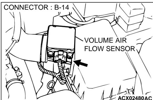
**STEP 7. Check for open circuit and harness damage between volume air flow sensor connector B-14 terminal 7 and ECM connector C-51 terminal 19 <M/T> or PCM connector C-52 terminal 19 <A/T>.**
