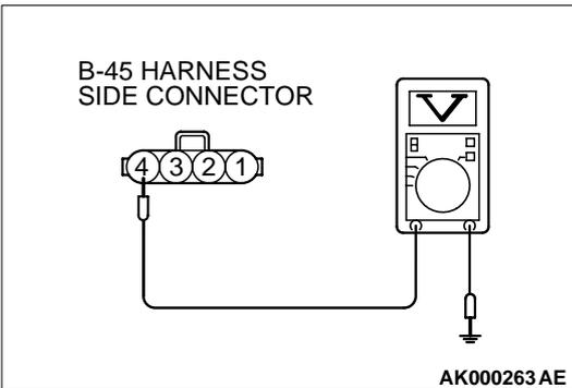
**STEP 6. Check the voltage at generator harness side connector B-45.**
