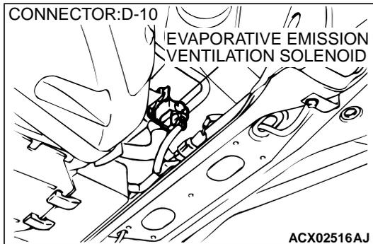
**STEP 11. Check for harness damage between evaporative emission ventilation solenoid connector D-10 terminal 1 and ECM connector C-51 terminal 35 <M/T> or PCM connector C-52 terminal 35 <A/T>.**
