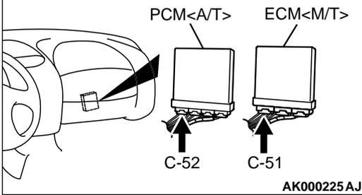
**STEP 9. Check connector C-51 at ECM <M/T> or connector C-52 at PCM <A/T> for damage.**
