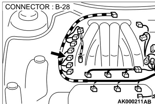
**STEP 10. Check for harness damage between right bank heated oxygen sensor (rear) connector B-28 terminal 3 and ECM connector C-51 terminal 27 <M/T> or PCM connector C-52 terminal 27 <A/T>.**
