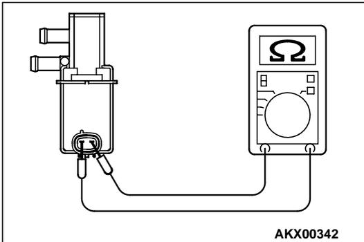
**STEP 3. Check the evaporative emission purge solenoid.**
