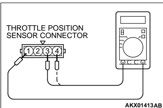
**STEP 7. Check for open circuit and harness damage between throttle position sensor connector B-07 terminal 1 and ECM connector C-58 terminal 49 <M/T> or PCM connector C-55 terminal 57 <A/T>.**
