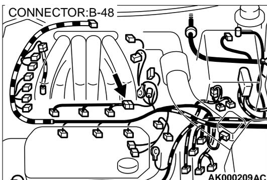
**STEP 7. Check connector B-48 at injector intermediate connector for damage.**
