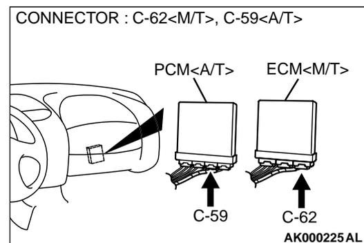
**STEP 4. Check connector B-28 at right bank heated oxygen sensor (rear) and connector C-62 at ECM <M/T> or connector C-59 at PCM <A/T> for damage.**
