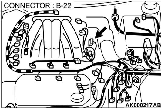
**STEP 2. Check the ignition coil.**
