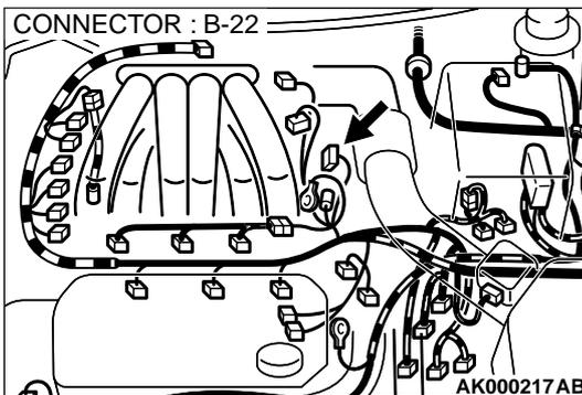
**STEP 16.** Check for harness damage between camshaft position sensor connector B-22 terminal 5 and ECM connector C-58 terminal 50 <M/T> or PCM connector C-55 terminal 56 <A/T>.
