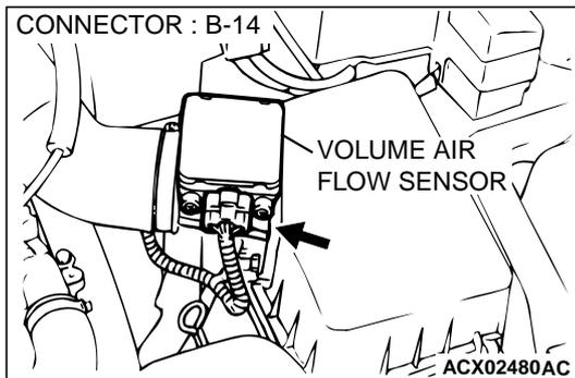
**STEP 6. Check connector B-14 at volume air flow sensor and connector C-51 at ECM <M/T> or connector C-52 at PCM <A/T> for damage.**
