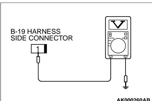
**STEP 6. Check the power supply voltage at power steering pressure switch harness side connector B-19.**
