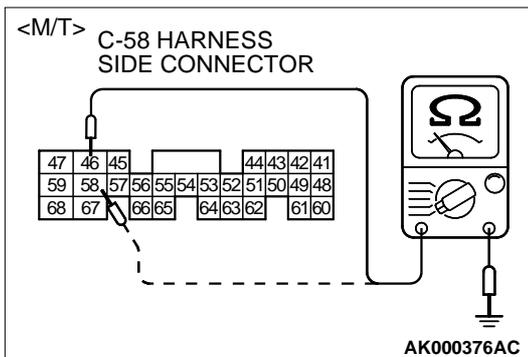
**STEP 7. Check the continuity at ECM harness side connector C-58 <M/T> or PCM harness side connector C-55 <A/T>.**
