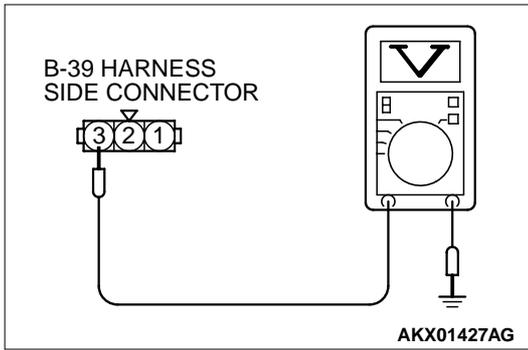
**STEP 11. Check the sensor supply voltage at vehicle speed sensor harness side connector B-39.**
