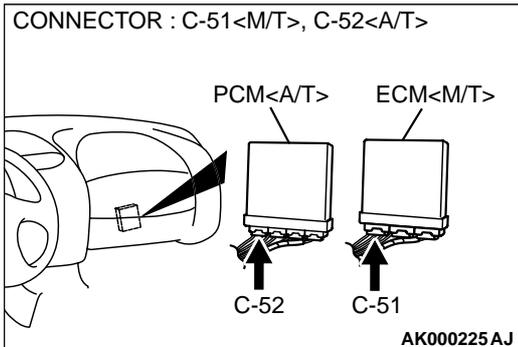
**STEP 7. Check connector C-51 at ECM <M/T> or connector C-52 at PCM <A/T> for damage.**
