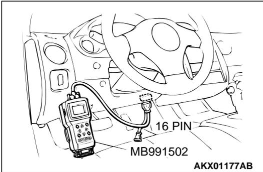
**STEP 2. Using the oscilloscope, check the crankshaft position sensor.**
