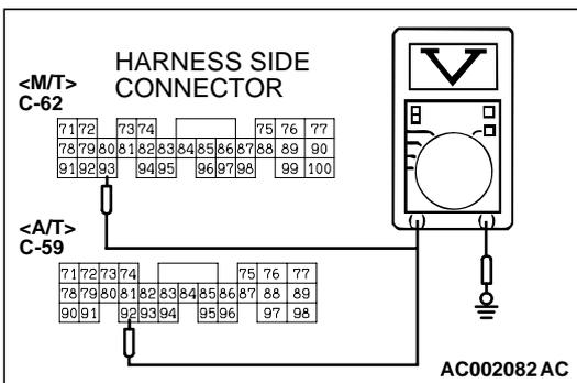
**STEP 10. Check the output circuit voltage at ECM connector C-62 <M/T> or PCM connector C-59 <A/T>.**
