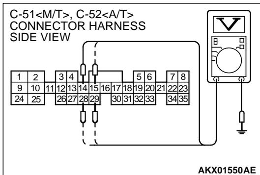
**STEP 7. Check the power supply voltage at ECM connector C-51 <M/T> or PCM connector C-52 <A/T> by backprobing**
