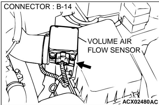
**STEP 8. Check for short circuit to ground between volume air flow sensor connector B-14 terminal 3 and ECM connector C-58 terminal 61 <M/T> or PCM connector C-55 terminal 65 <A/T>.**
