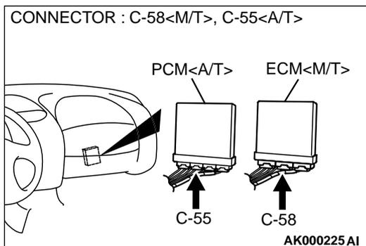
**STEP 11. Check for short circuit to ground between intake air temperature sensor connector B-14 terminal 6 and ECM connector C-58 terminal 62 <M/T> or PCM connector C-55 terminal 64 <A/T>.**
