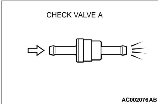
**STEP 28. Check the check valve A.**
