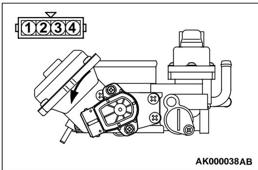
2. Turn the throttle position sensor 90 degrees counterclockwise to set it, and tighten the screws.
