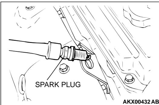
**STEP 4. Check the ignition coil spark**
