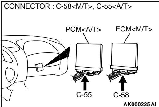
**STEP 13. Check for harness damage between power steering pressure switch connector B-19 terminal 1 and ECM connector C-58 terminal 54 <M/T> or PCM connector C-55 terminal 52 <A/T>.**
