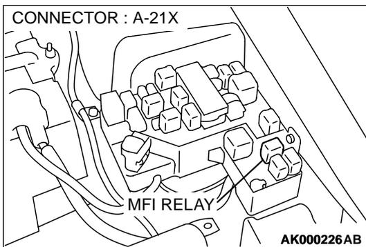
**STEP 8. Check for harness damage between MFI relay connector A-21X terminal 1 and injector intermediate connector B-48 terminal 1.**
