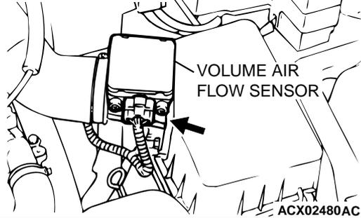
**STEP 11.** Check for open circuit and harness damage between volume air flow sensor connector B-14 terminal 5 and ECM connector C-58 terminal 49 <M/T> or PCM connector C-55 terminal 57 <A/T>.
