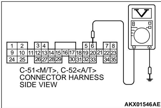
**STEP 6. Check the power supply voltage at ECM connector C-51 <M/T> or PCM connector C-52 <A/T> by backprobing**
