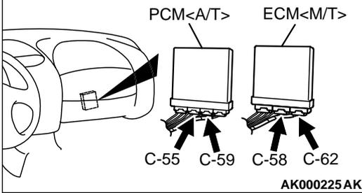
**STEP 9. Check connector C-58, C-62 at ECM <M/T> or connector C-55, C-59 at PCM <A/T> for damage.**
