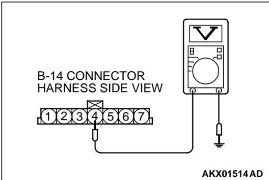
**STEP 2. Check the power supply voltage at volume air flow sensor connector B-14 by backprobing.**
