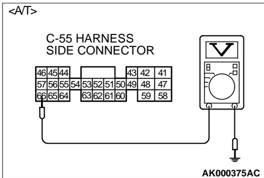
**STEP 6. Check the backup power supply voltage at ECM harness side connector C-58 <M/T> or PCM harness side connector C-55 <A/T>.**
