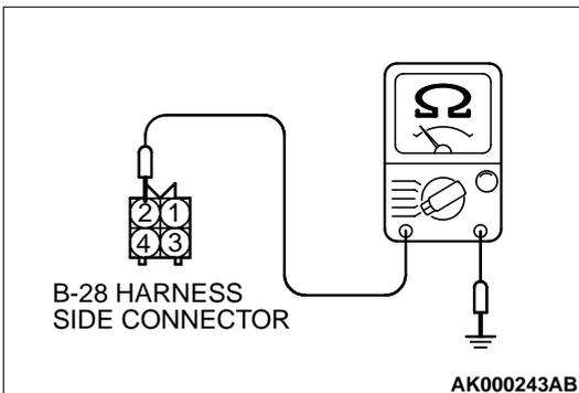
**STEP 8. Check the continuity at right bank heated oxygen sensor (rear) harness side connector B-28.**
