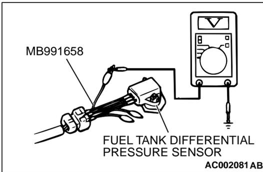
**STEP 7. Check the ground circuit voltage at fuel tank differential pressure sensor connector D-18.**
