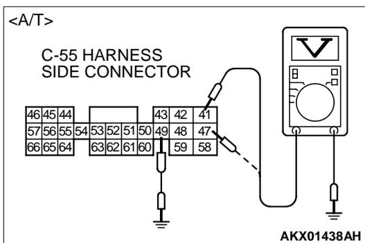
**STEP 9. Check the power supply voltage at ECM harness side connector C-58 <M/T> or PCM harness side connector C-55 <A/T>.**
