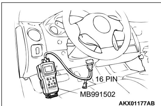
**STEP 4. Using scan tool MB991502, check actuator test.**
