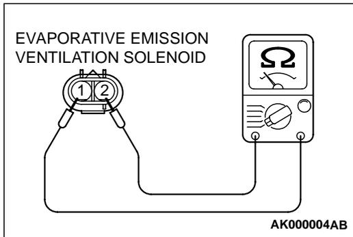
**STEP 3 Check the evaporative emission ventilation solenoid.**
