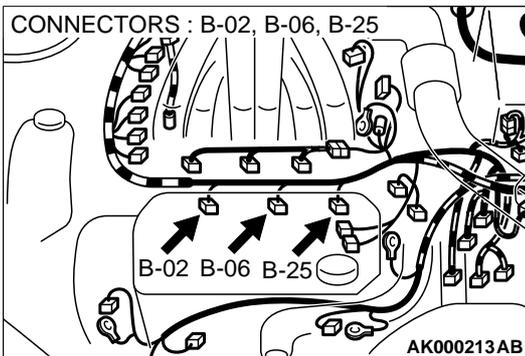
**STEP 7. Check connector B-02, B-06, B-25 at left bank injector for damage.**
