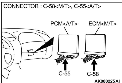
**STEP 4. Check connector C-58 at ECM <M/T> or connector C-55 at PCM <A/T> for damage.**
