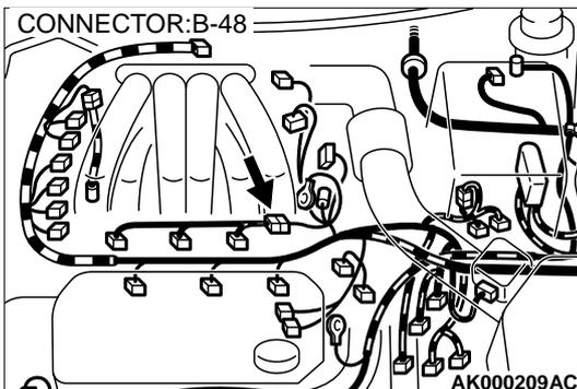
**STEP 12. Check connector B-48 at injector intermediate connector for damage.**
