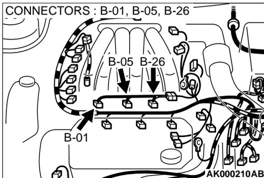
**STEP 11. Check connector B-01 or B-05 or B-26 at right bank injector for damage.**
