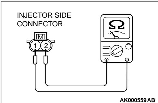
**STEP 9. Check the right bank injector resistance at injector intermediate connector B-48.**
