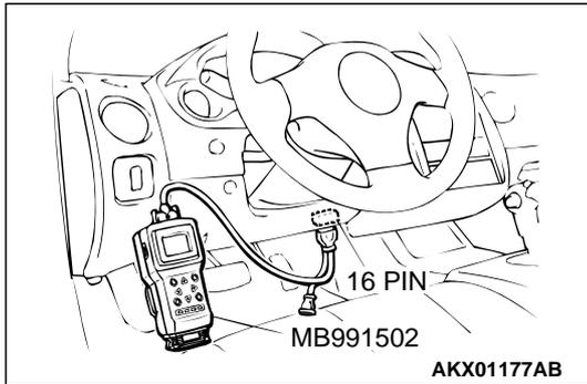
**STEP 6. Using scan tool MB991502, check actuator test items 01, 02, 03, 04, 05, 06: Injector.**
