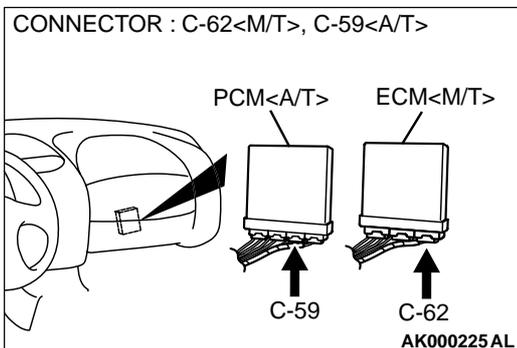
**STEP 3. Check for open circuit, short circuit to ground and harness damage between data link connector C-29 terminal 7 and ECM connector C-62 terminal 85 <M/T> or PCM connector C-59 terminal 85 <A/T>.**
