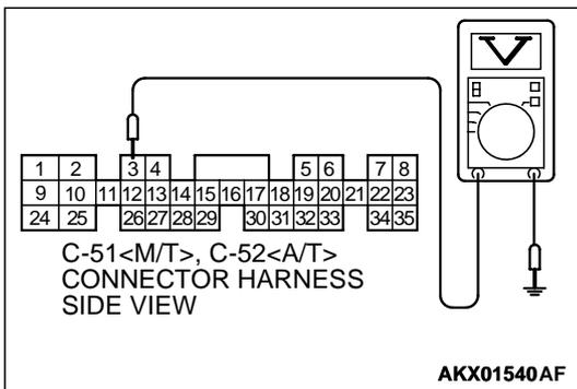
**STEP 6. Check connector C-51 at ECM <M/T> or connector C-52 at PCM <A/T> for damage.**
