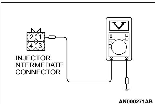
**STEP 6. Check the power supply voltage at injector intermediate connector B-48.**
