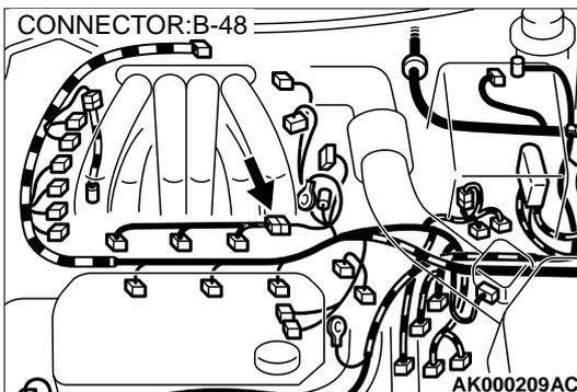
**STEP 10. Check connector B-48 at the injector intermediate connector for damage.**
