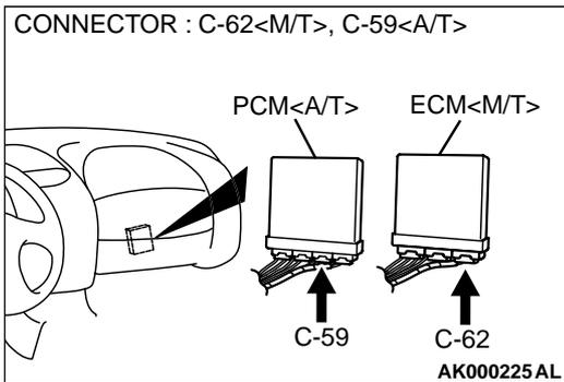
**STEP 2. Check for open circuit, short circuit to ground and harness damage between data link connector C-29 terminal 1 and ECM connector C-62 terminal 84 <M/T> or PCM connector C-59 terminal 84 <A/T>.**
