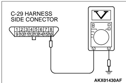
**STEP 2. Check the continuity at data link connector C-29.**
