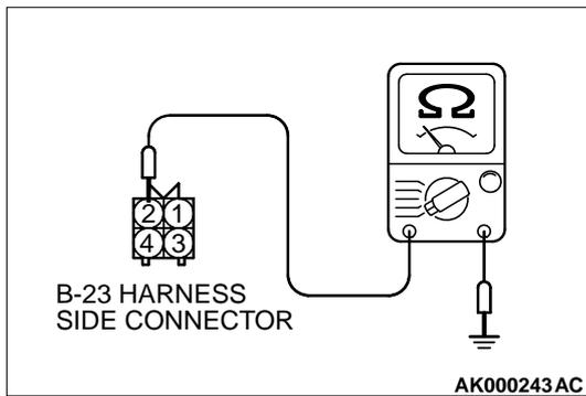
**STEP 8. Check the continuity at left bank heated oxygen sensor (rear) harness side connector B-23.**
