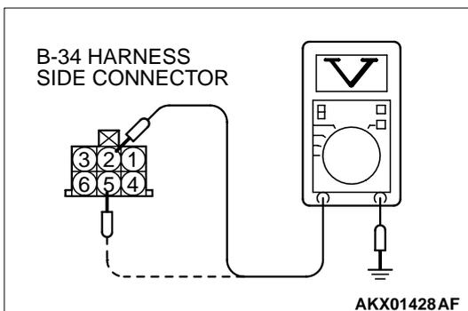
**STEP 5. Check the power supply voltage at idle air control motor harness side connector B-34.**
