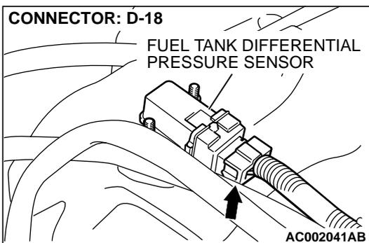
**STEP 8. Check fuel tank differential pressure sensor connector D-18 for damage.**
