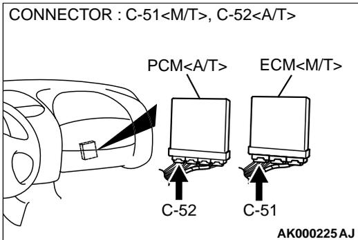
**STEP 10. Check for harness damage between injector connector and ECM connector <M/T> or PCM connector <A/T>.**
