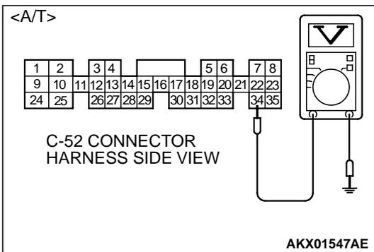
**STEP 6. Check the power supply voltage at ECM connector C-51 <M/T> or PCM connector <A/T> C-52 by backprobing**
