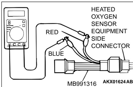
**STEP 3. Check the power supply voltage at left bank heated oxygen sensor (rear) harness side connector B-23.**
