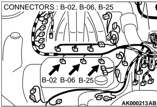
**STEP 8. Check for open circuit and short circuit to ground and harness damage between injector connector and ECM connector <M/T> or PCM connector <A/T>.**
