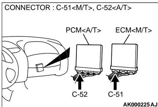
**STEP 2. Check the output voltage at ECM harness side connector C-51 <M/T> or PCM harness side connector C-52 <A/T>.**
