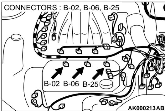
**STEP 13. Check connector B-02, B-06, B-25 at left bank injector for damage.**
