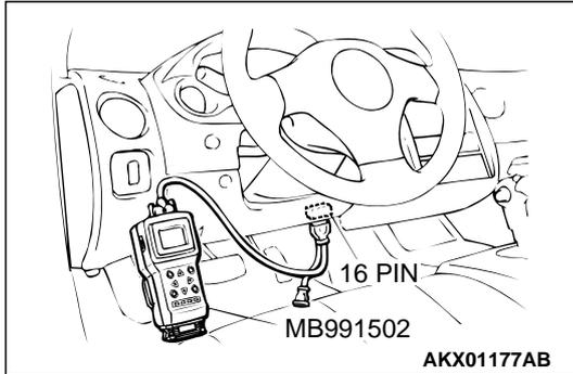
**STEP 14. Using scan tool MB991502, check data list item 59: Left Bank Heated oxygen sensor (rear).**
