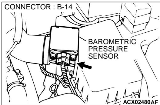
**STEP 8. Check connector B-14 at the barometric pressure sensor and connector C-58 at ECM <M/T> or connector C-55 at PCM <A/T> for damage.**
