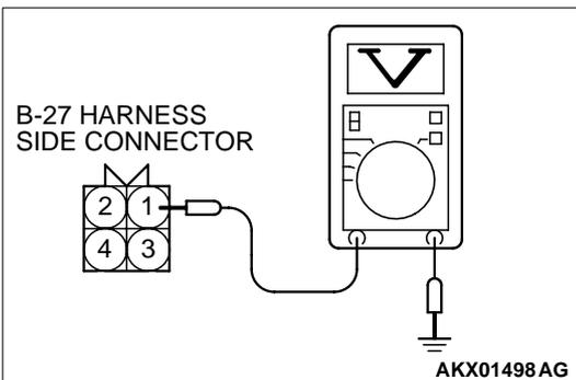
**STEP 3. Check the power supply voltage at right bank heated oxygen sensor (front) harness side connector B-27.**
