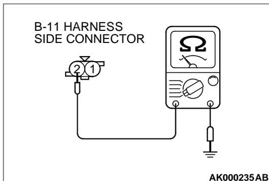
**STEP 8. Check the continuity at engine coolant temperature sensor harness side connector B-11.**
