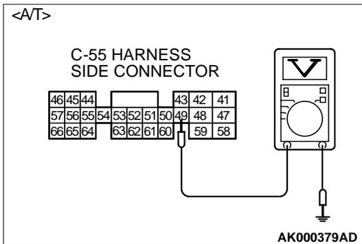
**STEP 8. Check the power supply voltage at ECM harness side connector C-58 <M/T> or PCM harness side connector C-55 <A/T>.**
