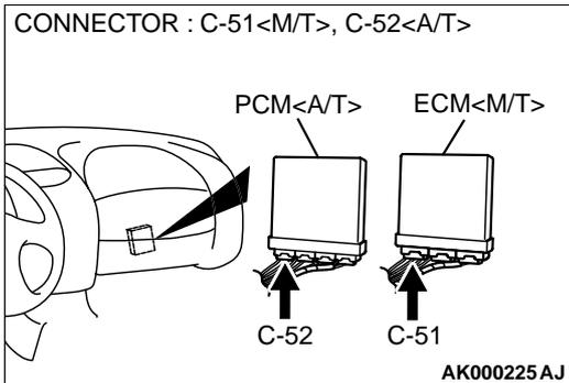
**STEP 12. Check for harness damage between right bank injector connector and ECM connector <M/T> or PCM connector <A/T>.**
