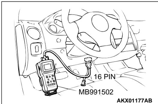
**STEP 14. Using scan tool MB991502, check data list item 27: Power Steering Pressure Switch.**
