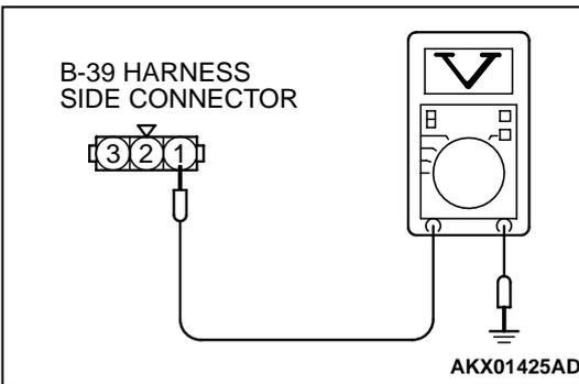
**STEP 9. Check the power supply voltage at vehicle speed sensor harness side connector B-39.**
