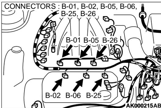
**STEP 6. Check for harness damage between injector connector and ECM connector <M/T> or PCM connector <A/T>.**
