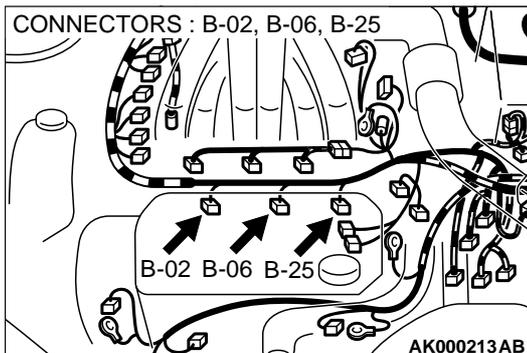
**STEP 11. Check connector B-02, B-06, B-25 at the left bank injector for damage.**
