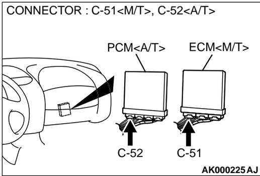
**STEP 5. Check connector C-51 at ECM <M/T> or connector C-52 at PCM <A/T> for damage.**
