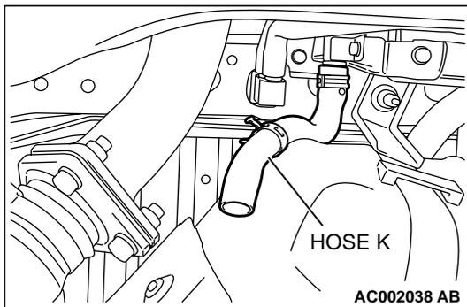
**STEP 11. Check for leaks in the evaporator line from hose J to hose K.**
