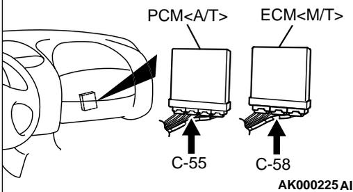
**STEP 9.** Check connector C-58 at ECM <M/T> or connector C-55 at PCM <A/T> for damage.
