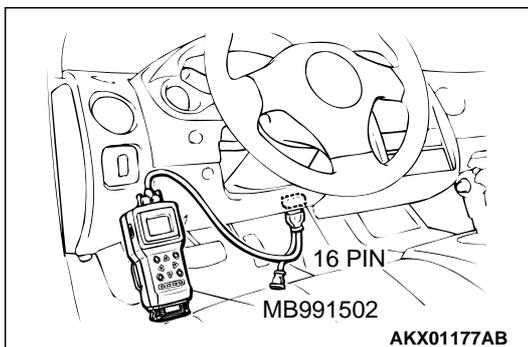
**STEP 5. Using scan tool MB991502, check data list item 21: Engine Coolant Temperature Sensor.**
