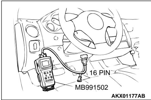
**STEP 2. Using scan tool MB991502, check actuator test items 01, 02, 03, 04, 05, 06: Injector.**
