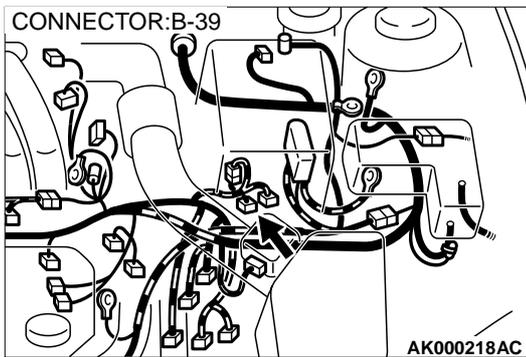
**STEP 16. Check for harness damage between vehicle speed sensor connector B-39 terminal 2 and ground.**
