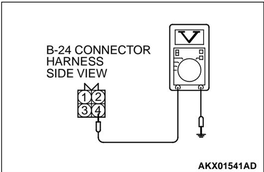
**STEP 2. Check the sensor output voltage at left bank heated oxygen sensor (front) connector B-24 by backprobing.**
