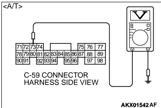
**STEP 3. Check the sensor output voltage at ECM connector C-62 <M/T> or PCM connector C-59 <A/T> by backprobing.**
