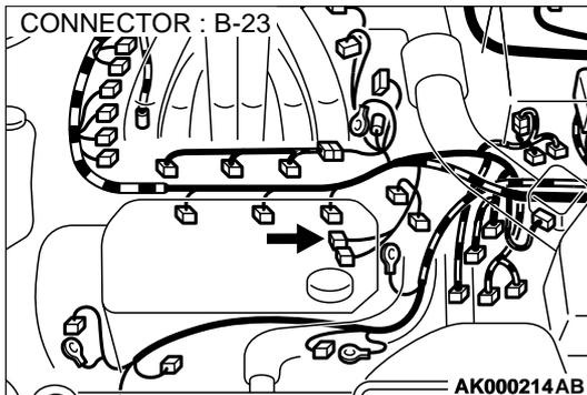
**STEP 10. Check for harness damage between left bank heated oxygen sensor (rear) connector B-23 terminal 3 and ECM connector C-51 terminal 26 <M/T> or PCM connector C-52 terminal 26 <A/T>.**
