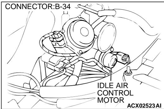
**STEP 13. Check for harness damage between idle air control motor connector B-34 and ECM connector C-51 <M/T> or PCM connector C-52 <A/T>.**
