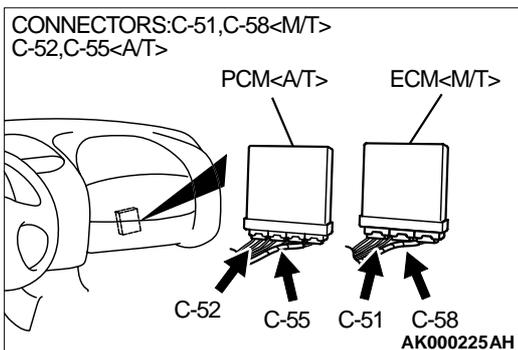
**STEP 6. Check connector C-51, C-58 at ECM <M/T> or connector C-52, C-55 at PCM <A/T> for damage.**
