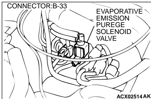
**STEP 11.** Check for harness damage between evaporative emission purge solenoid connector B-33 terminal 1 and ECM connector C-51 terminal 16 <M/T> or PCM connector C-52 terminal 34 <A/T>.
