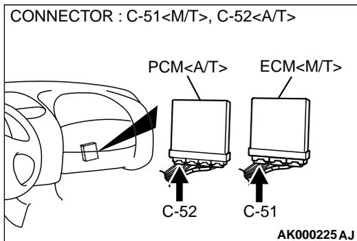
**STEP 7. Check for open circuit or short circuit to ground between left bank heated oxygen sensor (rear) connector B-23 terminal 3 and ECM connector C-51 terminal 26 <M/T> or PCM connector C-52 terminal 26 <A/T>.**
