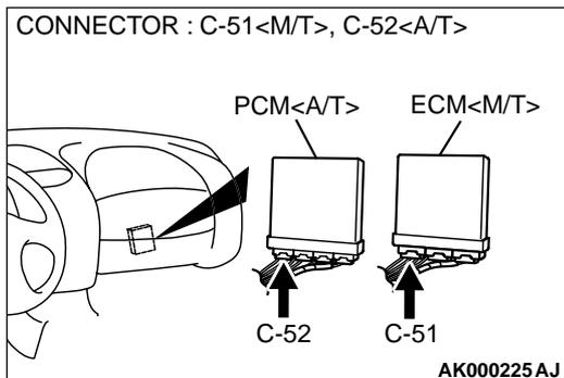
**STEP 9. Check for open circuit and short circuit to ground between idle air control motor connector B-34 and ECM connector C-51 <M/T> or PCM connector C-52 <A/T>.**
