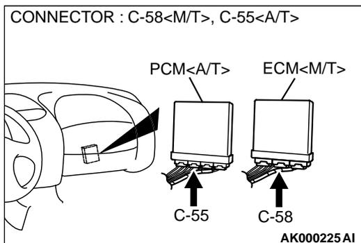
**STEP 14. Check for harness damage between barometric pressure sensor connector B-14 terminal 5 and ECM connector C-58 terminal 49 <M/T> or PCM connector C-55 terminal 57 <A/T>.**
