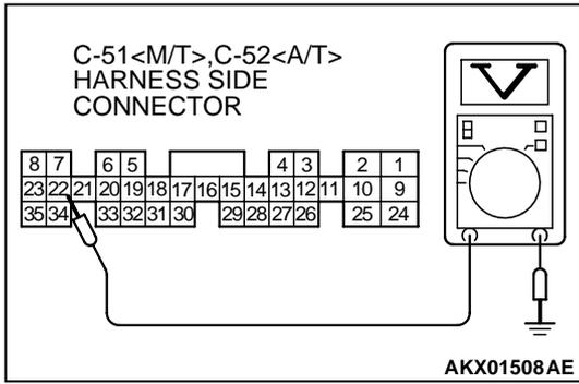
**STEP 6. Check the power supply voltage ECM connector C-51 <M/T> or PCM connector C-52 <A/T>.**
