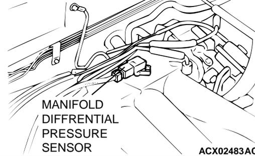
**STEP 8. Check for open circuit and harness damage between manifold differential pressure sensor connector B-04 terminal 2 and ECM connector C-58 terminal 49 <M/T> or PCM connector C-55 terminal 57 <A/T>.**
