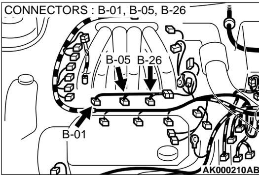
**STEP 10. Check connector B-01 or B-05 or B-26 at right bank injector for damage.**
