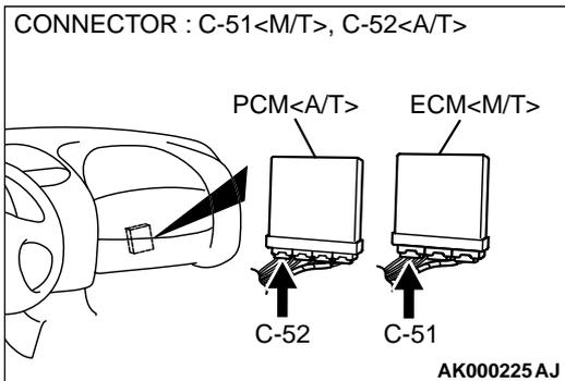
**STEP 15. Check for harness damage between injector connector and PCM connector.**
