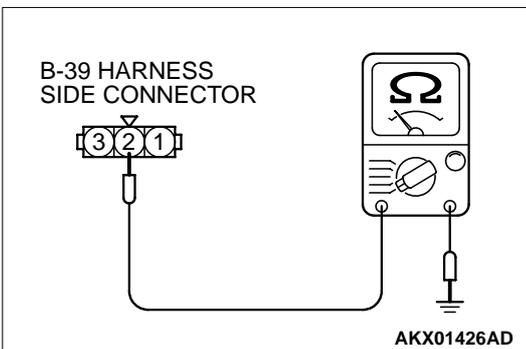
**STEP 10. Check the continuity at vehicle speed sensor harness side connector B-39.**
