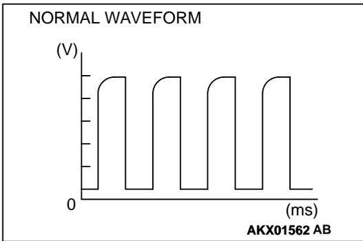
**STEP 3. Using the oscilloscope, check the sensor output voltage at ECM connector C-62.**
