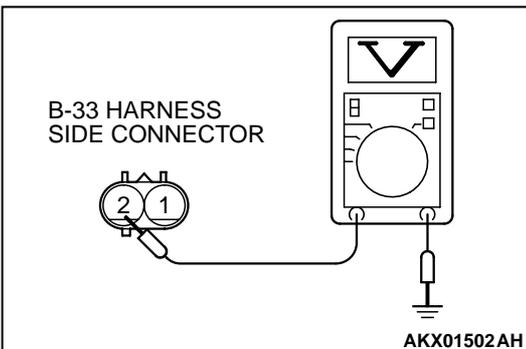
**STEP 4. Check the power supply voltage at evaporative emission purge solenoid harness side connector B-33.**
