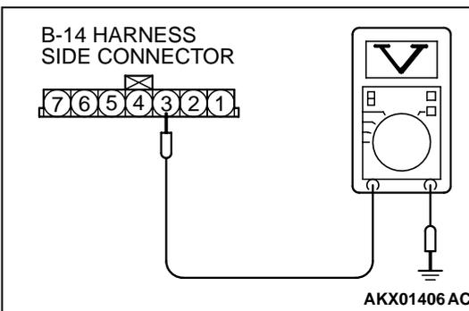
**STEP 6. Check the sensor supply voltage at volume air flow sensor harness side connector B-14.**
