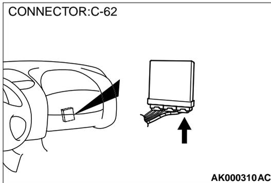
**STEP 4. Check connector C-62 at ECM for damage.**
