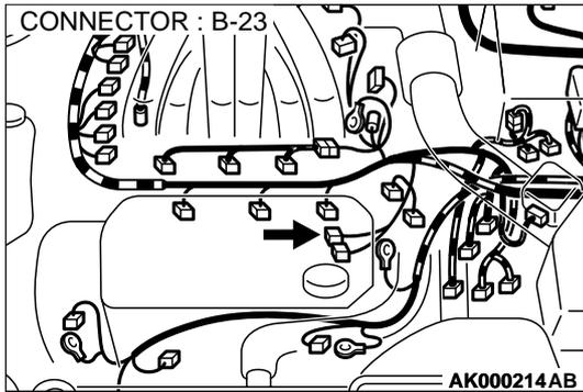
**STEP 7. Check connector B-23 at left bank heated oxygen sensor (rear) for damage.**
