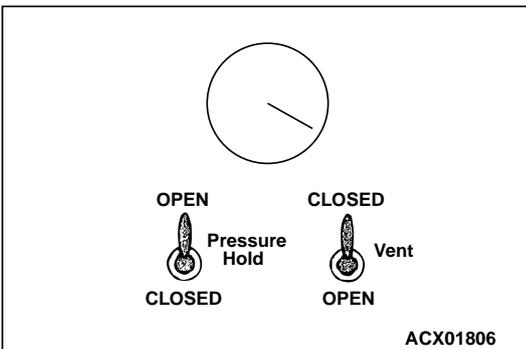
(2) On the EVAP pressure pump, set the pressure/hold valve to OPEN, and set the vent valve to CLOSED. Turn the pump timer to ON. You can reset the timer as required. (These settings are listed under "Leak Test" in the pump instructions.)
