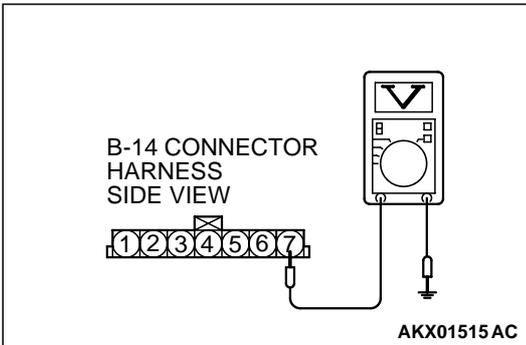
**STEP 2. Check the reset signal voltage at volume air flow sensor connector B-14 by backprobing**
