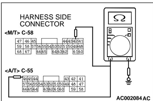
**STEP 13. Check the sensor power supply line for short circuit to ground at ECM connector C-58 <M/T> or PCM connector C-55 <A/T>.**
