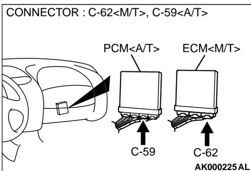
**STEP 12. Check for harness damage between right bank heated oxygen sensor (rear) connector B-28 terminal 2 and ECM connector C-58 terminal 49 <M/T> or PCM connector C-55 terminal 57 <A/T>.**
