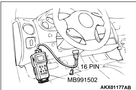
**STEP 5. Using scan tool MB991502, check data list item 25: Barometric Pressure Sensor.**
