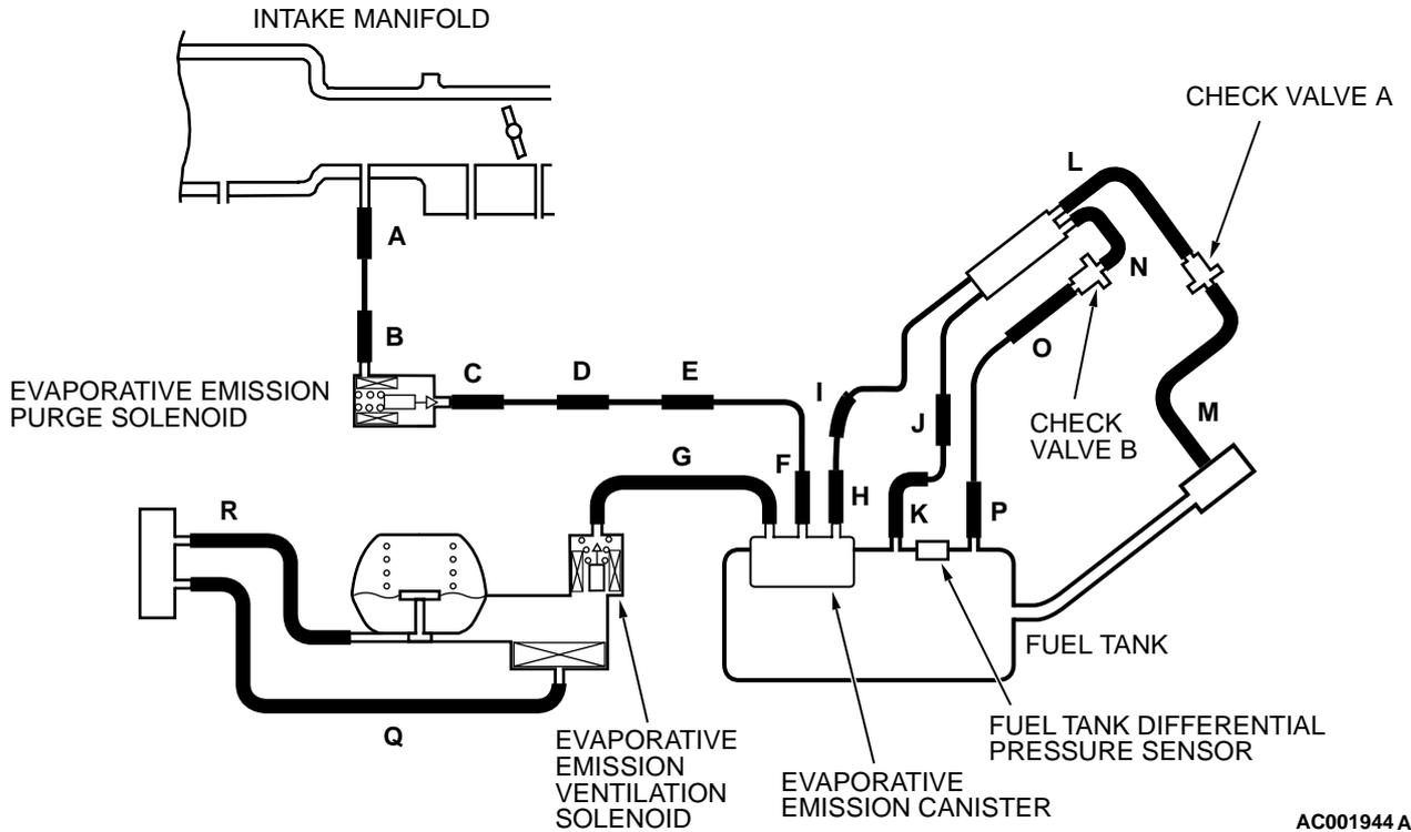
Fuel Tank Differential Pressure Sensor Circuit
