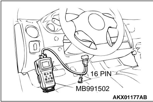
**STEP 2. Using scan tool MB991502, check data list item 13: Intake Air Temperature Sensor.**
