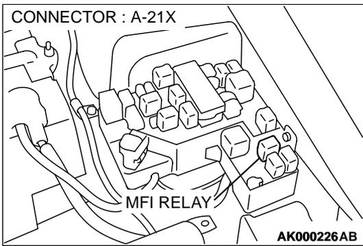
**STEP 13. Check connector A-21X at the MFI relay for damage.**
