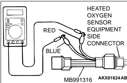
**STEP 3. Check the power supply voltage at right bank heated oxygen sensor (rear) harness side connector B-28.**
