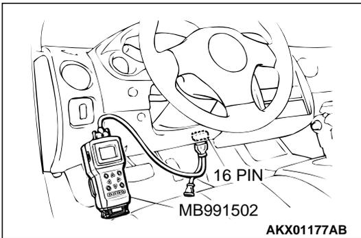
**STEP 3. Using scan tool MB991502, check data list item 21: Engine Coolant Temperature Sensor.**
