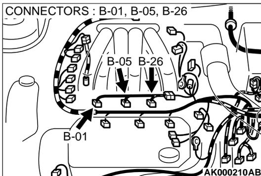
**STEP 7. Check connector B-01, B-05, B-26 at right bank injector for damage.**
