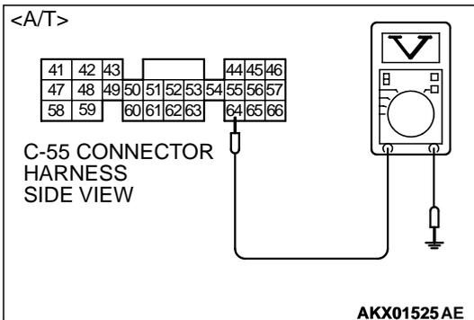
**STEP 8. Check the sensor supply voltage at ECM connector C-58 <M/T> or PCM connector C-55 <A/T> by backprobing.**
