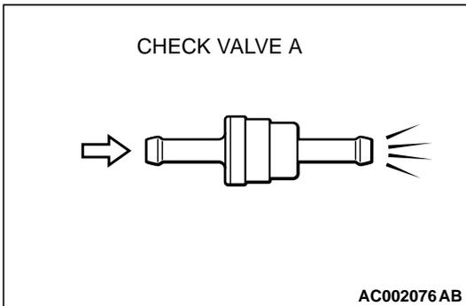
**STEP 13. Check the check valve A.**
