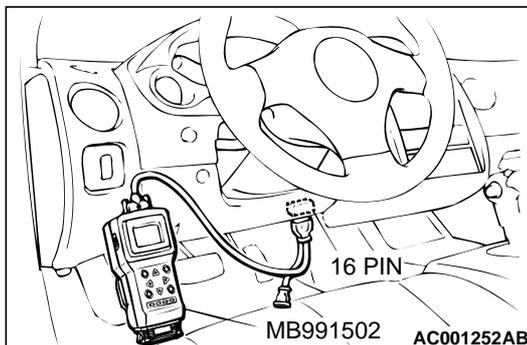
DTC P0500: Vehicle Speed Sensor Malfunction <M/T>
