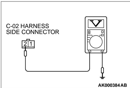
**STEP 8. Check the power supply voltage at interlock switch connector C-02.**
