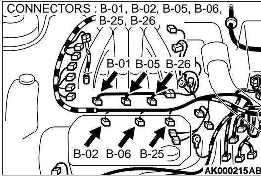
**STEP 12. Replace the injector.**
