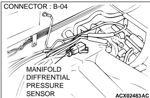
**STEP 3. Check the sensor supply voltage at manifold differential pressure sensor harness side connector B-04.**
