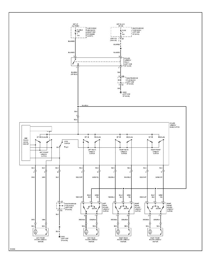
SYSTEM WIRING DIAGRAMS 2.0L, Power Window Circuit, W/ ETACS Unit (p. 13) 1991 Mitsubishi Galant
