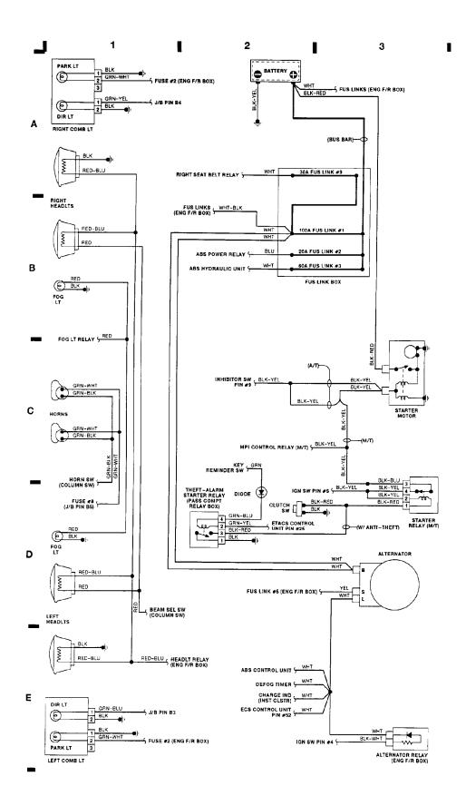
WIRING DIAGRAMS Fig. 2: Computer Engine Control (2.0L SOHC) (Grid 4-7) (p. 2) 1991 Mitsubishi Galant
