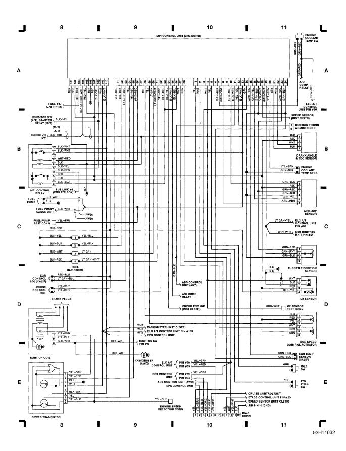
WIRING DIAGRAMS Fig. 4: Computer Engine Control (2.0L TURBO) (Grid 12-15) (p. 4) 1991 Mitsubishi Galant
