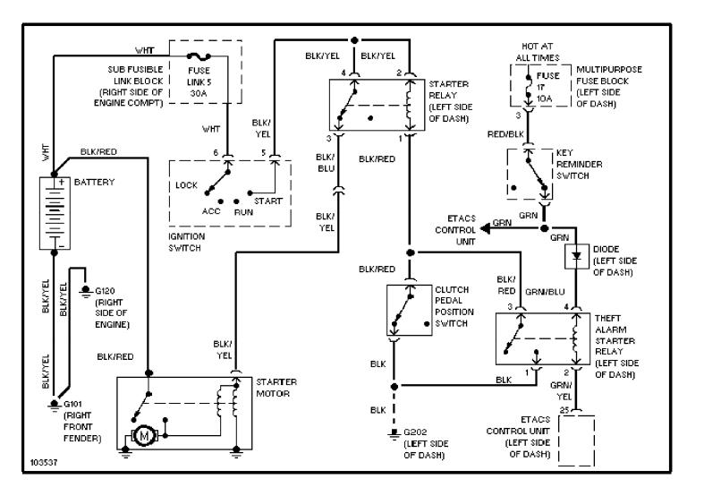
SYSTEM WIRING DIAGRAMS Starting Circuit, W/O Theft Deterrent (p. 19) 1991 Mitsubishi Galant
