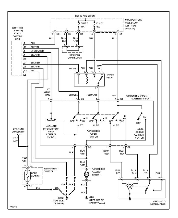
SYSTEM WIRING DIAGRAMS Wiper/Washer Circuit, W/O ETACS UNIT (p. 21)
