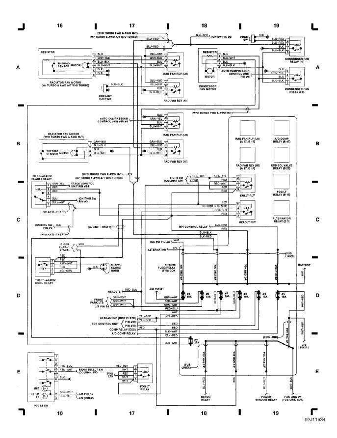
WIRING DIAGRAMS Fig. 6: Junction Block (Partial), Ignition Switch (Grid 20-23) (p. 6) 1991 Mitsubishi Galant
