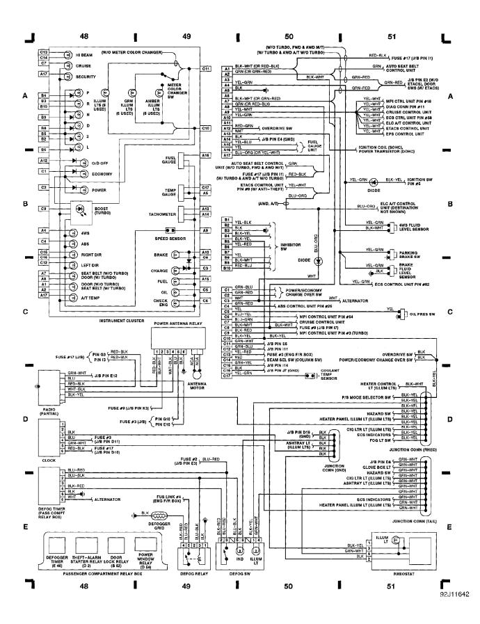
WIRING DIAGRAMS Fig. 14: Power Door/Window/Mir, Taillights (Grid 52-55) (p. 14) 1991 Mitsubishi Galant
