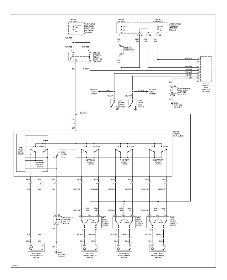
SYSTEM WIRING DIAGRAMS 2.0L, Power Window Circuit, W/O ETACS Unit (p. 14) 1991 Mitsubishi Galant
