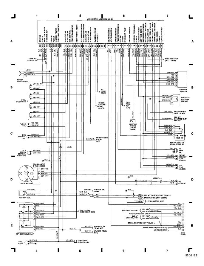
WIRING DIAGRAMS Fig. 3: Computer Engine Control (2.0L DOHC) (Grid 8-11) (p. 3) 1991 Mitsubishi Galant
