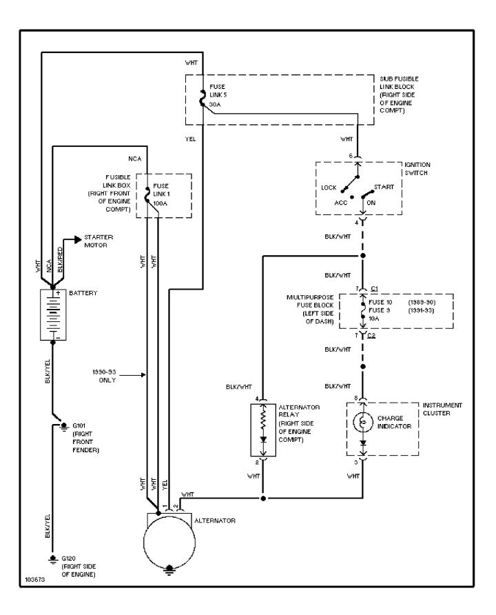
SYSTEM WIRING DIAGRAMS Starting Circuit, W/ Theft Deterrent (p. 18) 1991 Mitsubishi Galant
