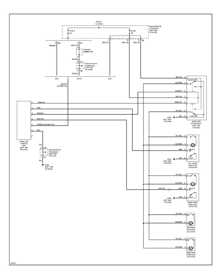
SYSTEM WIRING DIAGRAMS 2.0L, Power Door Lock Circuit, W/ ETACS Unit (p. 8) 1991 Mitsubishi Galant
