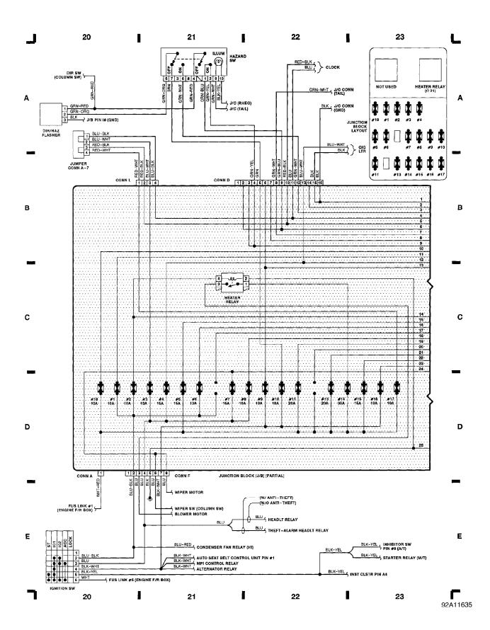
WIRING DIAGRAMS Fig. 7: Junction Block (Partial) (Grid 24-27) (p. 7)
