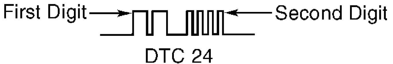
Fig. 9: Identifying Voltmeter Trouble Code Display Courtesy of Mitsubishi Motor Sales of America.
