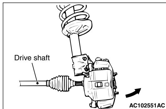
2. Remove the drive shaft from the hub by pulling the bottom of the brake disc towards you.
