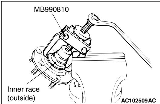
2. Remove the wheel bearing inner race (outside) from the front hub by using special tool side bearing puller (MB990810).
