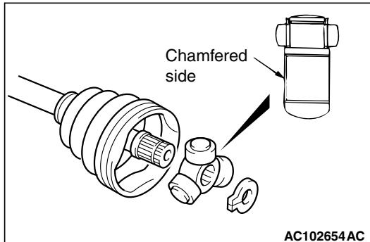
2. Install the spider assembly to the shaft from the direction of the spline chamfered side.
