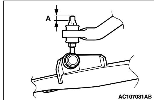
Tighten the self-locking nut so that the protruding length of the stabilizer link protruding part meets its standard value (A).
