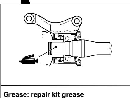
Grease: repair kit grease
