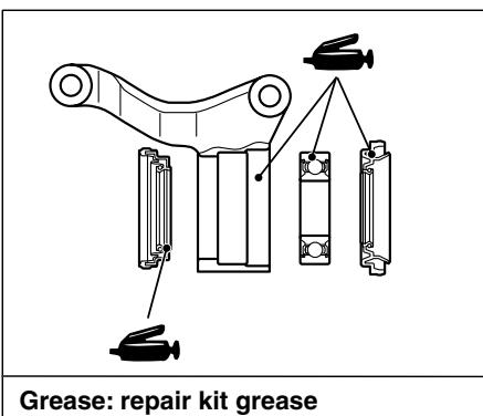
Grease: repair kit grease
