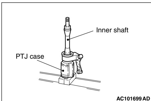
2. Apply repair kit grease to the inner shaft spline, then press fit it into the PTJ case.
