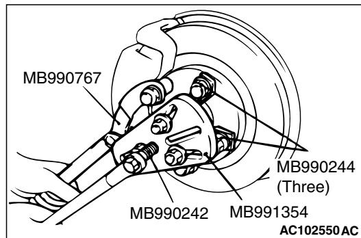
1. Use the following special tools to push out the drive shaft from the hub and knuckle.
