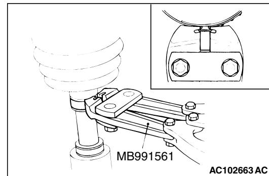
7. Use the special tool to crimp the boot band (small).
