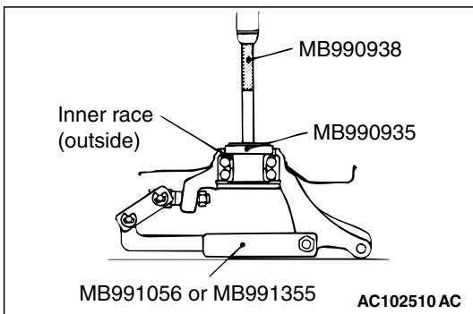
3. Install the inner race (outside) that was removed from the hub to the wheel bearing, and then use the following special tools to remove the wheel bearing.
