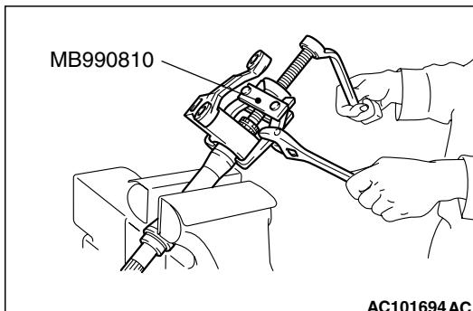
2. Use special tool side bearing puller (MB990810) to remove the centre bearing bracket from the inner shaft.
