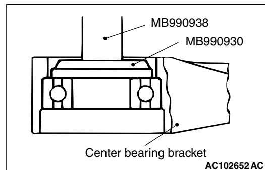
Use the following special tools to remove the centre bearing from the centre bearing bracket.
