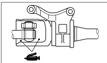
Grease: repair kit grease
