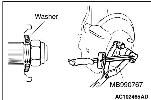
1. Be sure to install the drive shaft washer in the specified direction.
