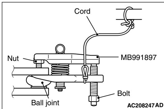
1. Install special tool ball joint remover (MB991897) as shown in the figure.
