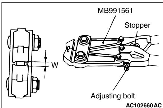
5. Turn the adjusting bolt on special tool boot band crimping tool (MB991561) so that the size of the opening (W) is at the standard value.
