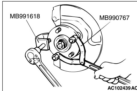
3. Use the following special tools to remove the hub bolts.
