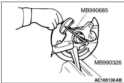
3. Measure the hub starting torque by using the following special tools.
