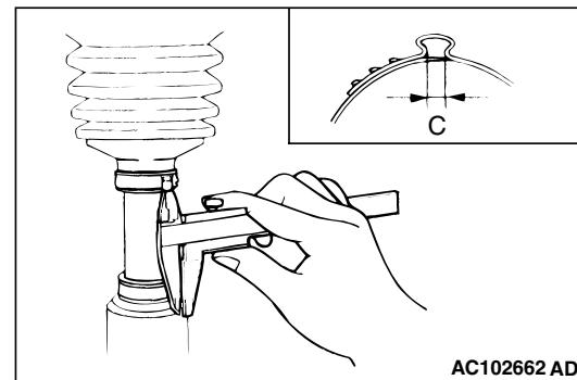
8. Check that the crimping amount (C) of the boot band is at the standard value.
