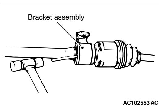
4. If the inner shaft is hard to remove from the transmission, strike the bracket assembly lightly with a plastic hammer and remove the inner shaft.
