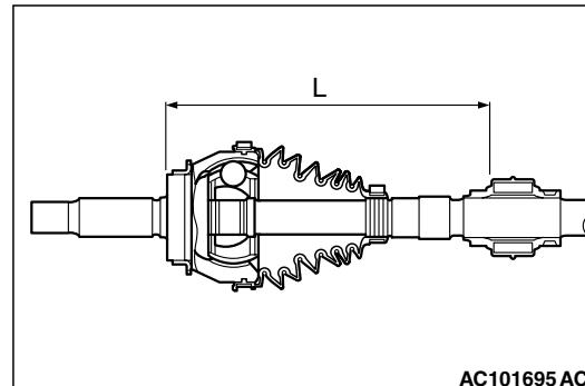
1. Install the dynamic damper in the position (L) shown in the figure .
