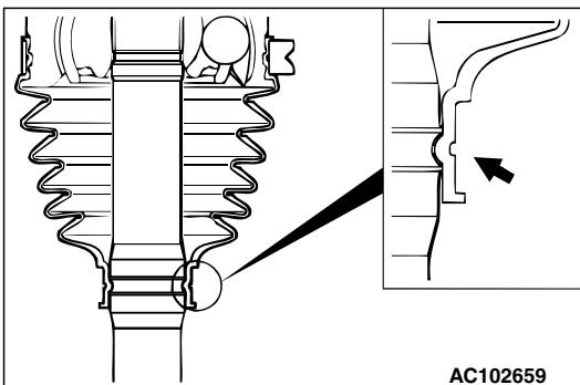
4. Align the centre groove on the BJ boot small end with the shaft groove.
