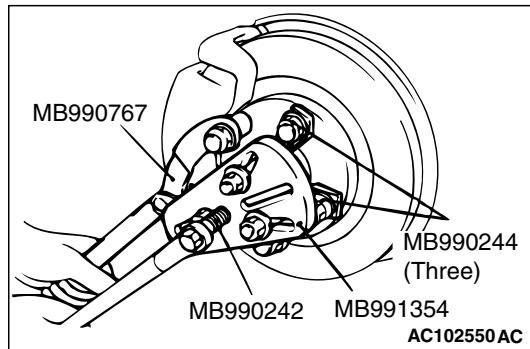
1. Use the following special tools to push out the drive shaft or the drive shaft and inner shaft assembly from the hub.
