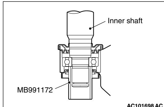
1. Use special tool inner shaft installer base (MB991172) to hold the centre bearing inner race, and then press-in the inner shaft.
