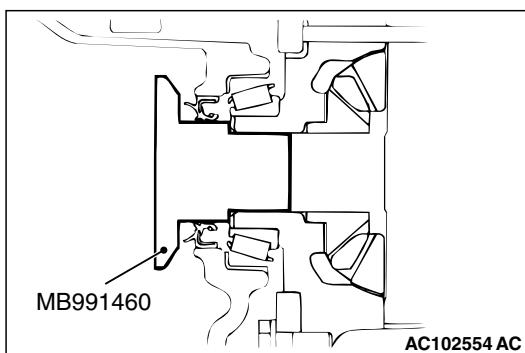
5. Use special tool plug (MB991460) to prevent the entry of foreign material into the transmission case.
