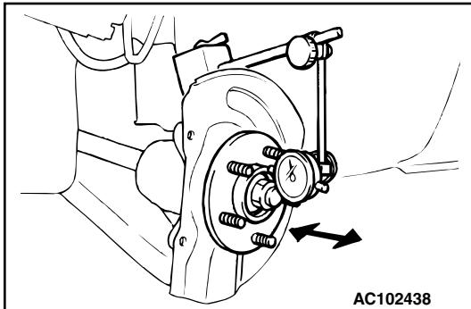
3. Attach a dial gauge as shown in the illustration, and then measure the axial play while moving the hub in the axial direction.
