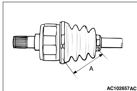
Set the PTJ boot bands at the specified distance in order to adjust the amount of air inside the PTJ boot, and then tighten the PTJ boot band (small), PTJ boot band (large) securely.
