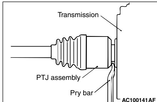
3. Insert a pry bar between the transmission case and the drive shaft, and then pry and remove the drive shaft from the transmission.
