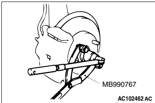
Use special tool end yoke holder (MB990767) to fix the hub and remove the drive shaft nut.
