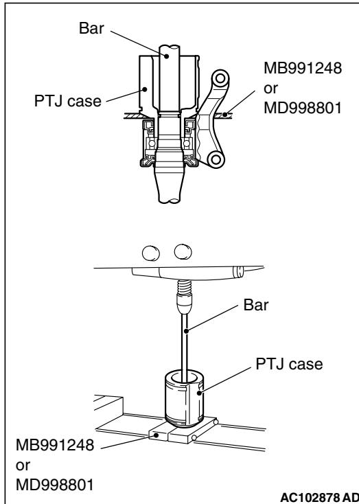
1. Use special tool inner shaft remover (MB991248 or MD998801) to remove the inner shaft assembly from the PTJ case.
