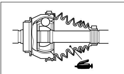
Grease: repair kit grease
