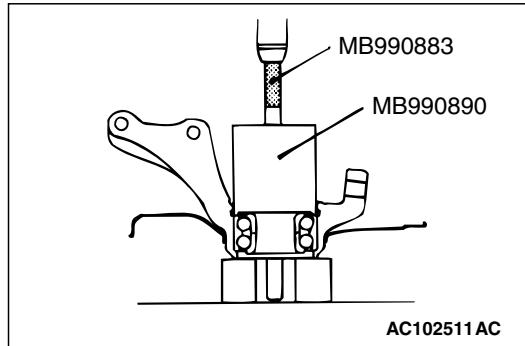
3. Press-in the bearing by using the following special tools.
