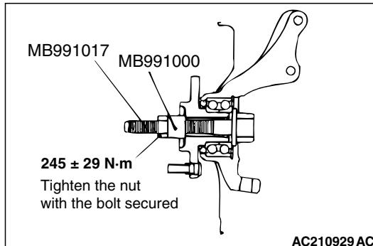
1. Tighten the following special tools to the specified torque, and then press-in the hub into the knuckle.
