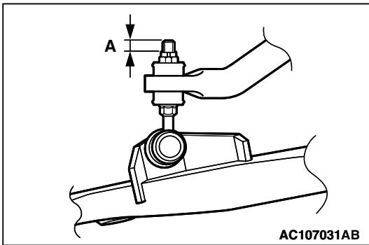
Tighten the self-locking nut so that the protruding length of the stabilizer link protruding part meets its standard value (A).
