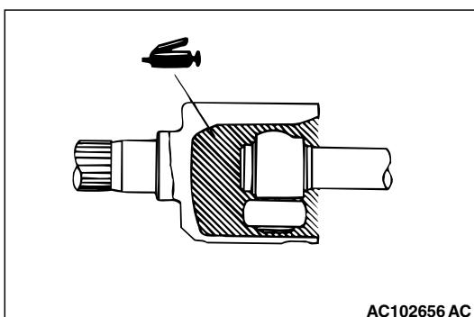
After applying the specified grease to the PTJ case, insert the drive shaft and apply grease one more time.
