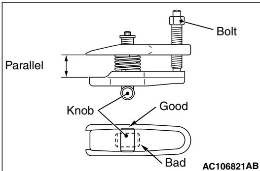
2. Turn the bolt and knob as necessary to make the jaws of special tool parallel, tighten the bolt by hand and confirm that the jaws are still parallel.
