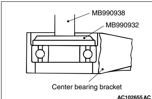
Use the following special tools to press-fit the centre bearing into the centre bearing bracket.
