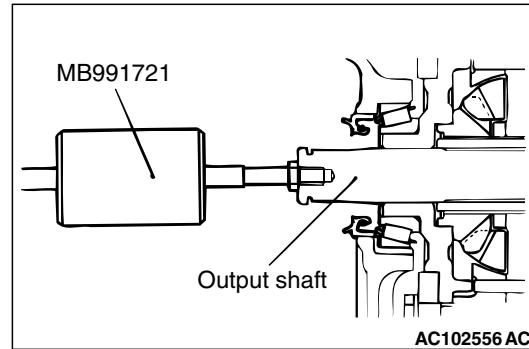
Use special tool sliding hammer (MB991721) to remove the output shaft.
