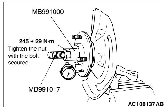
1. Measure to determine whether the wheel bearing axial play is within the limit or not by using the following special tools.
