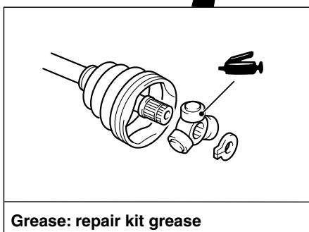
Grease: repair kit grease
