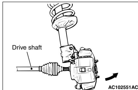
2. Withdraw the drive shaft from the hub by pulling the bottom of the hub and knuckle towards you.
