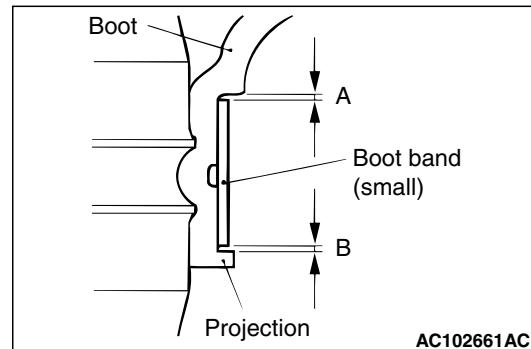
6. Position the BJ boot band (small) so that there is even clearance at either end (A and B).
