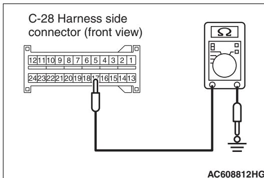
(2) Take the measurements below at the C-28 wiring harness side connectors.
