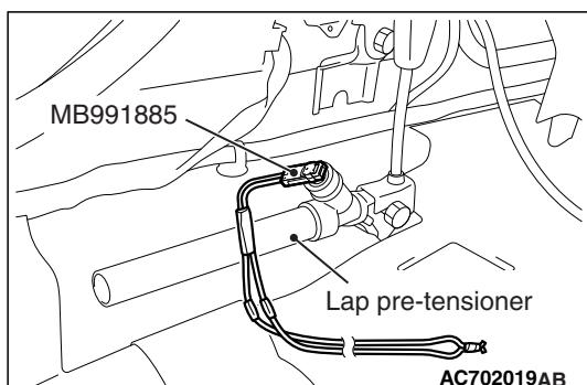
5. Connect deployment wires, each 6 meters (20 feet) or longer, to the two leads of special tool MB991885, and cover the connections with insulation tape. The other ends of the deployment wires should be connected to each other (short-circuited), to prevent sudden unexpected operation of the lap pre-tensioner.
