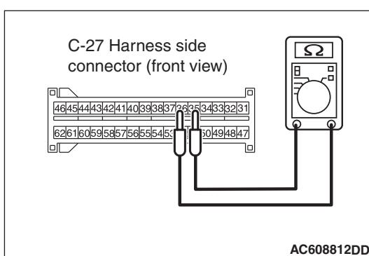
**STEP 5. Check the lap pre-tensioner circuit. Measure the resistance at the SRS-ECU connector C-27.**
