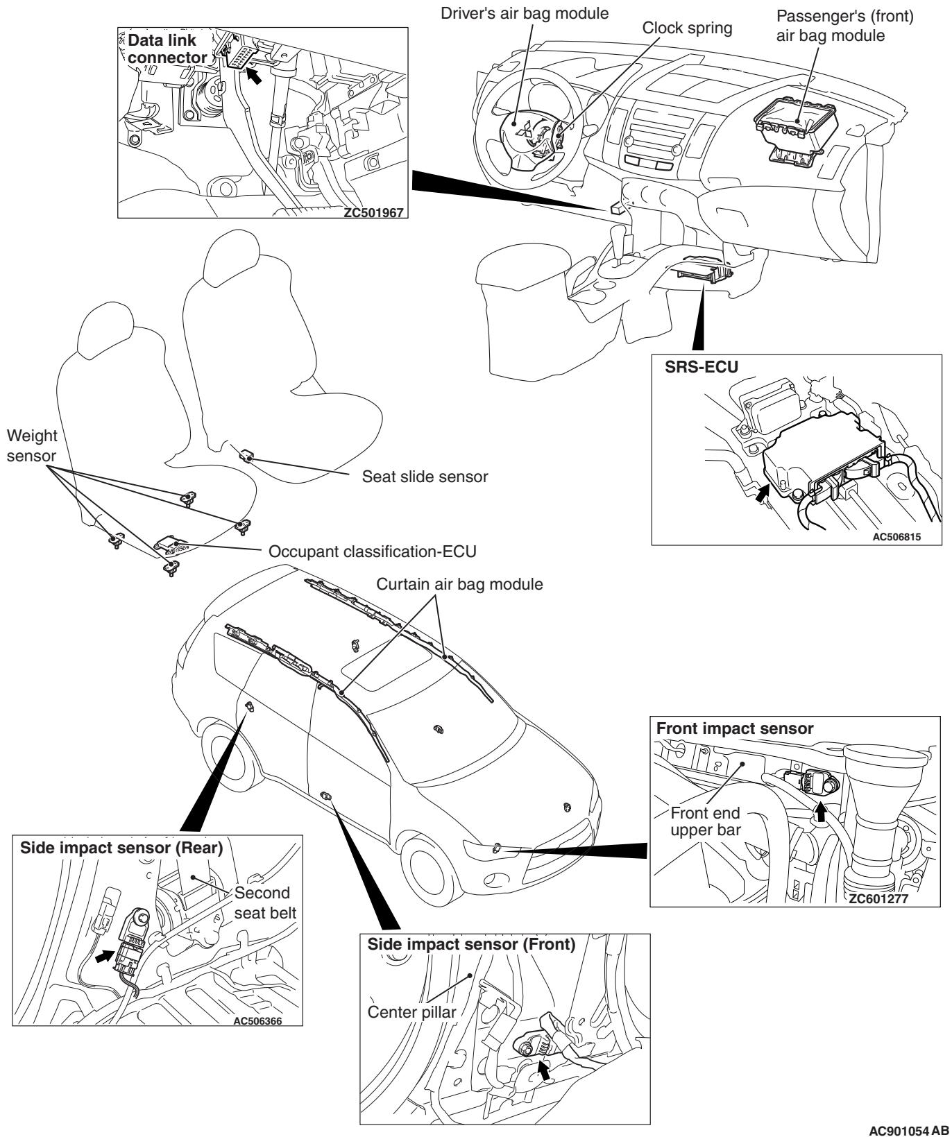
*NOTE: The illustration above shows the front impact sensor (RH) and the side impact sensor (RH). The position of the front impact sensor (LH) and the side impact sensor (LH) is symmetrical to this.*
