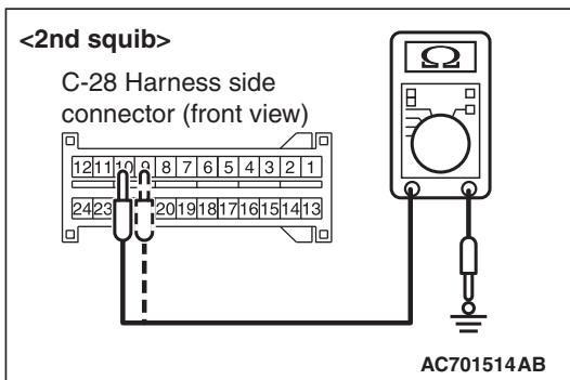
(4) Check for continuity between C-28 harness side connector terminals 5 and 6 <1st squib> or 9 and 10 <2nd squib> and body ground.
