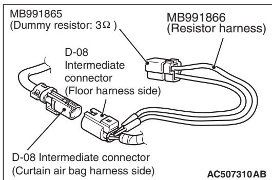
**STEP 4. Check by dummy resistor connection. (Using scan tool MB991958, read the diagnostic trouble code.)**
