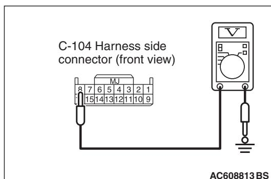
**STEP 5. Measure the voltage at the center panel assembly connector.**
