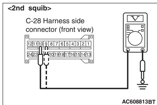
**STEP 6. Check the harness for short circuit to power supply between the following connector.**
