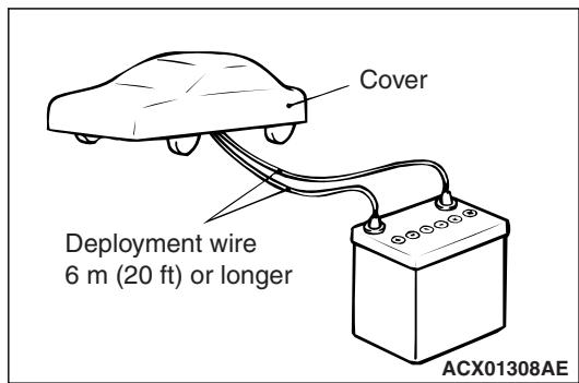
6. Connect the special tool MB992102 to the driver's air bag module, and then pull out the deployment wire to outside the vehicle.
