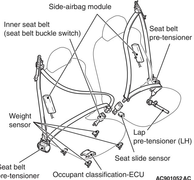
*NOTE: This construction diagram shows the general view of the SRS components. For details, refer to*
