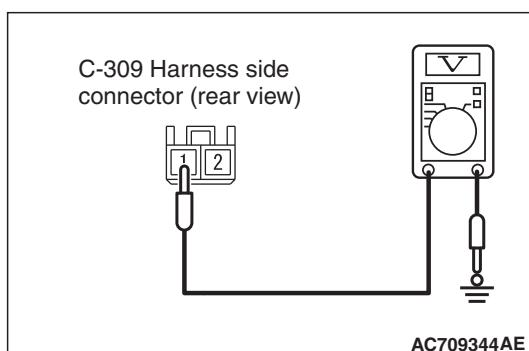
**STEP 4. Measure the voltage at the ETACS-ECU connector.**
