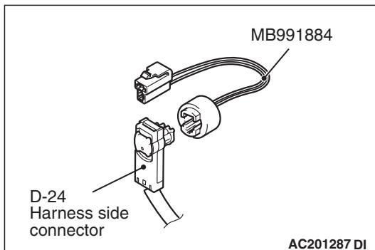
(5) Connect D-24 harness side connector to special tool MB991884.
