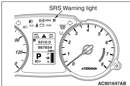
1. Check that the SRS warning light illuminates when the ignition switch is in the "ON" position.
