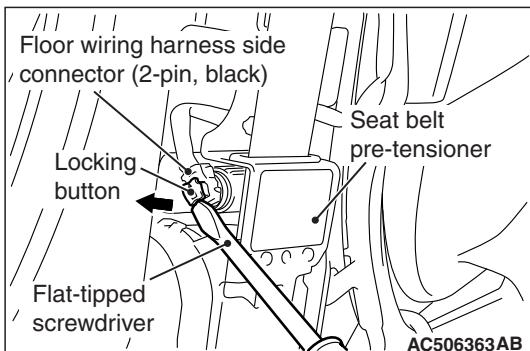
**STEP 3. Check SRS-ECU connector C-27 and passenger's seat belt pre-tensioner connector D-130. (Using scan tool MB991958, read the diagnostic trouble code.)**
