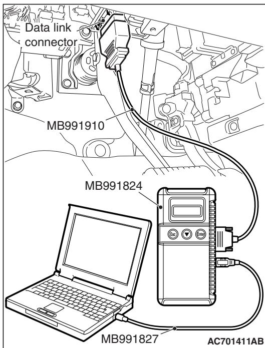
**STEP 3. Check the driver's air bag module. (Using scan tool MB991958, read the diagnostic trouble code.)**
