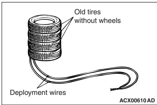
7. Place three old tires without wheels on the tire secured with the driver's air bag module.
