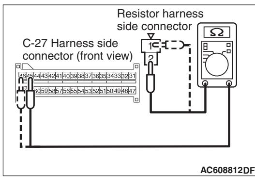
(6) Check for continuity between the following terminals. It should be less than 2 ohms.
