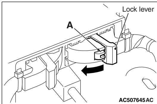
**STEP 3. Check SRS-ECU connector C-27 and lap pre-tensioner connector D-24. (Using scan tool MB991958, read the diagnostic trouble code.)**
