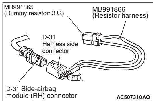
**STEP 4. Check the side-air bag module (RH). (Using scan tool MB991934, read the diagnostic trouble code.)**
