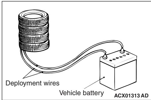
8. At a location as far away from the air bag module as possible, and from a shielded position, disconnect the two connected wires from each other, and connect them, to the two terminals of the battery (which has been removed from the vehicle) to deploy the air bag.
