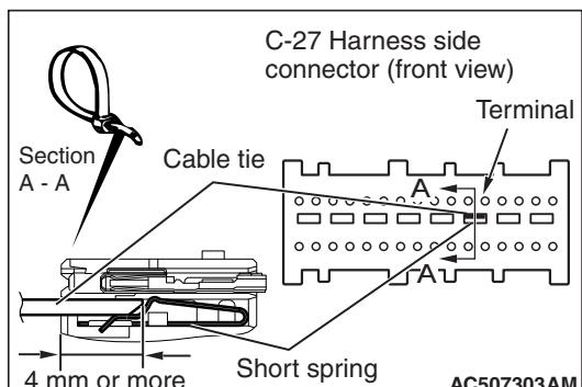
**STEP 4. Check the harness for open circuit between SRS-ECU connector C-27 (terminal No.35 and 36) and the lap pre-tensioner D-24 (terminal No.2 and 1).**
