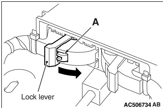
**STEP 5. Check the passenger's (front) air bag module circuit at SRS-ECU connector C-28.**
