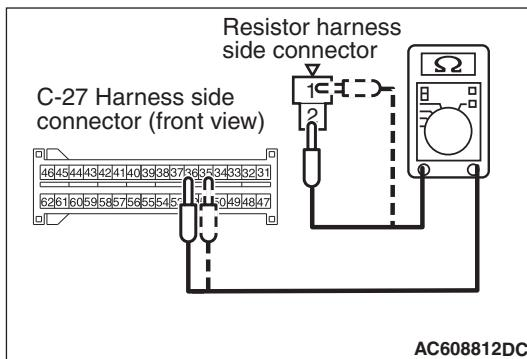
(6) Check for continuity between the following terminals. It should be less than 2 ohms.
