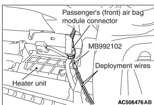
5. Connect deployment wires, each 6 meters (20 feet) or longer, to the two leads of SRS air bag adapter harness (MB9921020), and cover the connections with insulator tape. The other ends of the deployment wires should be connected to each other (short-circuited), to prevent sudden unexpected deployment of the air bag module.
