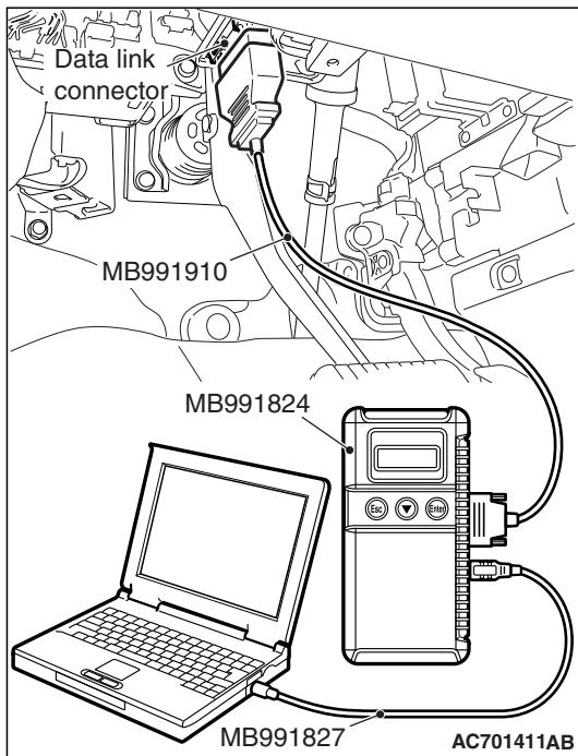
**STEP 4. Using scan tool MB991958, diagnose the ETACS.**
