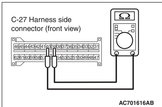
(5) Check for continuity between the C-27 wiring harness side connector terminal No. 39 and No. 40.
