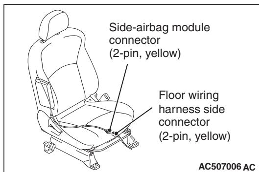
3. Disconnect the connections of the side-air bag module connector (two-pin: yellow) and the floor harness side connector (two-pin: yellow).
