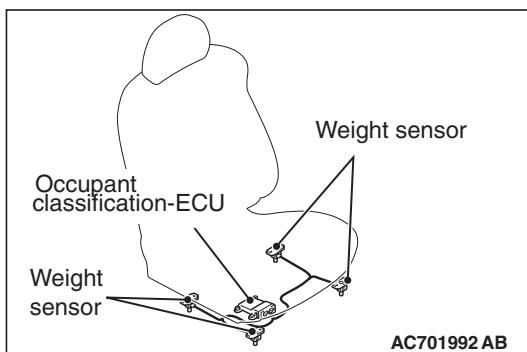
1. Check the occupant classification-ECU case and weight sensor for dents, cracks or deformation.
