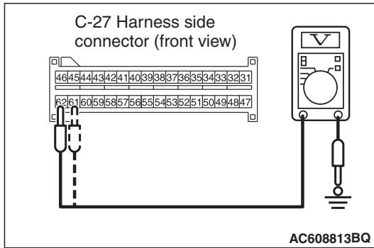
(5) Take the measurements below at the C-27 harness side connector.
