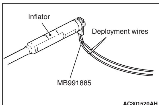
6. Connect the special tool MB991885 to the inflator, and then pull out the deployment wire to outside the vehicle.
