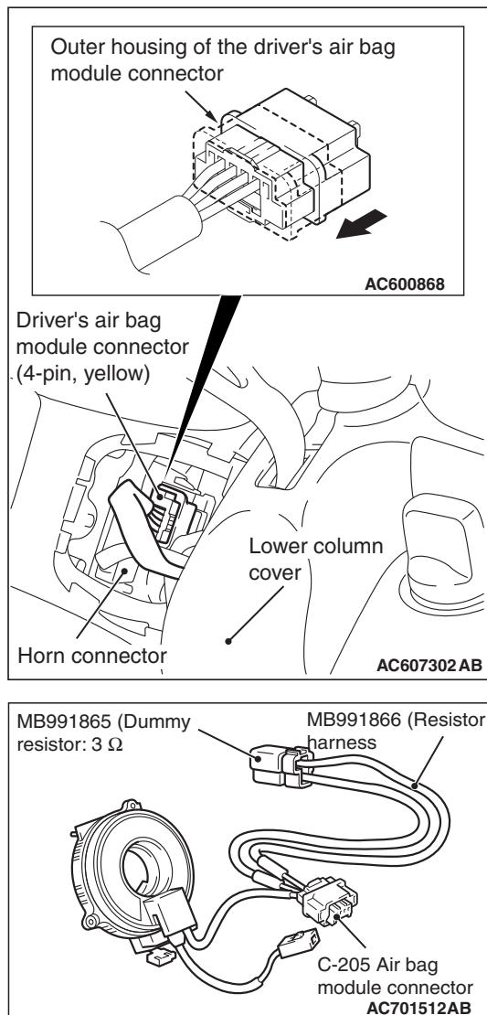
**STEP 3. Check the driver's air bag module. (Using scan tool MB991958, read the diagnostic trouble code.)**
