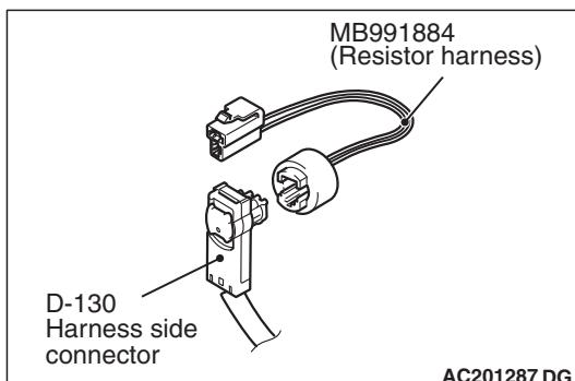
(5) Connect D-130 harness side connector to special tool MB991884.
