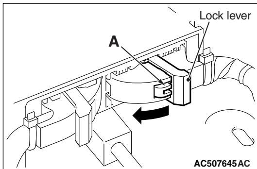
**STEP 4. Check the side-air bag module (LH) circuit.****Measure the resistance at the SRS-ECU connector C-27.**
