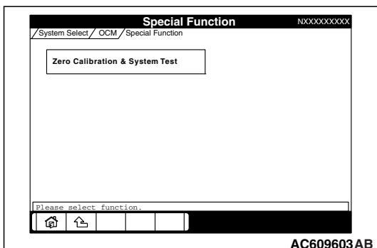
2. To execute accuracy check and calibration, operate scan tool MB991958 (M.U.T.-III Sub Assembly) as follows.
