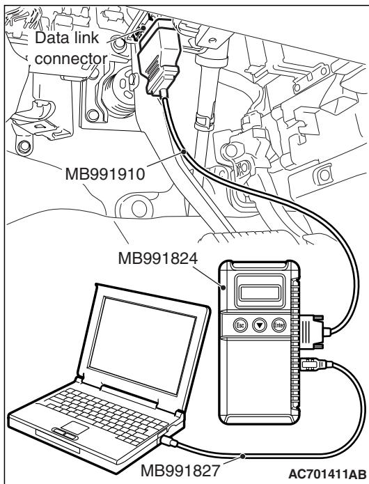
**DTC B1C33: Driver's Lap Pre-tensioner (Squib) System (Shorted to Squib Circuit Ground)**
