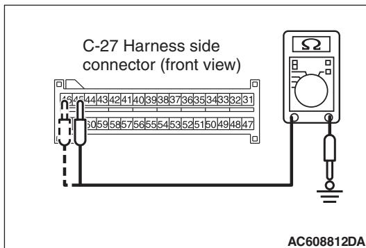
(5) Check for continuity between C-27 harness side connector terminals 45, 46 and body ground.
