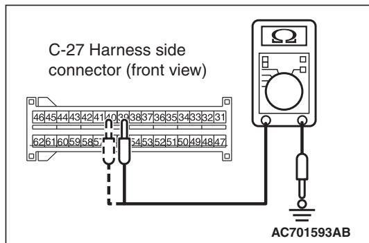
(5) Check for continuity between C-27 wiring harness side connector terminal No. 39, 40 and body ground.
