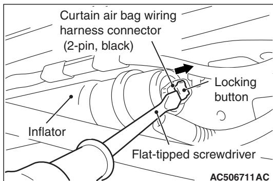
4. Use the flat-tipped screwdriver to pull out the locking button of curtain air bag harness side connector. After releasing the lock, disconnect the connector.
