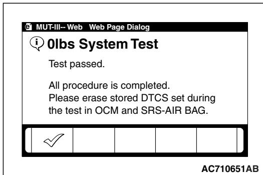
(12) The 0 lbs system test has been completed when the screen as shown in the illustration is displayed.
