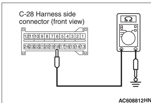
**STEP 5. Resistance measurement at the C-28 SRS-ECU connector.**
