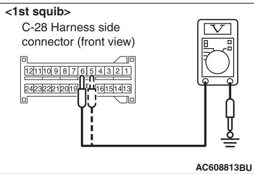
(7) Measure the voltage between C-28 harness side connector terminals 5 and 6 <1st squib> or 9 and 10 <2nd squib> and body ground.
