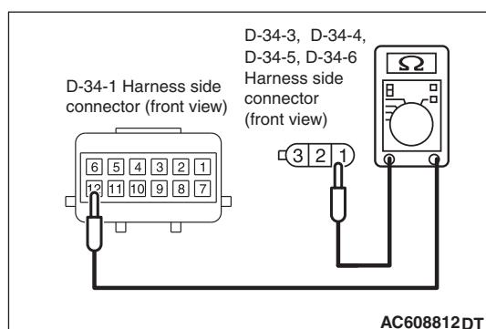
**STEP 4. Check the harness open circuit between occupant classification-ECU connector D-34-1 and weight sensor connector D-34-3, D-34-4, D-34-5 or D-34-6.**
