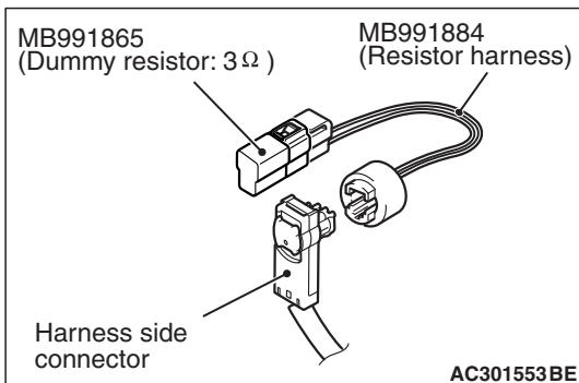
**STEP 4. Check the driver's seat belt pre-tensioner. (Using scan tool MB991958, read the diagnostic trouble code.)**
