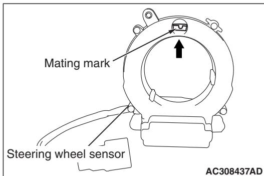
(3) Check that the white roller can be seen from the window for checking the neutral point when the mating marks are aligned.
