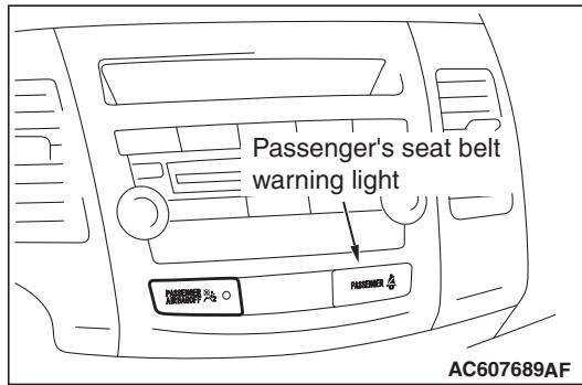
When an adult on the front passenger's seat wears the seat belt with the ignition switch "ON," confirm that the passenger's seat belt warning light goes out.
