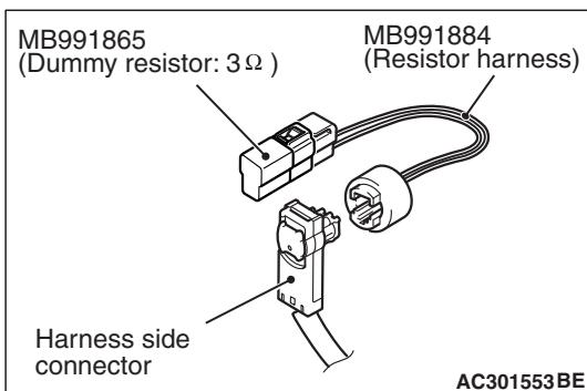
**STEP 3. Check the driver's seat belt pre-tensioner. (Using scan tool MB991958, read the diagnostic trouble code.)**
