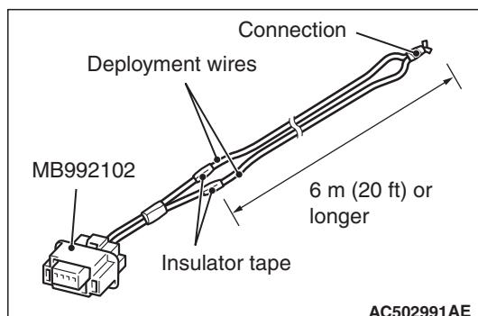
5. Connect deployment wires, each 6 meters (20 feet) or longer, to the two leads of special tool MB992102, and cover the connections with insulator tape. The other ends of the deployment wires should be connected to each other (short-circuited), to prevent sudden unexpected deployment of the air bag module.
