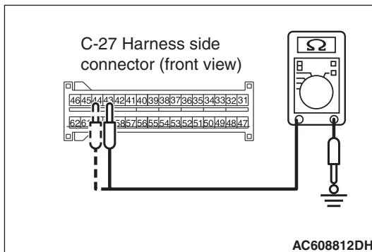
(5) Check for continuity between C-27 harness side connector terminals 43, 44 and body ground.
