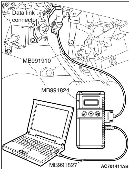
**STEP 3. Check SRS-ECU connector C-28, driver's air bag module connector C-205 and clock spring connector C-207. (Using scan tool MB991958, read the diagnostic trouble code.)**
