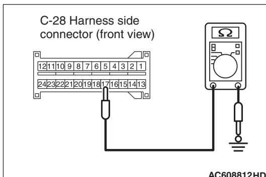
**STEP 6. Resistance measurement at the C-28 SRS-ECU connector.**
