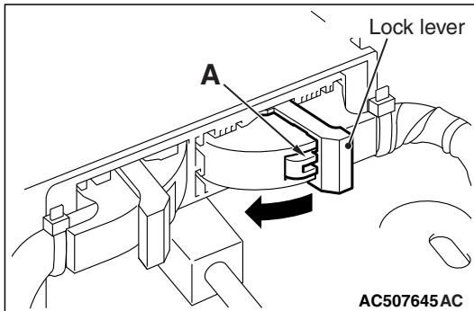
**STEP 4. Check the side-air bag module (RH) circuit.**
