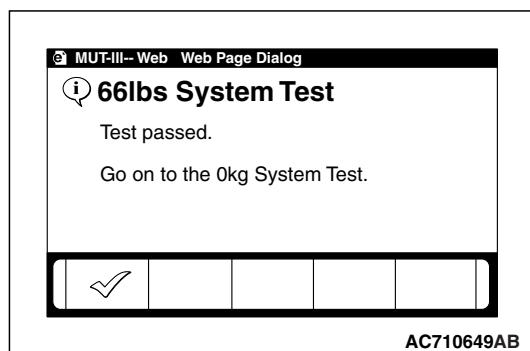
(9) The 66 lbs system test has been completed when the screen as shown in the illustration is displayed. The OK button is pushed and it progresses to the next.
