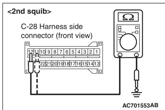
**STEP 5. Check the harness wires for short circuit to ground between the following connector.**
