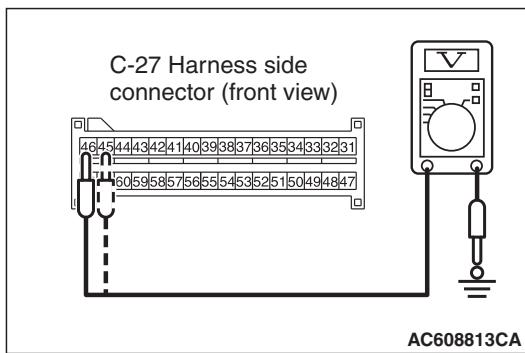
(7) Measure the voltage between C-27 harness side connector terminals 45, 46 and body ground.
