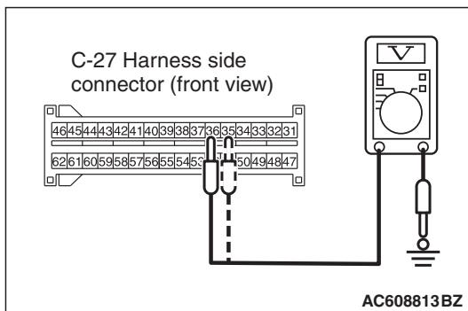
(7) Measure the voltage between C-27 harness side connector terminals 35, 36 and body ground.
