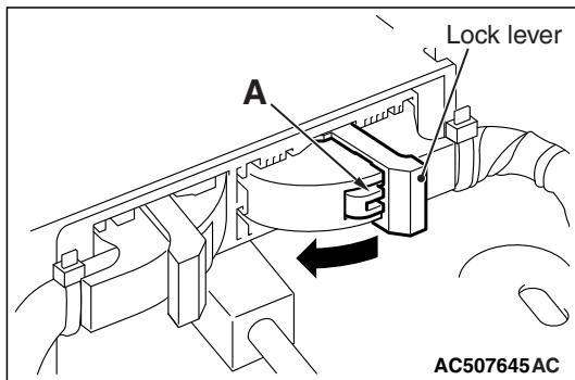
**STEP 5. Check the side-air bag module (LH) circuit.****Measure the resistance at the SRS-ECU connector C-27.**
