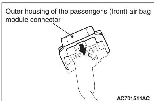
**STEP 3. Check SRS-ECU connector C-28 and passenger's (front) air bag module connector C-11. (Using scan tool MB991958, read the diagnostic trouble code.)**
