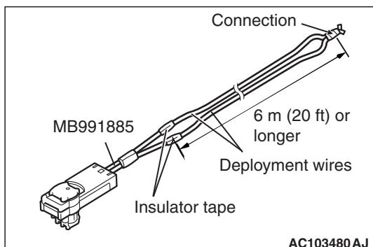
5. Connect deployment wires, each 6 meters (20 feet) or longer, to the two leads of special tool MB991885, and cover the connections with insulation tape. The other ends of the deployment wires should be connected to each other (short-circuited), to prevent sudden unexpected deployment of the curtain air bag module.
