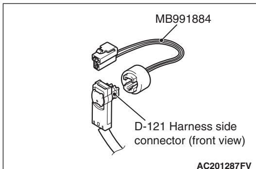
(5) Connect D-121 harness side connector to special tool MB991884.
