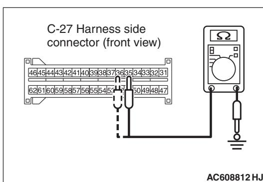
**STEP 4. Check the lap pre-tensioner circuit. Measure the resistance at the SRS-ECU connector C-27.**
