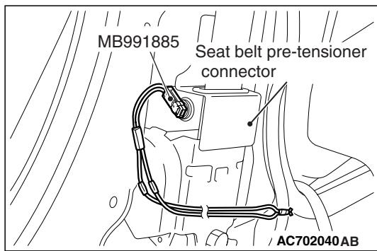
5. Connect deployment wires, each 6 meters (20 feet) or longer, to the two leads of special tool MB991885, and cover the connections with insulation tape. The other ends of the deployment wires should be connected to each other (short-circuited), to prevent sudden unexpected operation of the seat belt pre-tensioner.
