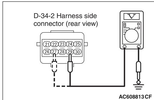
**STEP 4. Check the harness wires for short circuit to power supply between the occupant classification-ECU connector D-34-2 (terminal No.27 and 29) and seat slide sensor connector D-27 (terminal No.2 and 1).**
