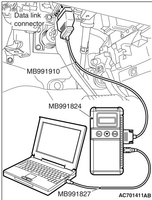
**STEP 1. Using scan tool MB991958, diagnose the CAN bus line****⚠ CAUTION**
