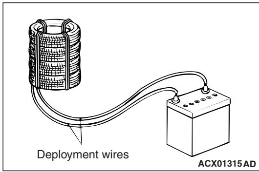
7. Place the tire to which the inflator is fixed onto the two stacked tires. Then, place 1 or more old tires without wheel onto the stacked tires, and tie and fix all the tires with rope. (4 positions)
