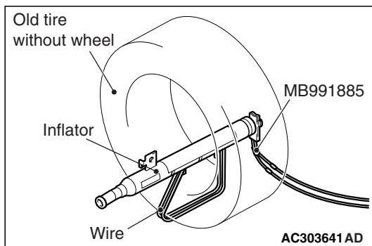
3. Cut the inflator from the air bag as shown in the figure using a cutter or a similar tool.
