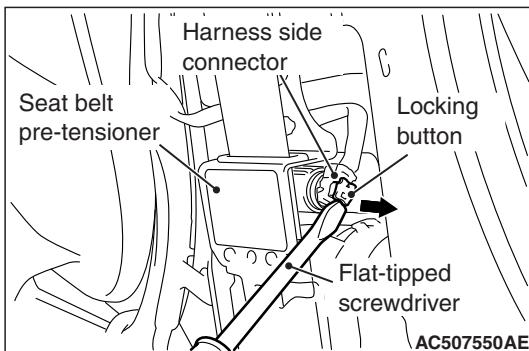
**STEP 3. Check SRS-ECU connector C-27 and driver's seat belt pre-tensioner connector D-121. (Using scan tool MB991958, read the diagnostic trouble code.)**
