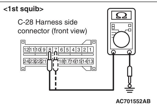
(5) Check for continuity between C-28 harness side connector terminals 7 and 8 <1st squib> or 11 and 12 <2nd squib>, and body ground.
