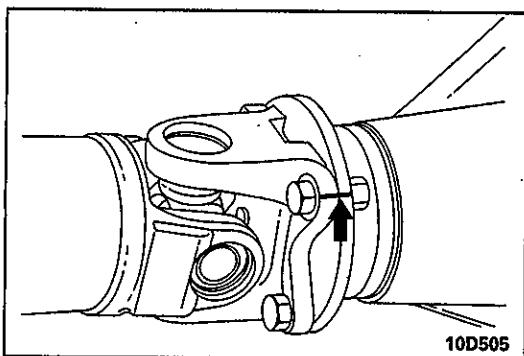
Install the propeller shaft to the companion flange so that the mating marks are aligned.
