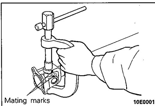
(4) Align the mating marks on the yoke and propeller shaft, and install the propeller shaft journal bearings in the method described in (2) and (3) above.
