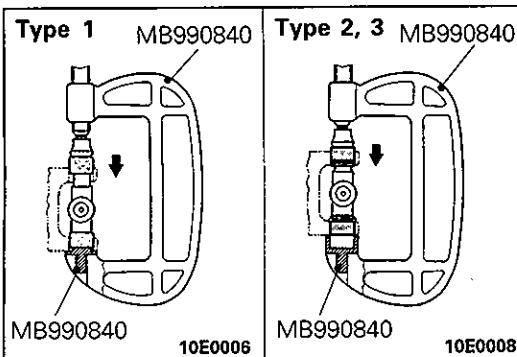
(3) Use the special tool to press the opposite side journal bearing into the yoke.
