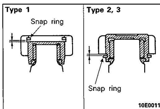
(3) Install the snap ring on the opposite side, and measure the clearance of the snap ring groove with a thickness gauge.
