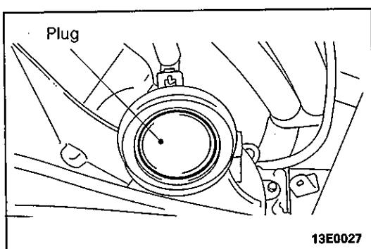
(2) Use the plug as a cover so that no foreign material gets into the transmission or transfer.
