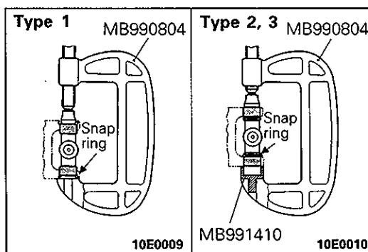
(2) Use the special tool at the opposite side of the installed snap ring to press in the journal bearing towards the snap ring.
