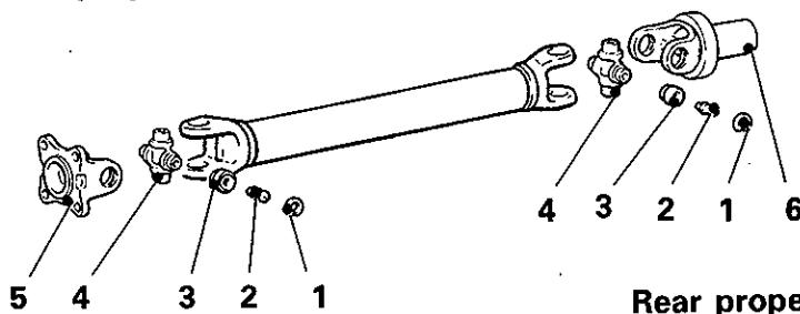
Rear propeller shaft (Type 1)
