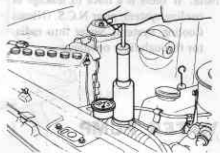
Fig. CO-7 Testing cooling system pressure
