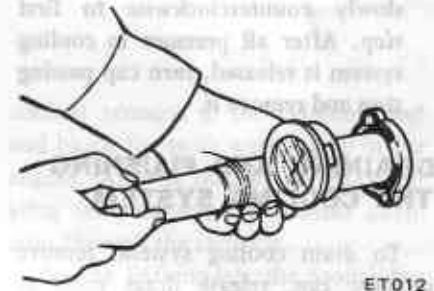
Fig. CO-6 Testing radiator cap
