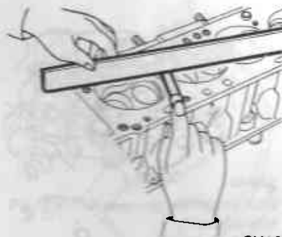
Fig. EM-20 Checking cylinder head surface
