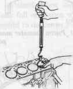
Fig. EM-43 Measuring piston fit in cylinder
