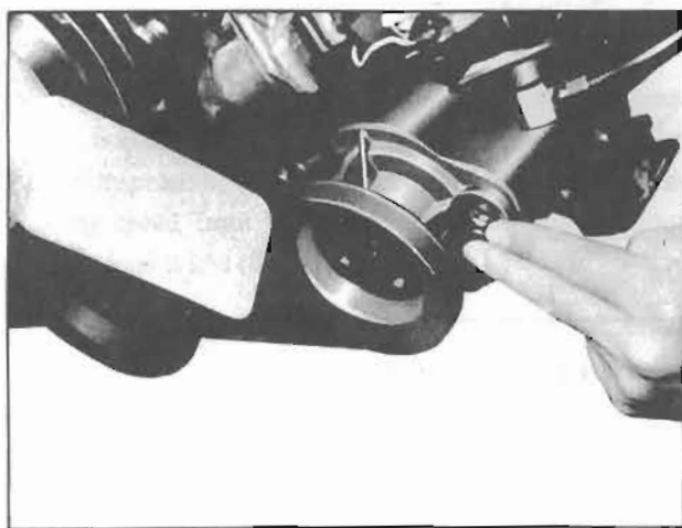
Fig. EC-21 Testing of relief valve
