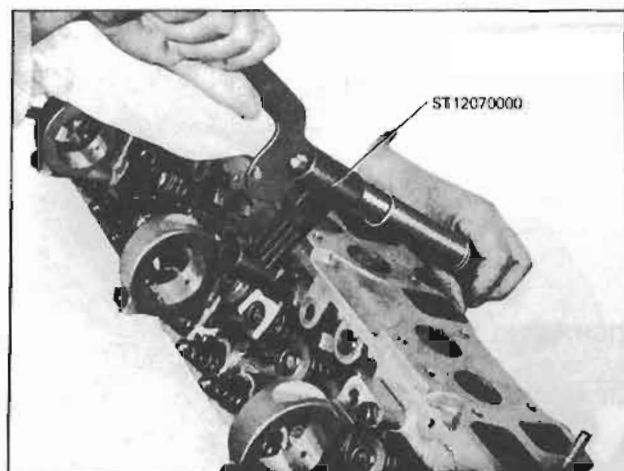
Fig. EM-69 Valve installation
