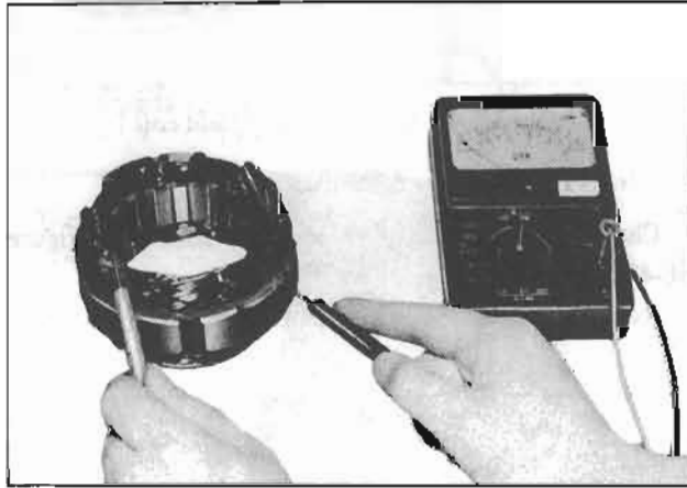
Fig. EE-51 Ground test
