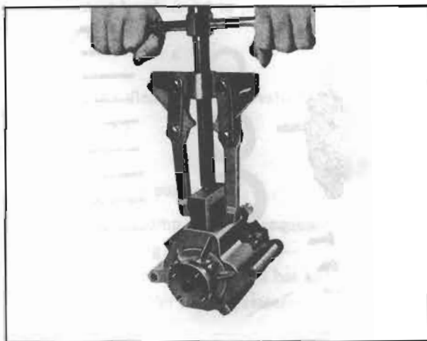
Fig. EC-13 Removing relief valve
