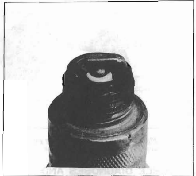
Fig. EE-99 Overheating (III)
