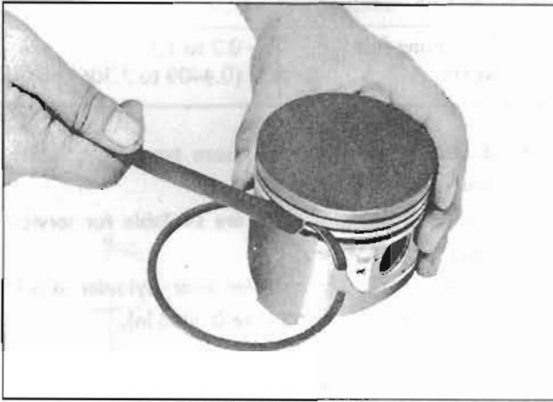
Fig. EM-53 Side clearance measurement
