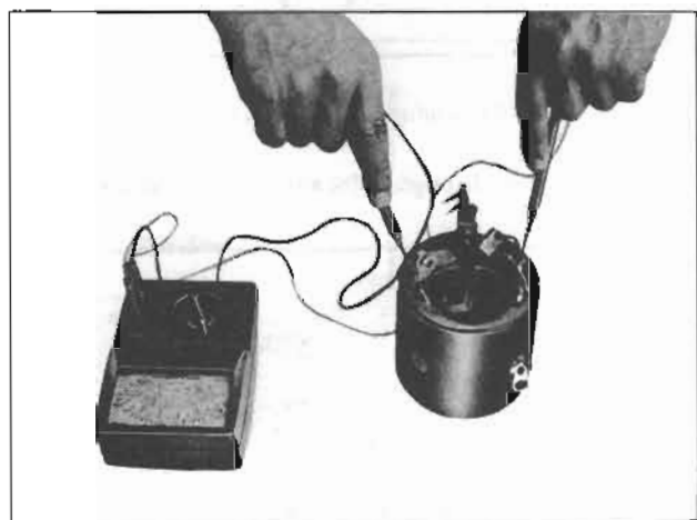
Fig. EE-12 Field coil test for continuity
