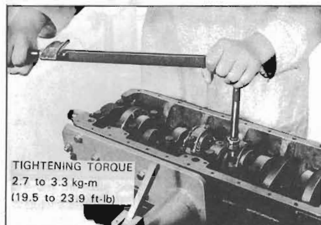
Fig. EM-80 Connecting rod cap installation
