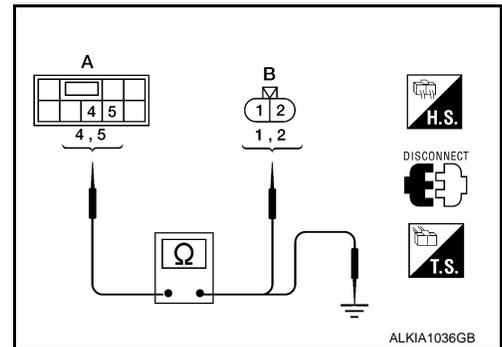
4. Check continuity between rear power window switch RH connector (A) and ground.
