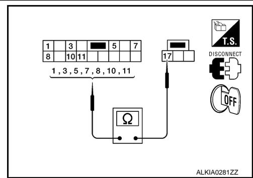
3. Check continuity between main power window and door lock/unlock switch (power window lock switch). (Unlock operation).
