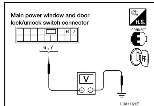
Is the measurement value within the specification?
