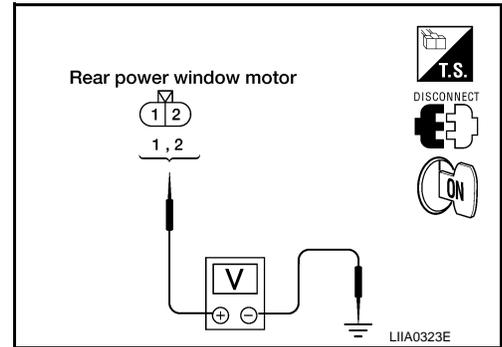
Is the measurement value within the specification?
