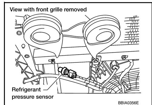
3. Check voltage between refrigerant pressure sensor terminal 1 and ground with CONSULT or tester.
