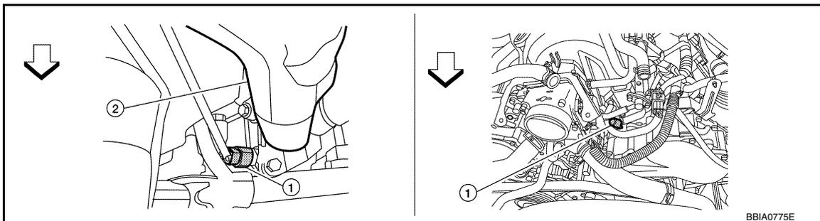
1. Engine coolant temperature (ETC) 2. Intake manifold sensor
