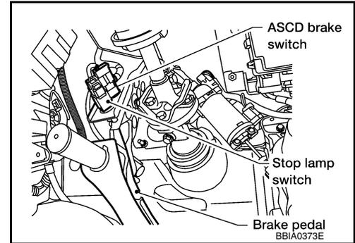
3. Check voltage between stop lamp switch terminal 1 and ground with CONSULT or tester.
