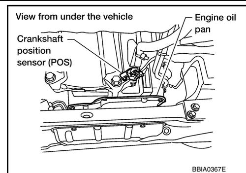
3. Check voltage between CKP sensor (POS) terminal 3 and ground with CONSULT or tester.
