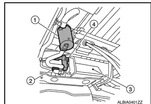
2. Check sensor harness connector for water.
