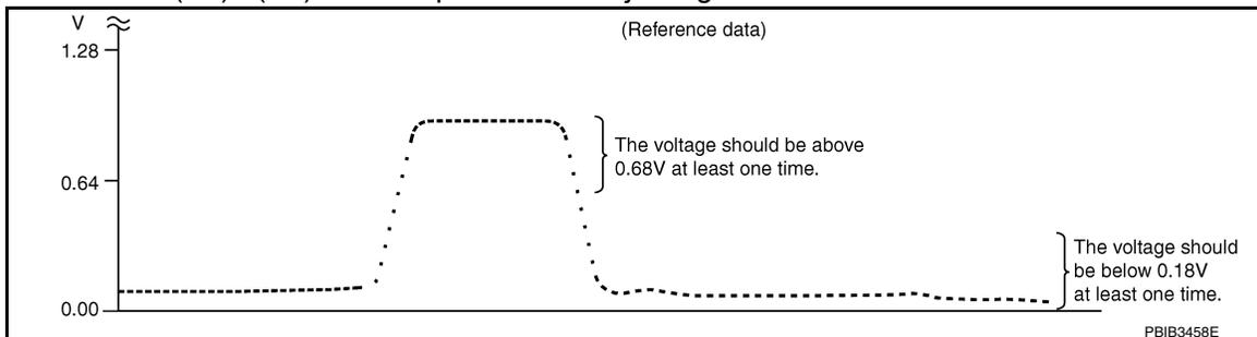
"HO2S2 (B1)/(B2)" should be above 0.70 V at least once when the "FUEL INJECTION" is +25%.
