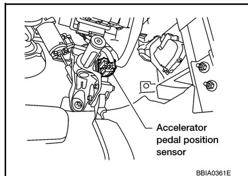
3. Check voltage between APP sensor terminal 7 and ground with CONSULT or tester.
