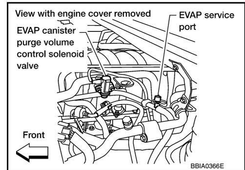
2. Also attach the pressure pump with pressure gauge to the EVAP service port adapter.
