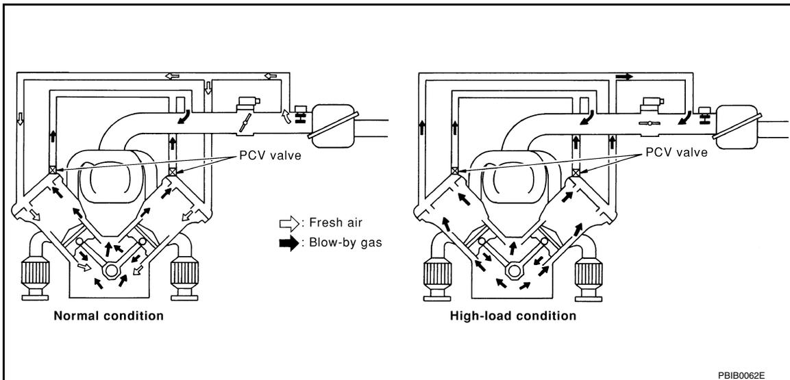
This system returns blow-by gas to the intake manifold.
