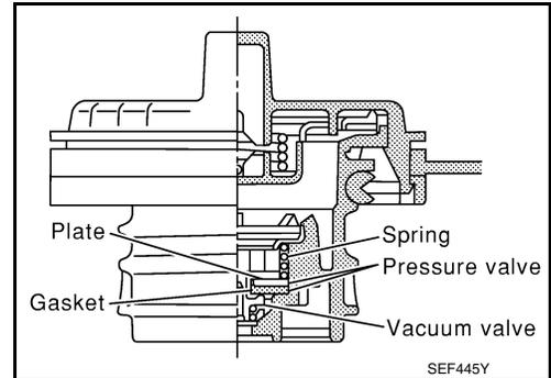
2. Check valve opening pressure and vacuum.
