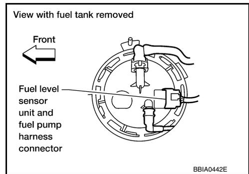
4. Check voltage between "fuel level sensor unit and fuel pump" terminal 4 and ground with CONSULT or tester.
