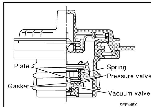
2. Check valve opening pressure and vacuum.
