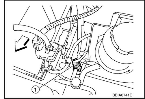
3. Check voltage between PSP sensor terminal 1 and ground with CONSULT or tester.
