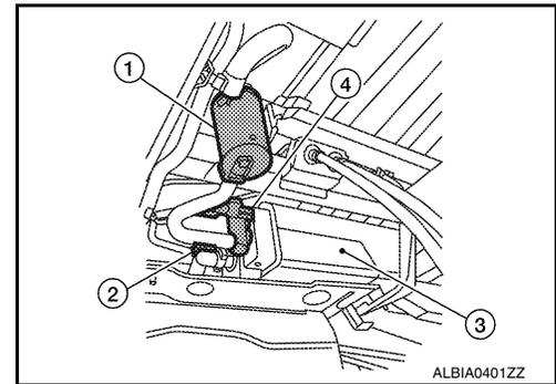
3. Pressurize the EVAP line using pressure pump with 1.3 to 2.7 kPa (10 to 20 mmHg, 0.39 to 0.79 inHg), then remove pump and EVAP service port adapter.
