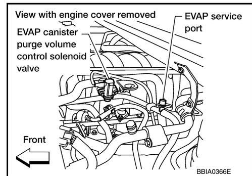
4. Check voltage between EVAP canister purge volume control solenoid valve terminal 1 and ground with CONSULT or tester.
