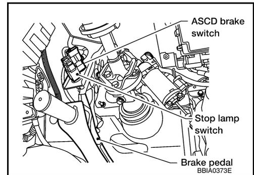
4. Check voltage between ASCD brake switch terminal 1 and ground with CONSULT or tester.
