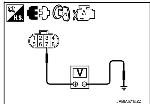
3. CHECK APP SENSOR 2 POWER SUPPLY CIRCUIT-I
