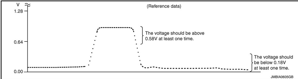
"HO2S2 (B1)/(B2)" should be above 0.58V at least once when the "FUEL INJECTION" is +25%.
