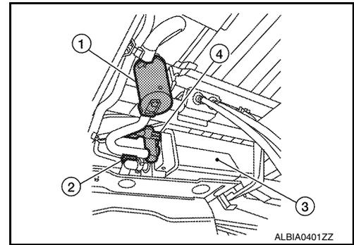
4. To locate the leak, deliver positive pressure to the EVAP system until pressure gauge points reach 1.38 to 2.76 kPa (0.014 to 0.028 kg/cm<sup>2</sup>, 0.2 to 0.4 psi).
