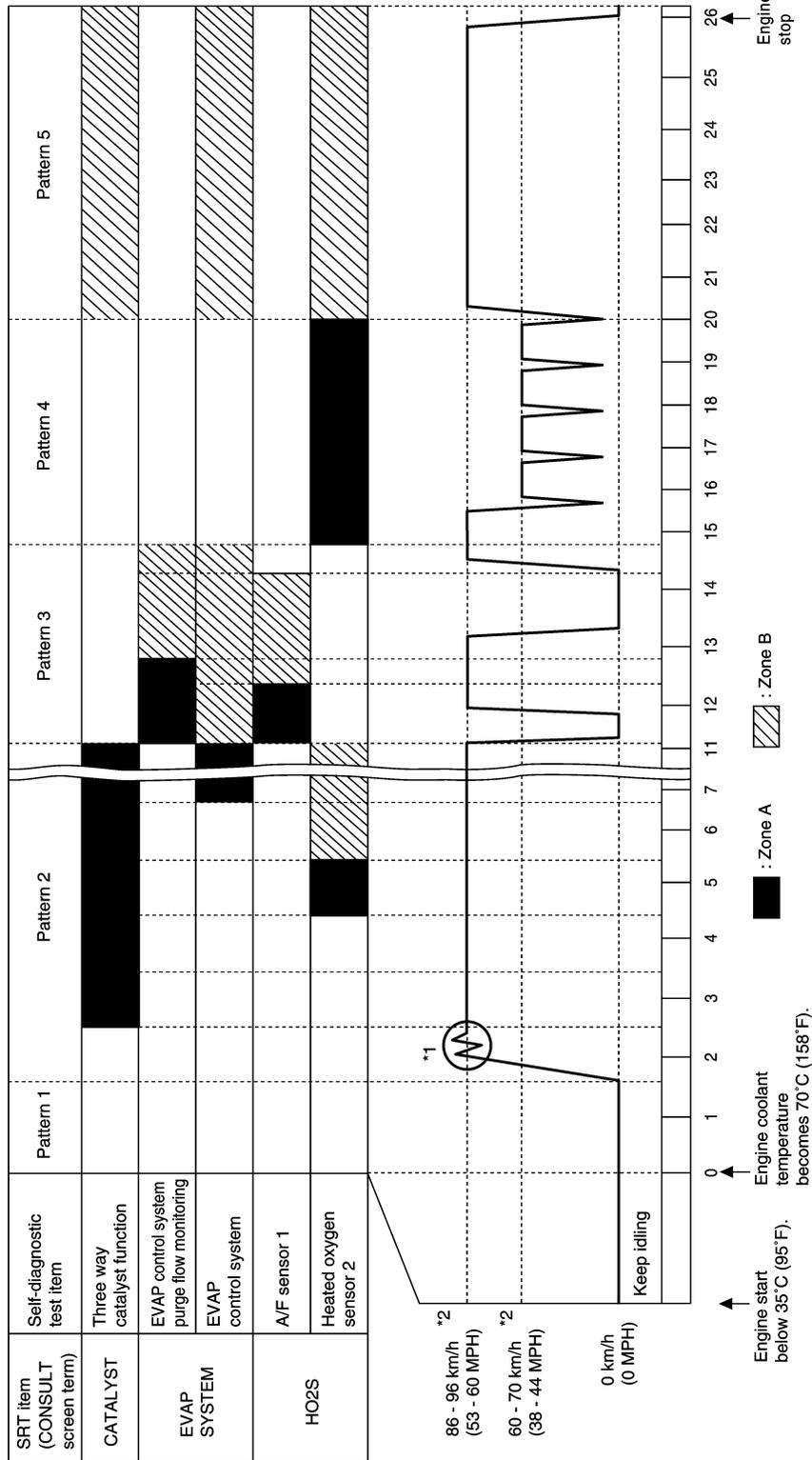
\*1: Depress the accelerator pedal until vehicle speed is 90 km/h (56 MPH), then release the accelerator pedal and keep it released for more than 10 seconds. Depress the accelerator pedal until vehicle speed is 90 km/h (56 MPH) again.
