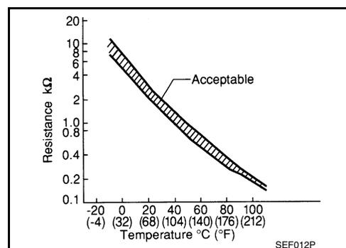
\*: This data is reference value and is measured between ECM terminal 73 (Engine coolant temperature sensor) and ground.
