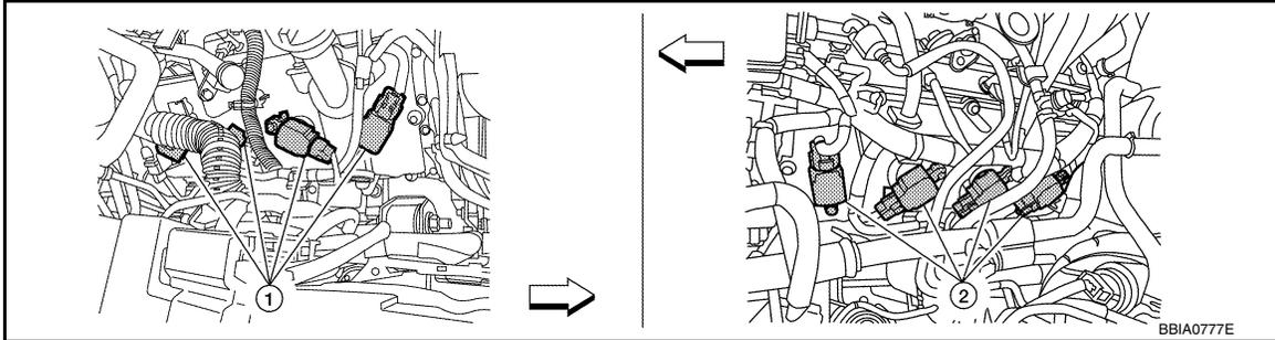
1. Ignition coils (with power transistor) (bank 2)
