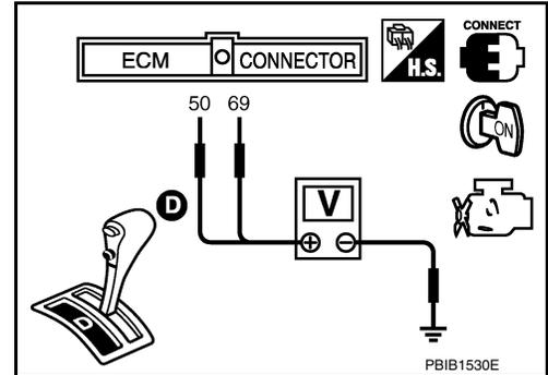
6. If NG, replace electric throttle control actuator and go to the next step.
