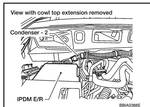
5. Check voltage between condenser-2 terminal 1 and ground with CONSULT or tester.
