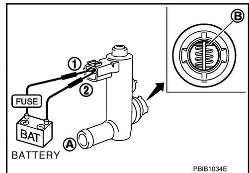
4. Clean the air passage (portion **A to B**) of EVAP canister vent control valve using an air blower.
