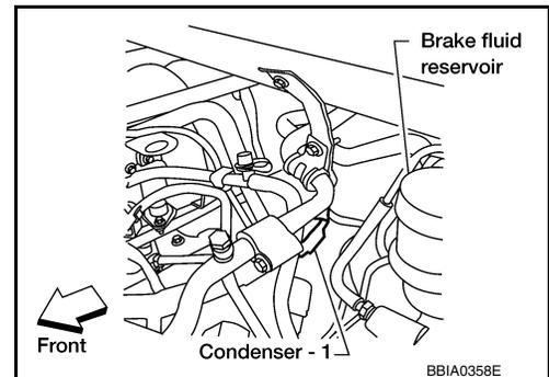
4. Check voltage between condenser-1 terminal 1 and ground with CONSULT or tester.
