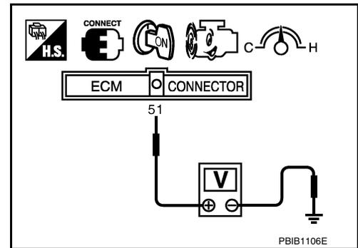
\*: Check for linear voltage rise in response to engine being increased to about 4,000 rpm.
