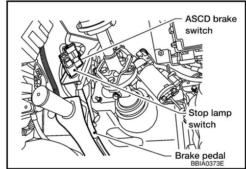
2. Check voltage between stop lamp switch terminal 1 and ground with CONSULT or tester.
