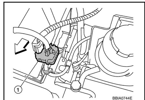
3. Check voltage between battery current sensor terminal 1 and ground with CONSULT or tester.
