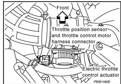
3. Check voltage between electric throttle control actuator terminal 2 and ground with CONSULT or tester.
