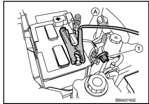
5. Check voltage between ECM terminal 71 (battery current sensor signal) and ground.
