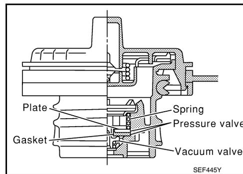
2. Check valve opening pressure and vacuum.
