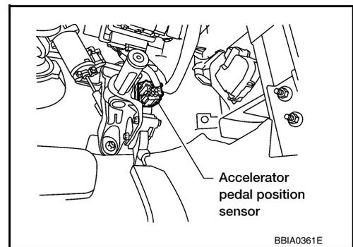
3. Check voltage between APP sensor terminal 6 and ground with CONSULT or tester.
