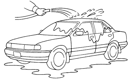
Water intrusion test
